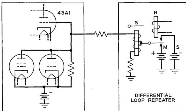
Fig. 17—Connection to other telegraph repeaters.
