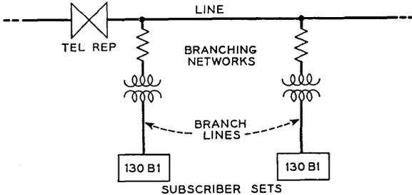
Fig. 14—Intermediate branch lines.
