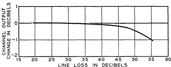
Fig. 17—Typical over-all channel net loss variation, nonrepeated.
