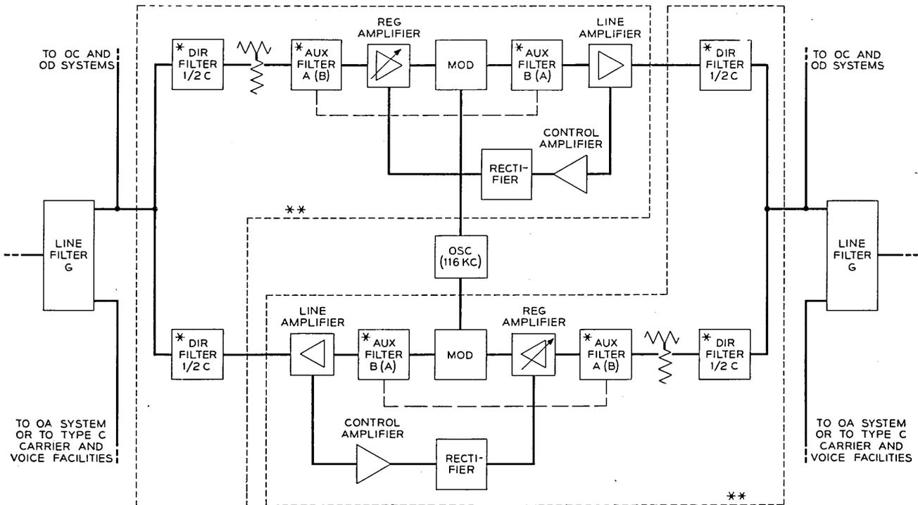
\* FILTERS ARE PLUG-IN AND REVERSIBLE    \*\* BASIC AMPLIFIER USED FOR OB, OC AND OD FOR REPEATERS AND GROUP RECEIVING UNITS
