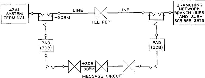
Fig. 15—Emergency circuit.
