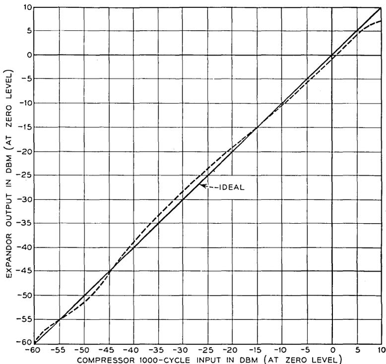
Fig. 16—Typical over-all channel load characteristic.
