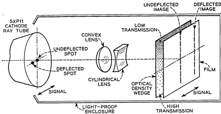
Fig. 8—Basic arrangement of probabloscope.
