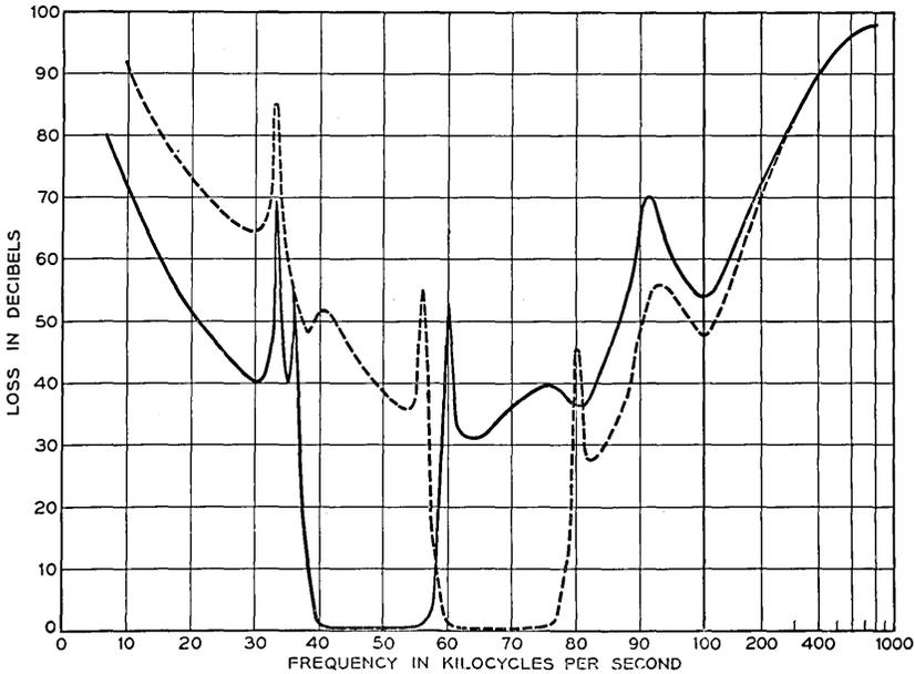
Fig. 23—Typical directional filter characteristics ( $C_B$ , 538A).
