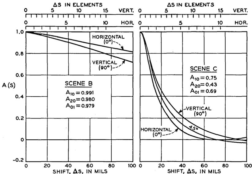
Fig. 7—Plots of autocorrelation for small shifts.  $A_{10}$  is the autocorrelation for a shift of one horizontal elemental distance,  $A_{20}$  for two horizontal elemental distances, and  $A_{01}$  for one vertical elemental distance. Alternatively  $A_{10}$  may be described as the average correlation between horizontally adjoining elements, etc.
