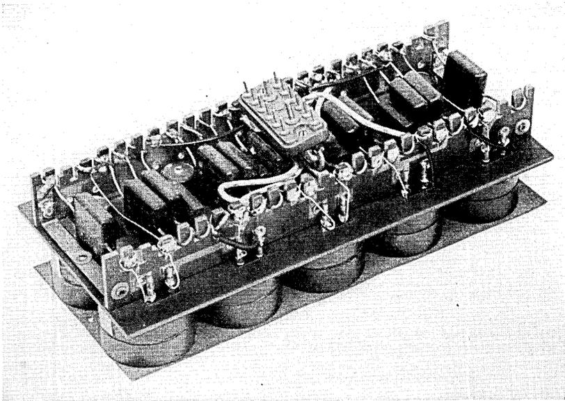
Fig. 32—Typical directional or auxiliary band filter—internal view.
