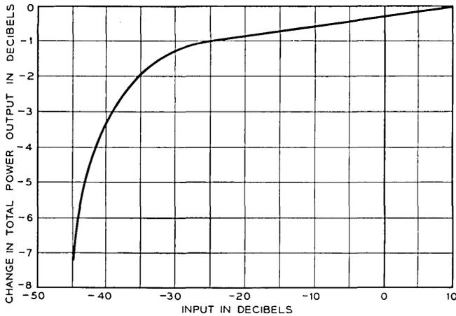
Fig. 18—Typical group receiving and repeater regulator characteristic.
