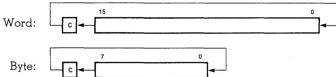
The contents of the destination operand with the C flag are rotated left one bit position if the source operand is 1, or two bit positions if the source operand is 2. The most significant bit (msb) of the destination operand replaces the C flag and the previous value of the C flag is moved to the bit 0 position of the destination during each rotation.
