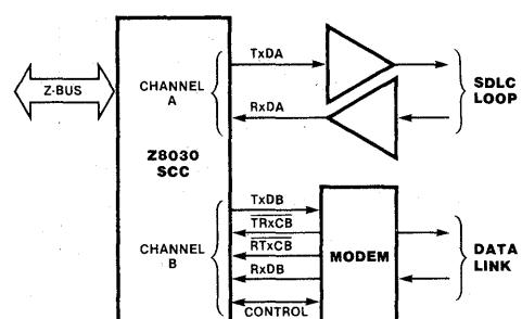
Figure 4. Loop Secondary Station and Serial Port
