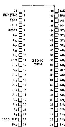
Figure 2. Pin Assignments
