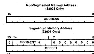
Figure 3-3. Segmented and Non-Segmented Address Formats
