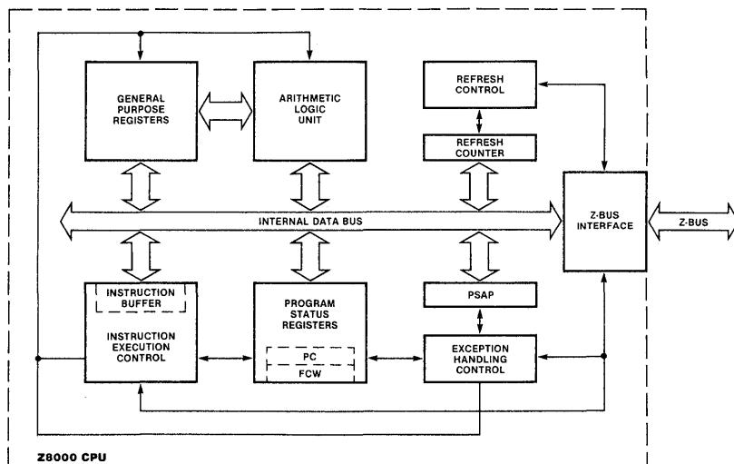
Figure 2-1. Z8000 CPU Functional Block Diagram
