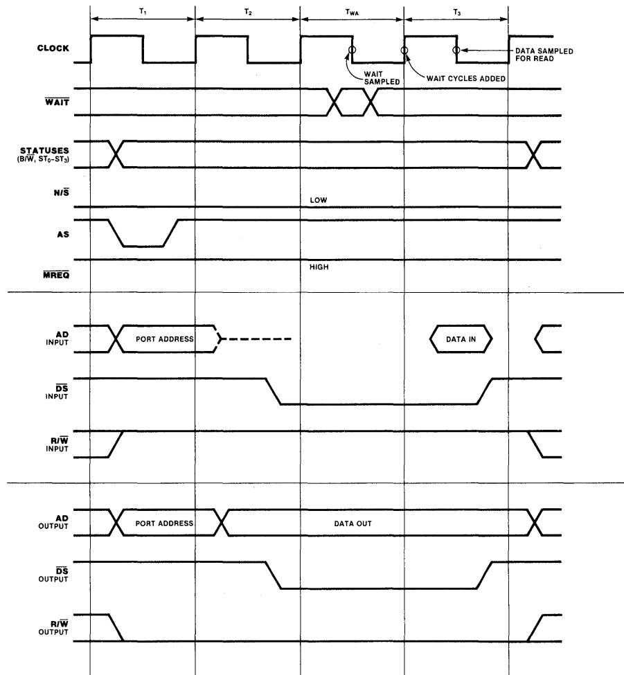
Figure 9-5. Input/Output Transaction
