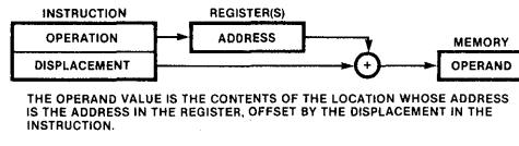
Any double-word register can be used for the base address *except RR0*. The Base Address mode allows access to locations whose segment numbers are not known at assembly time.
