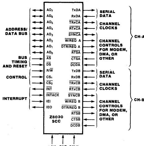
Figure 1. Pin Functions
