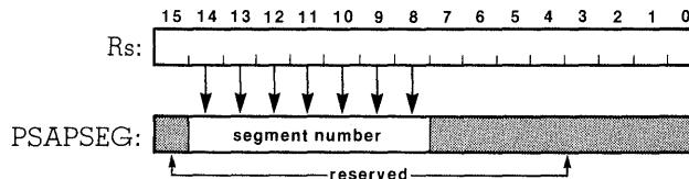
The PSAPSEG register may not be used in the nonsegmented Z8002. In the segmented Z8001, care must be exercised when changing the two PSAP register values so that an interrupt occurring between the changing of PSAPSEG and PSAPOFF is handled correctly. This is typically accomplished by first disabling interrupts before changing PSAPSEG and PSAPOFF.
