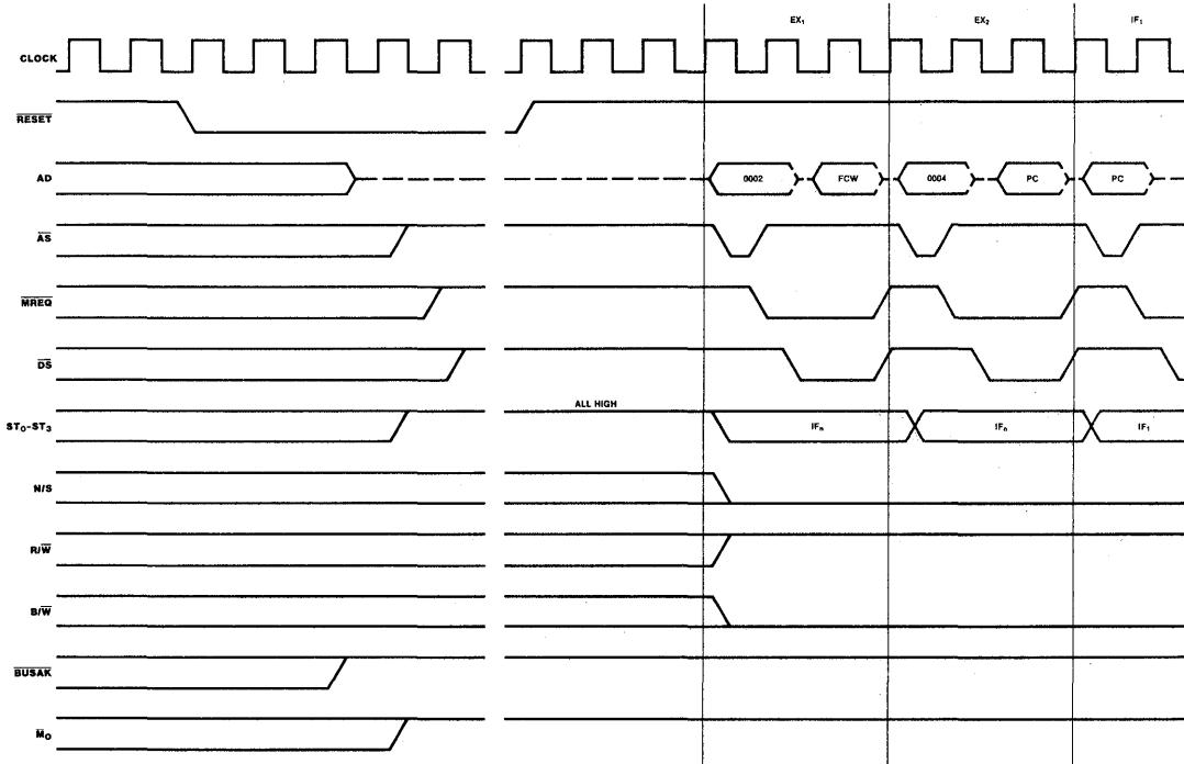
Figure 9-11. Reset Timing
