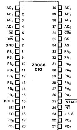
Figure 2. Pin Assignments
