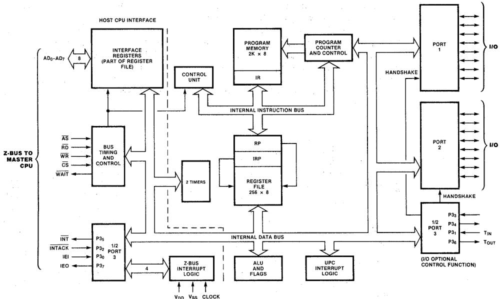
Figure 3. Z-UPC Functional Block Diagram
