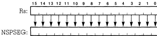
In segmented mode, the NSPSEG register is the normal mode R14 and contains the segment number of the normal mode processor stack pointer which is otherwise inaccessible for system mode.
