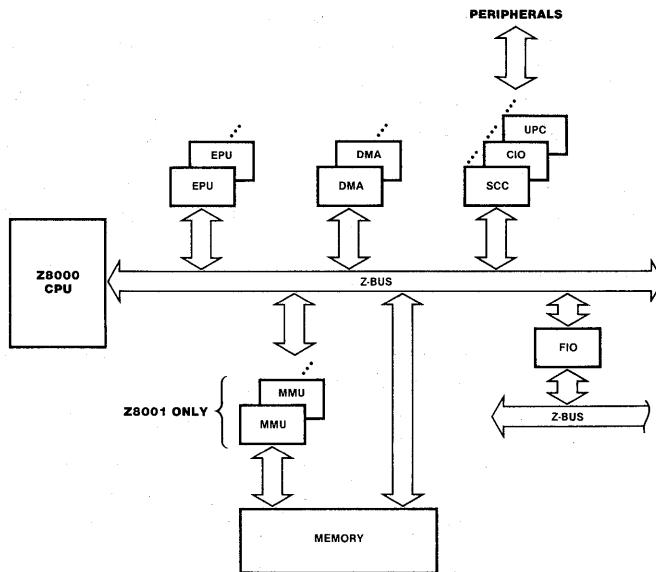
**Figure 2-2. Z8000 System Configuration**
