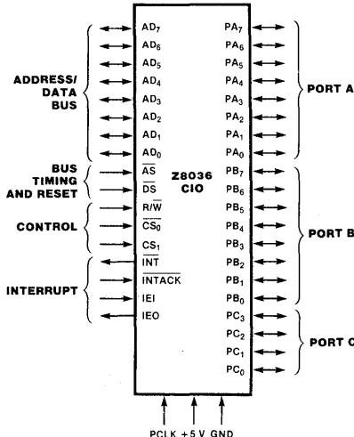
Figure 1. Pin Functions
