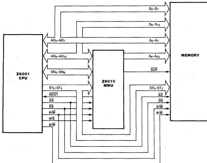
Figure 3. The MMU in a Z8000 System
