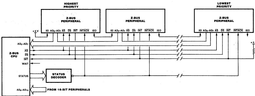
Figure 2. Interrupt Connections
