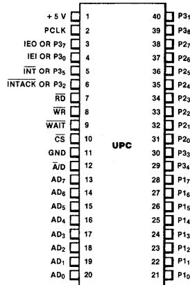
Figure 2. Pin Assignments
