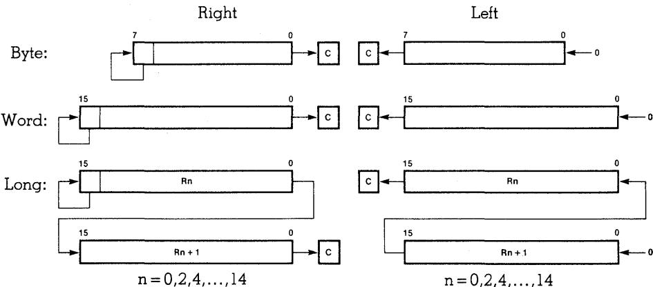
The destination operand is shifted arithmetically left or right by the number of bit positions specified by the contents of the source operand, a word register.
