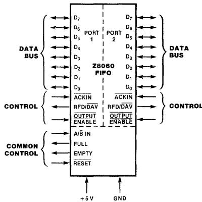
Figure 1. Pin Functions
