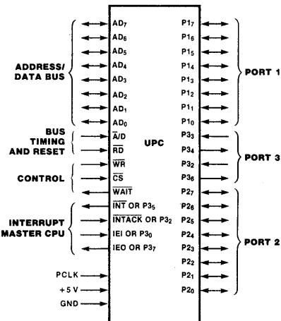
Figure 1. Pin Functions
