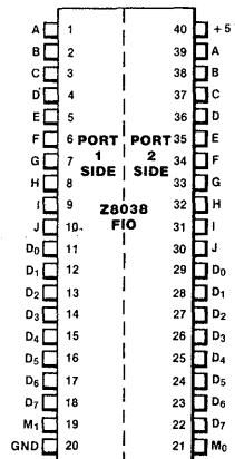
Figure 2. Pin Assignments
