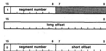
Figure 5.2. Segmented Memory Address Within Instruction.
