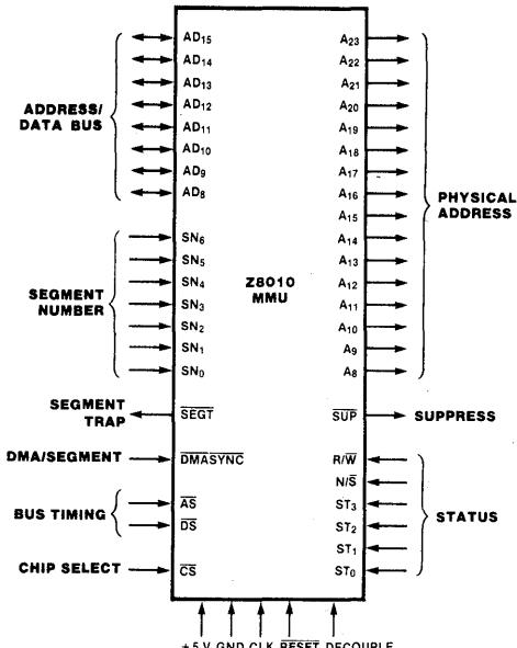
Figure 1. Pin Functions
