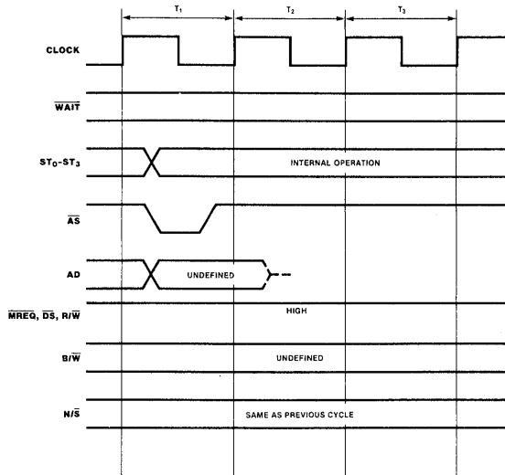
Figure 9-7. Internal Operation Timing
