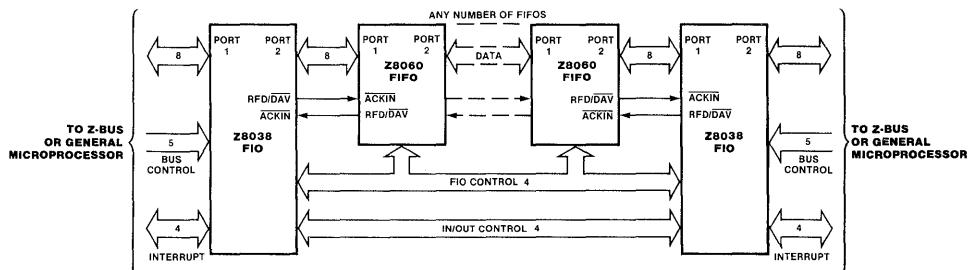
Figure 2. Using FIFOs to Extend FIOs
