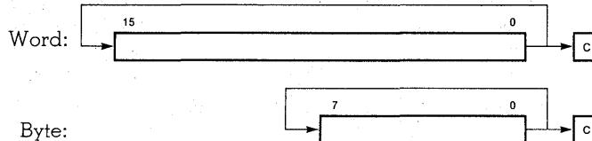
The contents of the destination operand are rotated right one bit position if the source operand is 1, or two bit positions if the source operand is 2. The least significant bit of the destination operand is moved to the most significant bit (msb) and also replaces the C flag.
