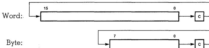
The contents of the destination operand with the C flag are rotated one bit position if the source operand is 1, or two bit positions if the source operand is 2. The least significant bit of the destination operand replaces the C flag and the previous value of the C flag is moved to the most significant bit (msb) position of the destination during each rotation.
