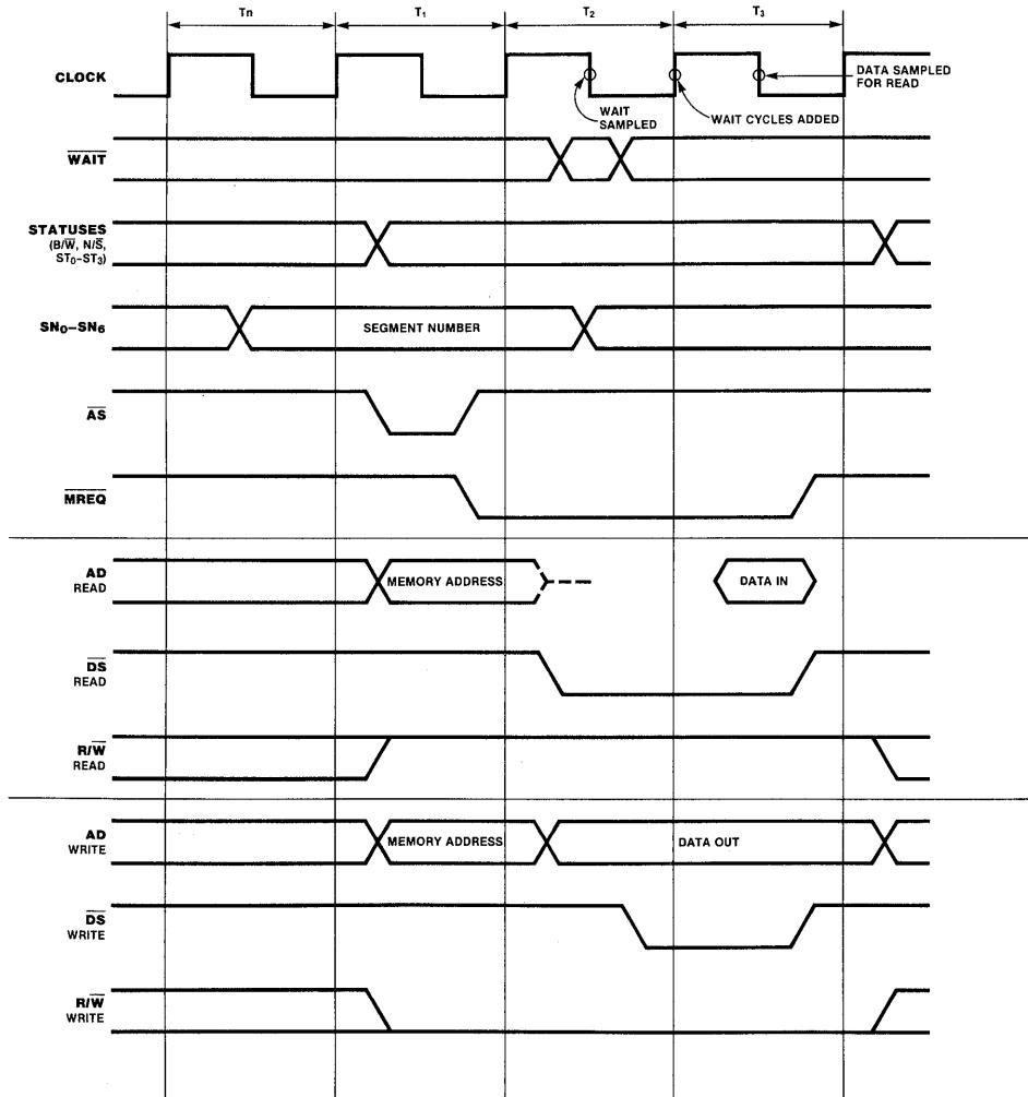
Figure 9-3. Memory Read and Write Transaction
