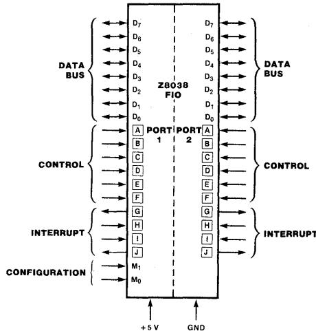
Figure 1. Pin Functions
