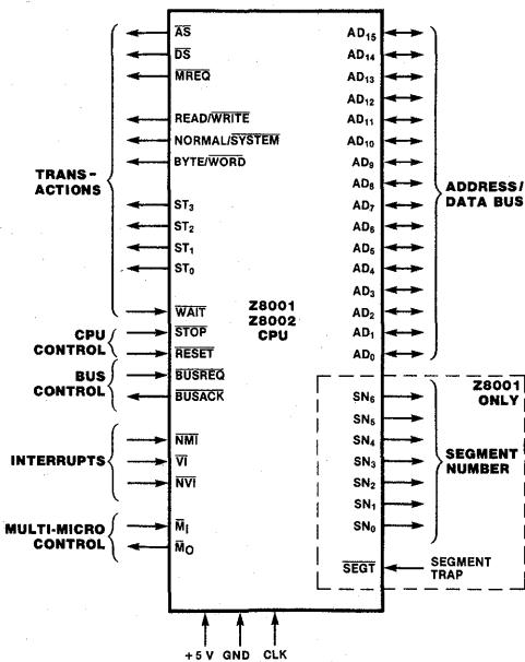
Figure 9-1. Pin Functions
