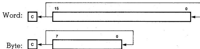
The contents of the destination operand are rotated left one bit position if the source operand is 1, or two bit positions if the source operand is 2. The most significant bit (msb) of the destination operand is moved to the bit 0 position and also replaces the C flag.
