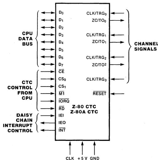
Figure 1. Pin Functions
