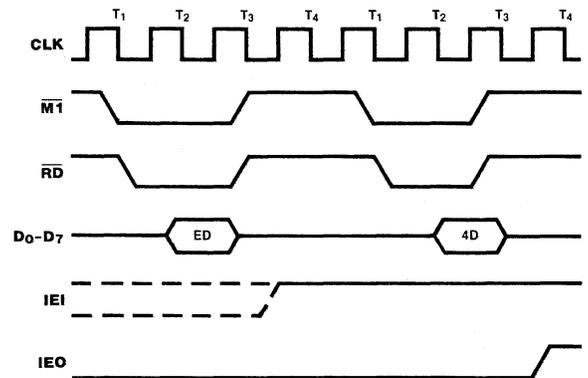
Figure 15. Return From Interrupt Timing
