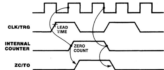
Figure 12. Counter Mode Timing
