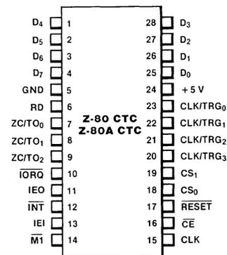
Figure 2. Pin Assignments
