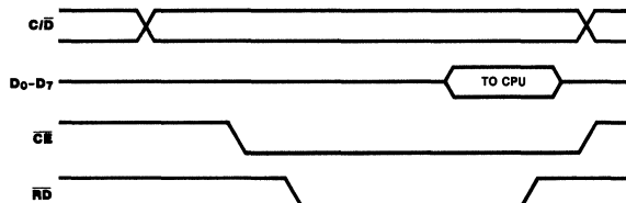
Figure 9. Non-Z-BUS Read Cycle Timing
