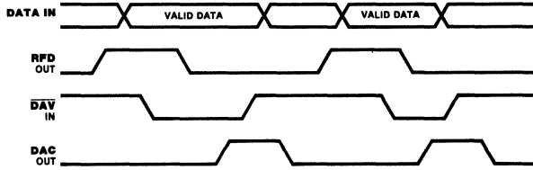
Figure 23. Input (Acceptor) Timing IEEE-488 HS Port: Port 2 Side Only
