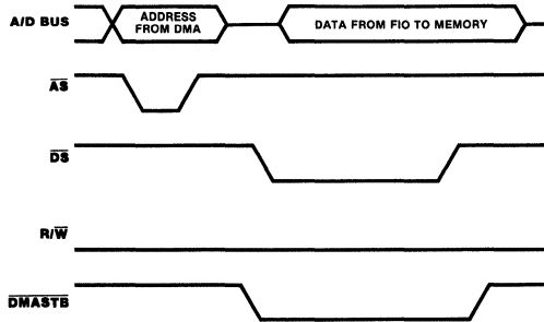
Figure 13. Z-BUS FIO to Memory Data Transaction
