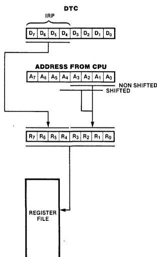
Figure 7. DSC Register Addressing Scheme
