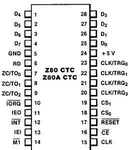
Figure 2. Pin Assignments
