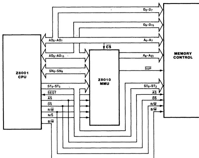
Figure 13. The MMU in a Z8001 System
