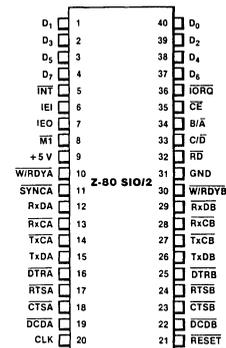
Figure 2. Z-80 SIO/2 Pin Assignments
