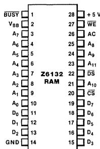
Figure 2. Pin Assignments
