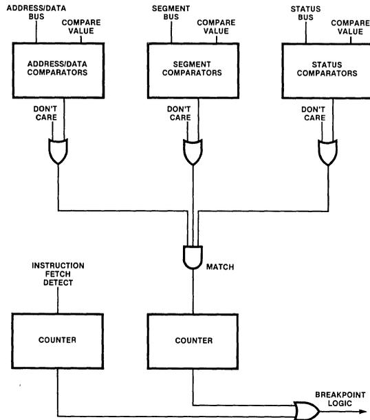
Figure 1. Hardware Trigger Implementation
