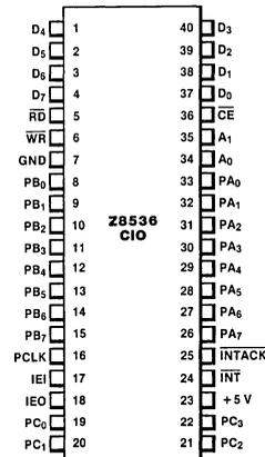
Figure 2. Pin Assignments
