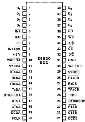
Figure 2. Pin Assignments
