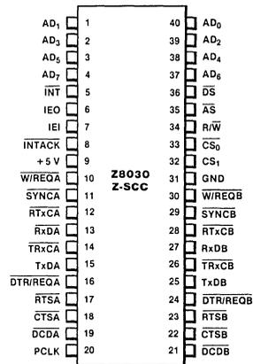
Figure 2. Pin Assignments
