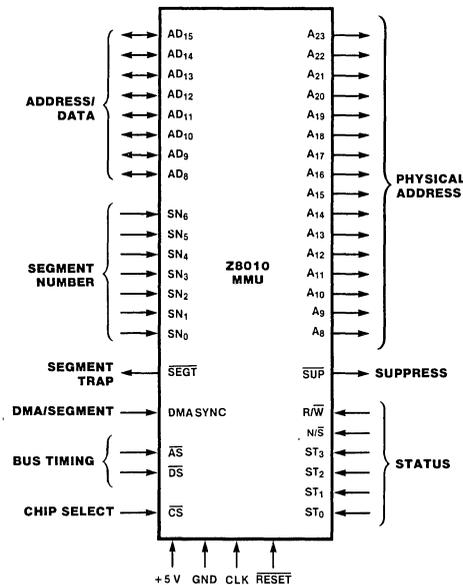
Figure 1. Pin Functions
