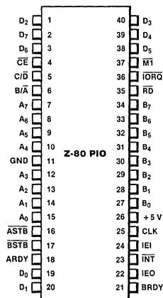
Figure 2. Pin Assignments
