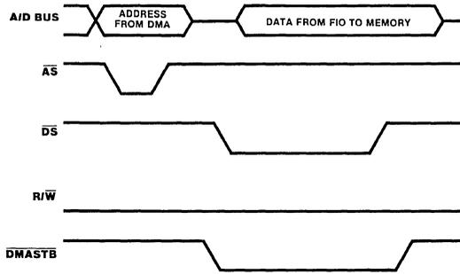
Figure 13. Z-BUS FIO to Memory Data Transaction
