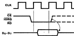
Figure 11. CPU-to-DMA Read Cycle
