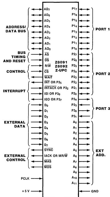
Figure 9. Z8091/Z8092 Z-UPC Pin Functions
