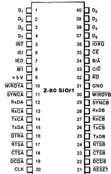
Figure 4. Z-80 SIO/1 Pin Assignments
