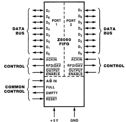
Figure 1. Pin Functions
