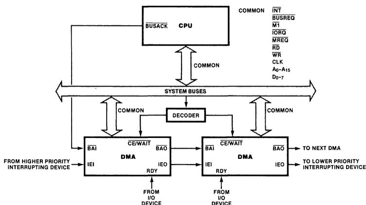
Figure 7. Multiple-DMA Interconnection to the Z-80 CPU
