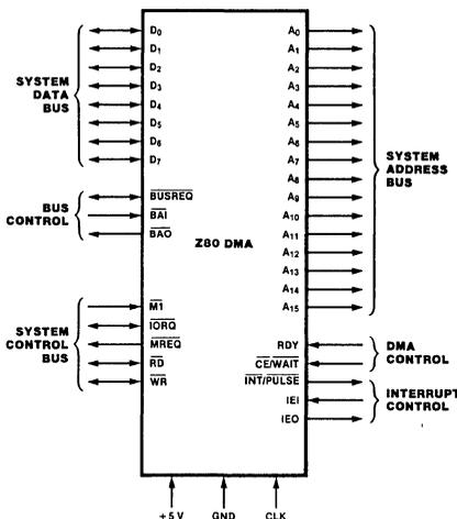
Figure 1. Pin Functions
