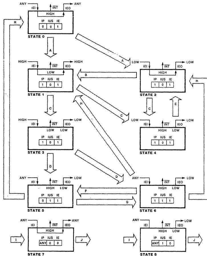
**Figure 5. State Diagram for an Interrupt Source**
