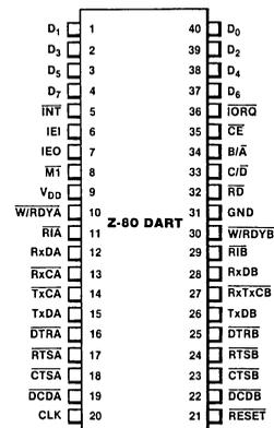
Figure 2. Pin Assignments
