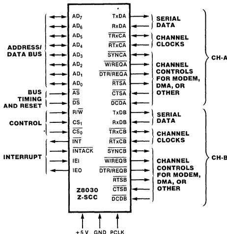
Figure 1. Pin Functions
