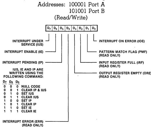
Figure 12. Port Specification Registers
