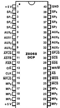
Figure 2. Pin Assignments
