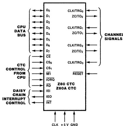
Figure 1. Pin Functions
