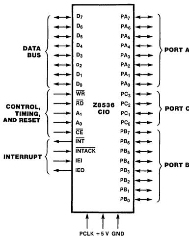
Figure 1. Pin Functions
