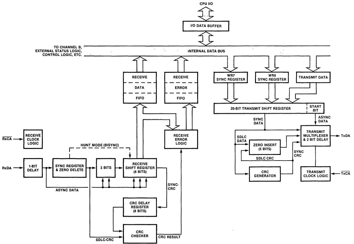
Figure 12. Transmit and Receive Data Path (Channel A)
