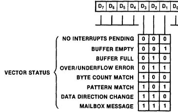
Figure 29. Interrupt Vector Register
