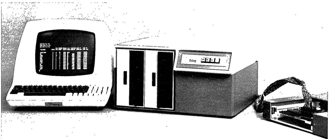
**ZDOS II File Manager.** The file manager organizes, stores and retrieves data from the floppy disk units. A directory provides a data index which is accessed using a "hierarchical linked list." All space on the disk is dynamically allocated on an as needed basis to prevent gaps in the storage space. Logical record lengths from 128 to 4096 bytes per record may be used. Also, all files may be assigned one or more attributes for protection and privacy.
