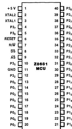
Figure 2. Pin Assignments
