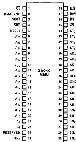
Figure 2. Pin Assignments
