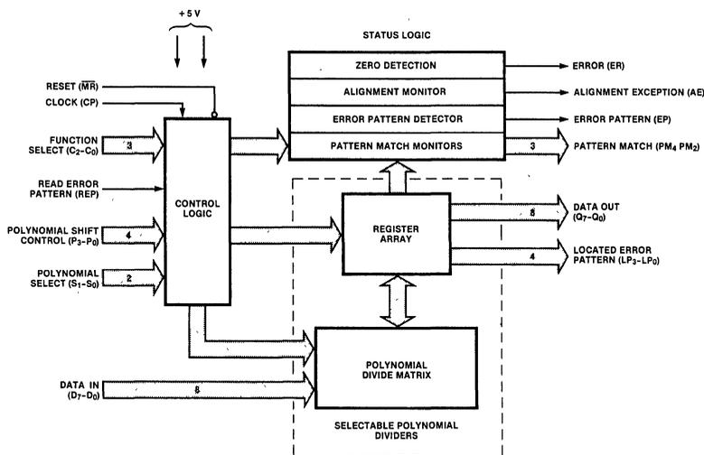
Figure 3. Block Diagram
