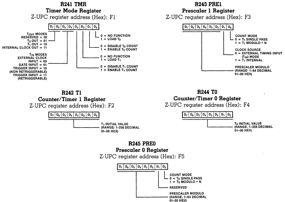
Figure 17. Z-UPC Counter/Timer Registers
