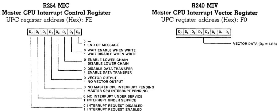
Figure 14. Master CPU Interrupt Registers
