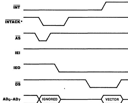
\* $\overline{INTACK}$  is decoded from Z8000 status.
