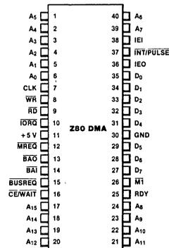
Figure 2. Pin Assignments
