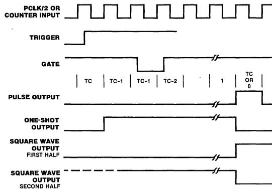
**Figure 10. Counter/Timer Waveforms**
