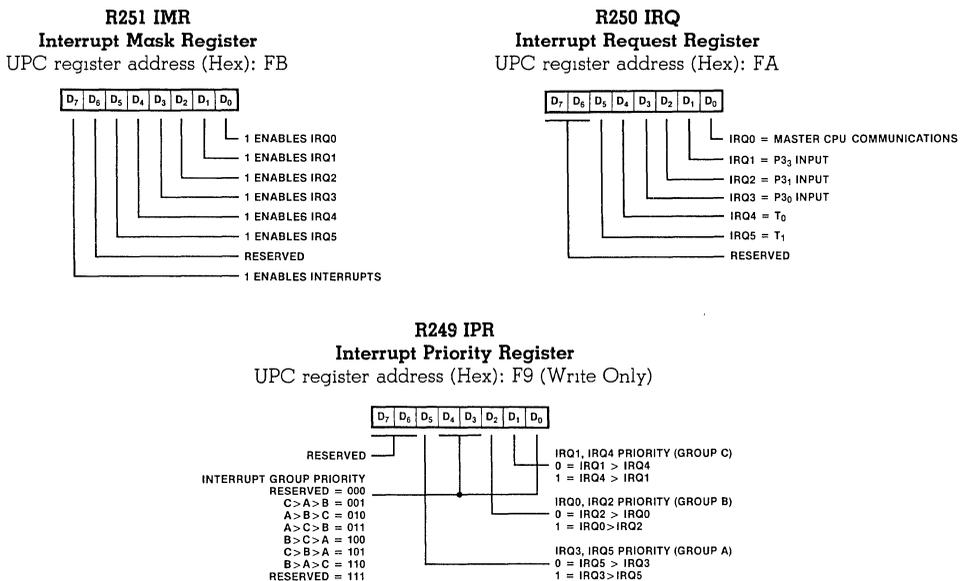
Figure 13. Interrupt Control Registers
