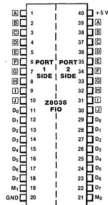
Figure 2. Pin Assignments
