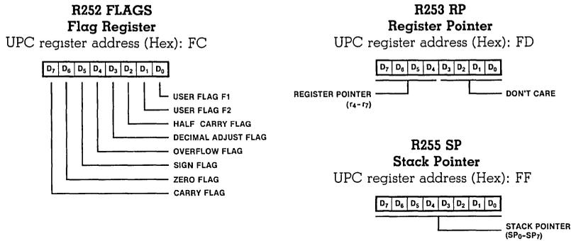
Figure 15. UPC Control Registers
