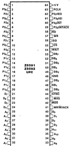
Figure 10. Z8591/Z8592 UPC Pin Assignments
