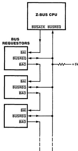
Figure 6. Bus Request Connections
