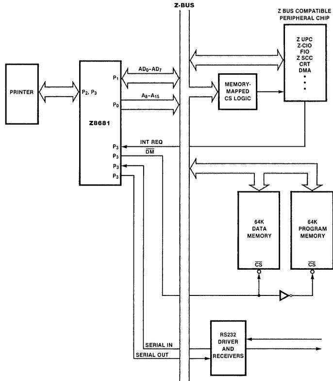
Figure 4. Z8681 Interfacing to External Memory
