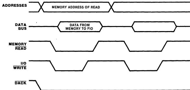
Figure 16. Non-Z-BUS Memory to FIO Data Transaction
