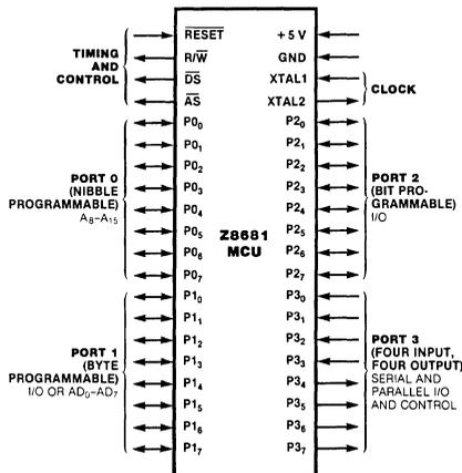
Figure 1. Pin Functions
