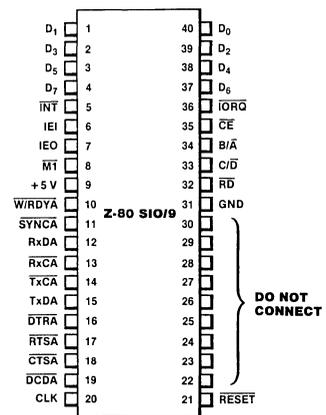
Figure 2. Z-80 SIO/9 Pin Assignments
