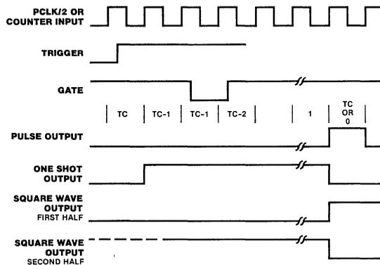
**Figure 10. Counter/Timer Waveforms**
