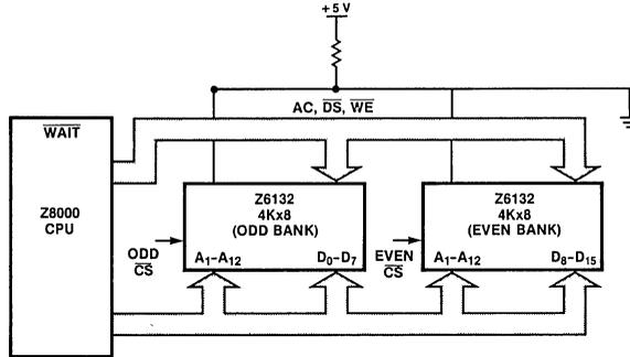
Figure 5. Block Diagram
