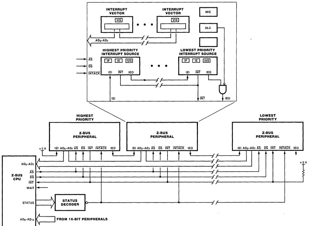
Figure 4. Interrupt Connections
