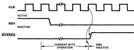
Figure 18. Bus Release When Not Ready (Burst Mode)
