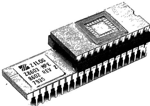
Figure 12. The Z8603 Microcomputer Protopack Emulator
