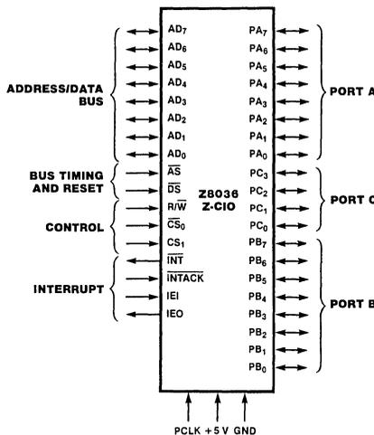
Figure 1. Pin Functions
