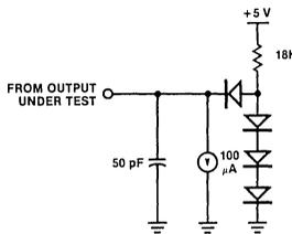
Figure 16. Test Load 2
