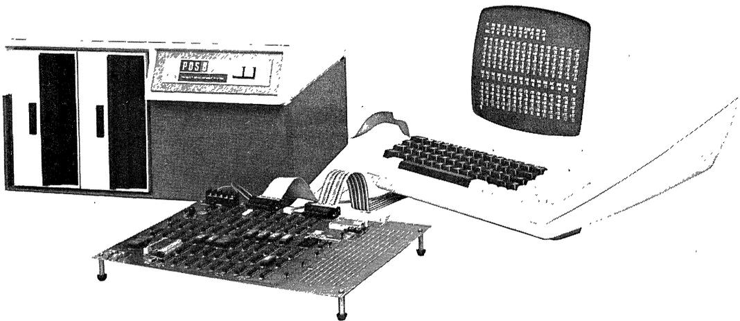
**Z8 Development Module conveniently connects to both the CRT and PDS 8000 Development System.**
