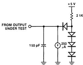
Figure 15. Test Load 1
