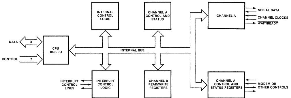
Figure 3. Block Diagram
