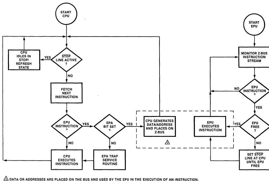
Figure 8. EPA and Z8000 CPU Instruction Execution
