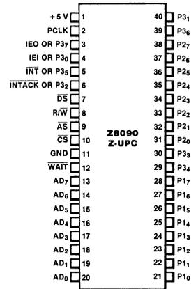
Figure 2. Z8090 Z-UPC Pin Assignments
