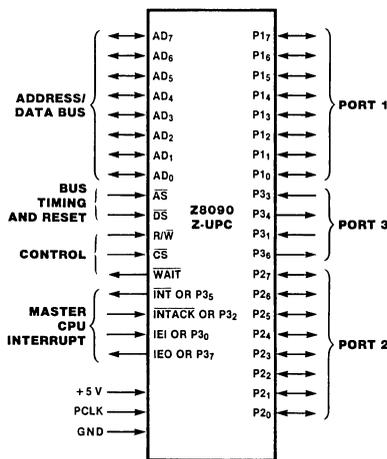
Figure 1. Z8090 Z-UPC Pin Functions
