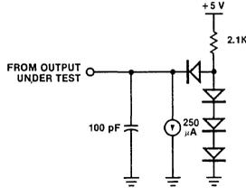
Figure 15. Standard Test Load
