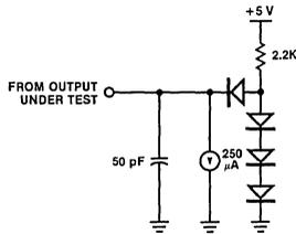
Figure 18. Test Load 1
