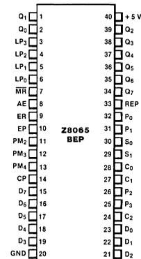
Figure 2. Pin Assignments
