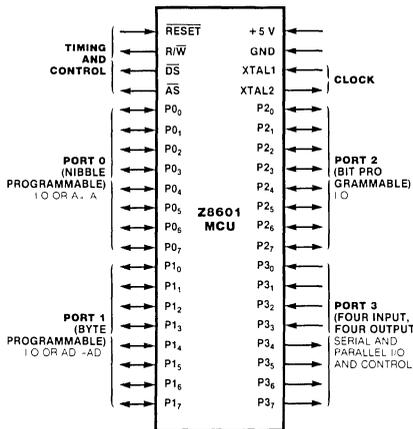
Figure 1. Z8601 MCU Pin Functions
