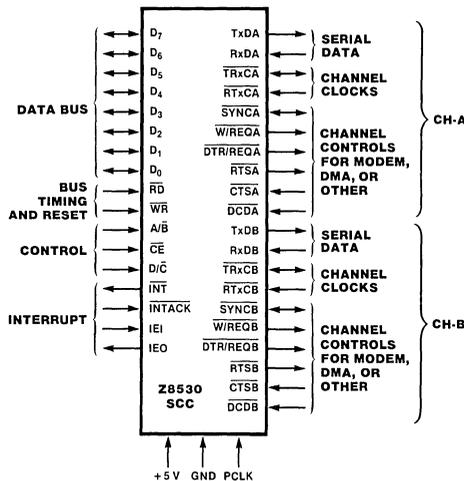
Figure 1. Pin Functions
