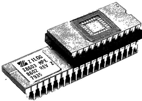
Figure 12. The Z8613 Microcomputer Protopack Emulator
