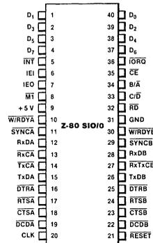
Figure 6. Z-80 SIO/0 Pin Assignments
