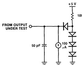
Figure 16. Test Load 2
