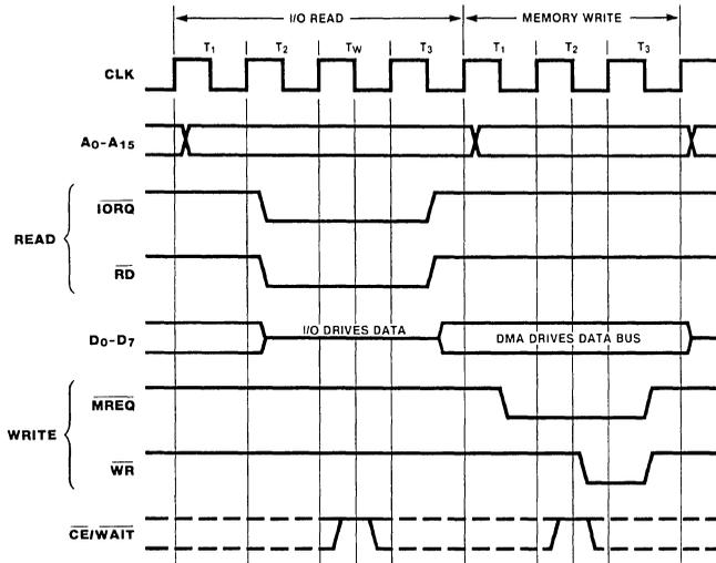
Figure 13. I/O-to-Memory Transfer
