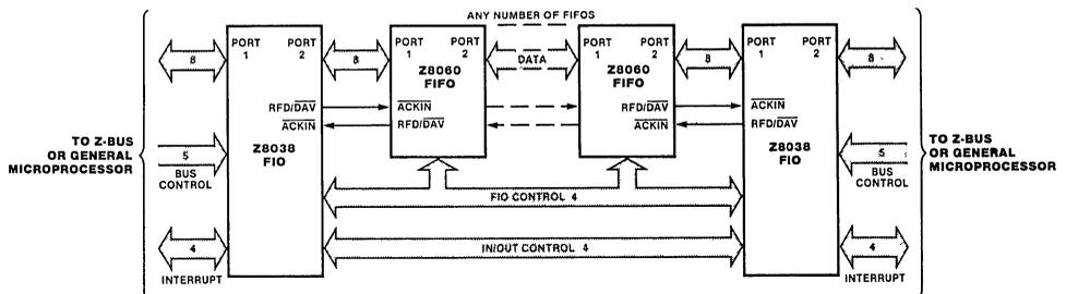
Figure 2. Using FIFOs to Extend FIOs
