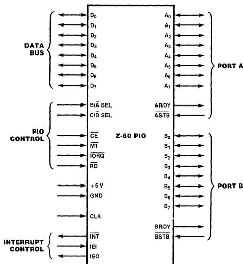
Figure 1. Pin Functions
