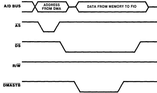
Figure 14. Z-BUS Memory to FIO Data Transaction
