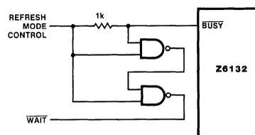
Figure 4. External  $\overline{\text{WAIT}}$  Generation
