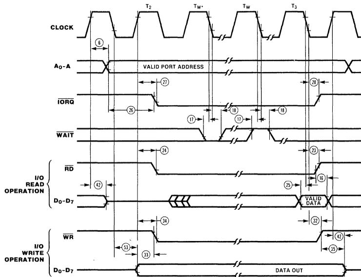
NOTE:  $T_w$ \* = One Wait cycle automatically inserted by CPU.
