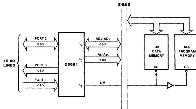
Figure 3. Z8681 Interfacing to Memory-Mapped I/O
