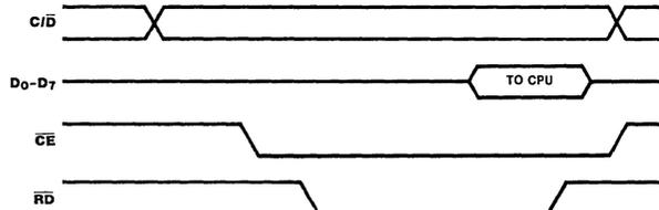
**Figure 9. Non-Z-BUS Read Cycle Timing**
