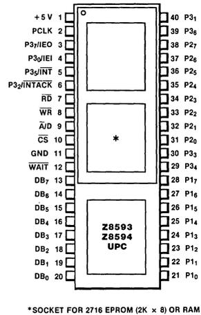
Figure 11. Z8593/Z8594 UPC Prototack Pin Assignments
