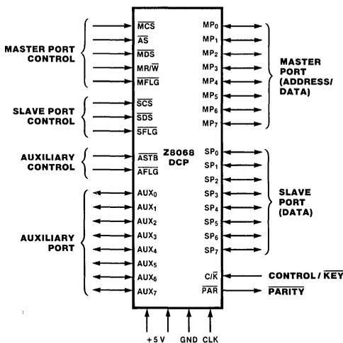
Figure 1. Pin Functions
