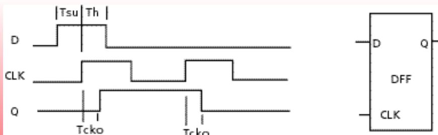
Figure 1 - Setup and hold timing.
