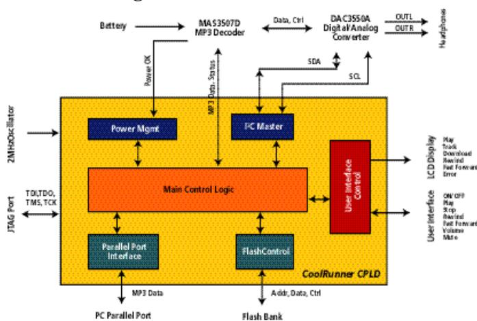
Figure 1 - MP3 portable player block diagram.
