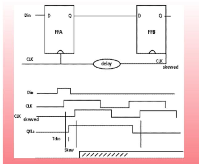
Figure 4 - Synchronous circuit with clock skew.
