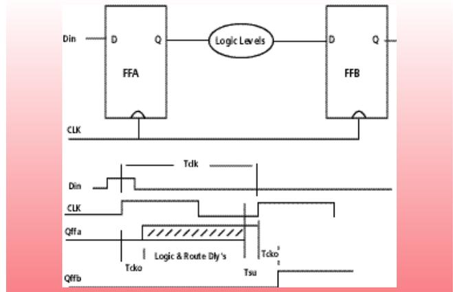
Figure 2 - Basic timing model.
