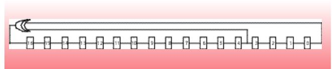
Figure 1 - A typical LFSR.
