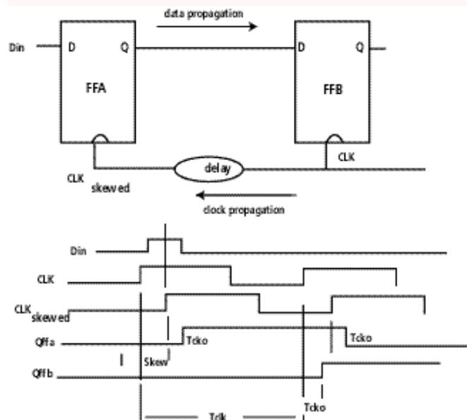
Figure 6 - Controlling the effects of clock skew through propagating the clock in the opposite direction.
