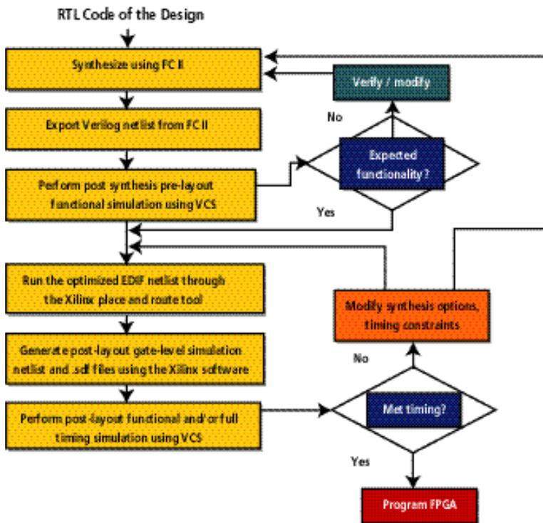
Figure 1 - Detailed design flow for Xilinx FPGA's
