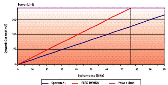
Figure 2: Dynamic power comparison of Spartan-XL device with 10K30A.
