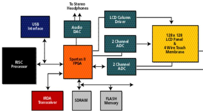
Figure 1: MP3 system block diagram.
