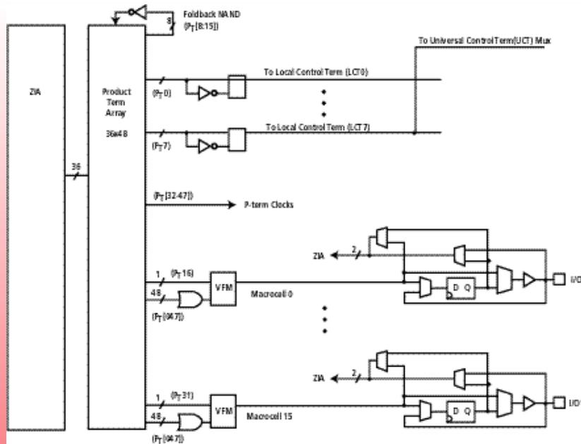
Figure 2 - XPLA3 Logic Block architecture.
