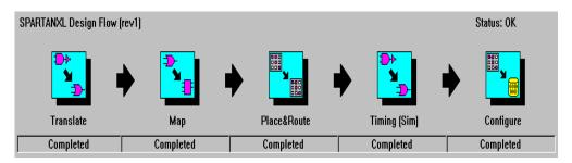
Figure 2-5 Flow Engine Shows All Design Segments Completed (FPGAs)
