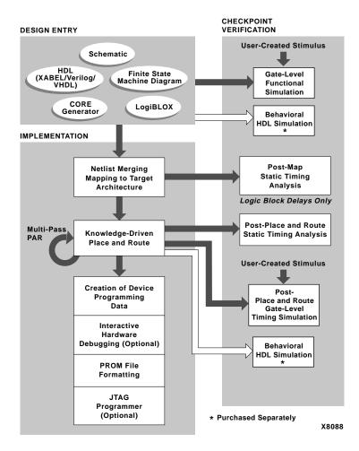
Figure 2-1 Foundation Overall Design Flow for FPGAs
