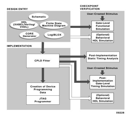
Figure 2-2 Foundation Overall Design Flow for CPLDs
