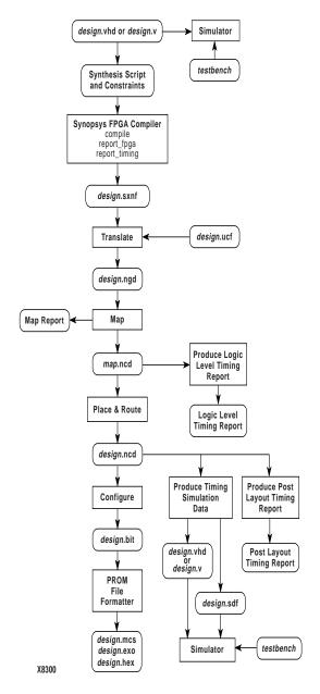
Figure 3-2 Design Flow Using the Design Manager
