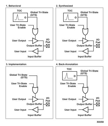
Figure 5-5 TOC Simulation and Implementation
