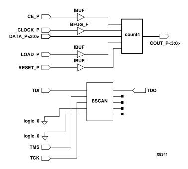
Figure 4-7 Bnd\_scan Schematic
