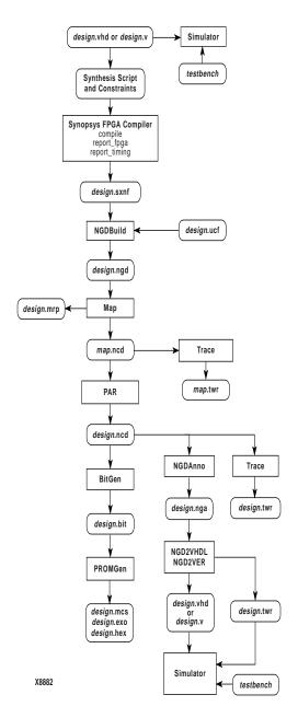
Figure 3-3 Design Flow using the Command Line
