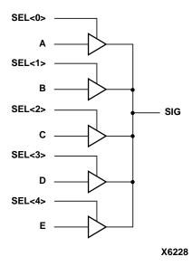
Figure 4-10 5-to-1 MUX Implemented with BUFTs
