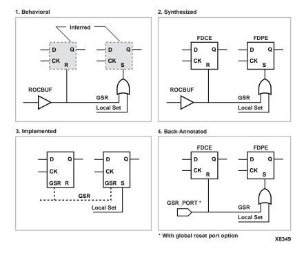
Figure 5-4 ROCBUF Simulation and Implementation
