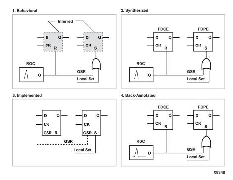
Figure 5-3 ROC Simulation and Implementation
