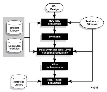
Figure 5-1 Three Simulation Points for HDL Designs
