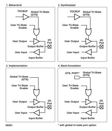
Figure 5-6 TOCBUF Simulation and Implementation
