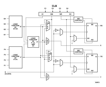
Figure 2-7 XC4000 Configurable Logic Block
