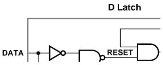
Figure 2-3 D Latch Implemented with Gates
