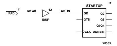
Figure 5-9 Verilog User-Controlled Inverted GR
