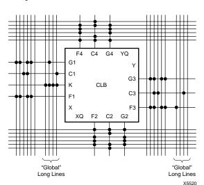
and G pins are the inputs to the F and G function generators, respectively.
