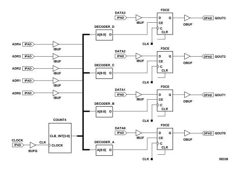
Figure 4-6 Schematic Block Representation of I/O Decoder
