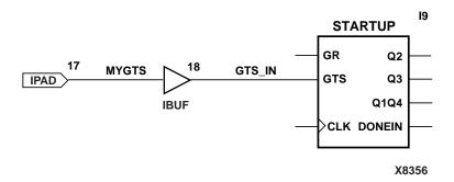
Figure 5-10 Verilog User-Controlled Inverted GTS
