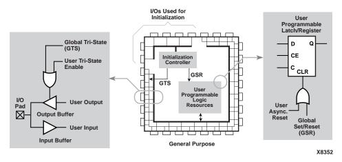
Figure 5-2 Built-in FPGA Initialization Circuitry
