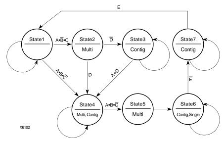
Figure 4-5 State Machine Bubble Diagram
