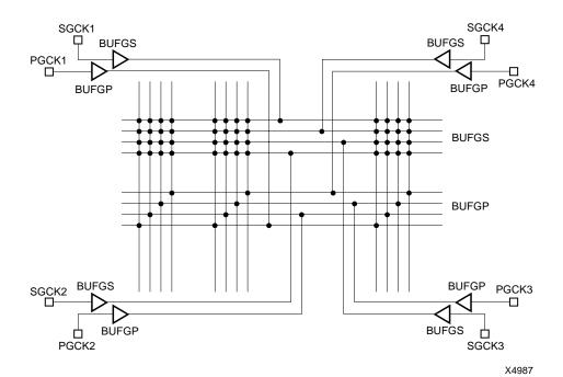
Figure 4-1 Global Buffer Routing Resources (XC4000E, Spartan)
