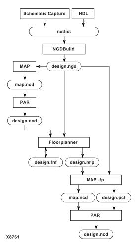
Figure 2-1 PAR Before Floorplanning Design Flow
