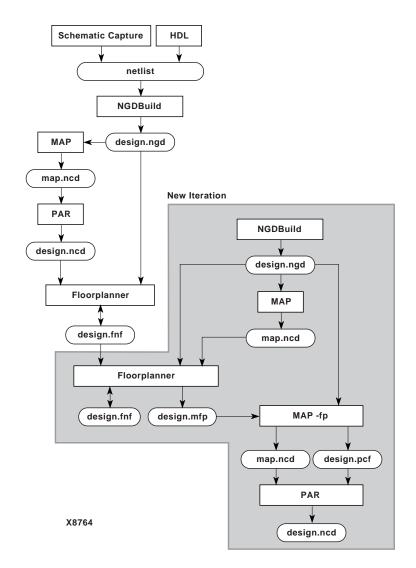
Figure 2-4 Incremental Design Change Design Flow
