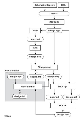
Figure 2-3 Iterative Floorplanning Design Flow
