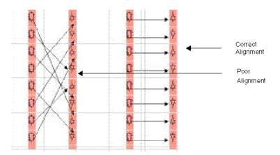
Figure 4-8 Flip-flop/BUFT Alignment Example
