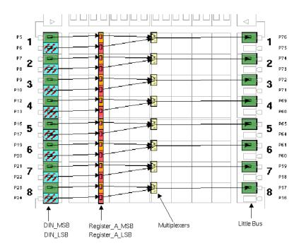
Figure 4-28 Final Placement of Interleave Design
