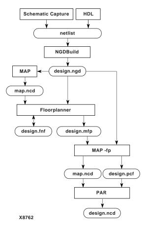
Figure 2-2 Floorplan First Design Flow
