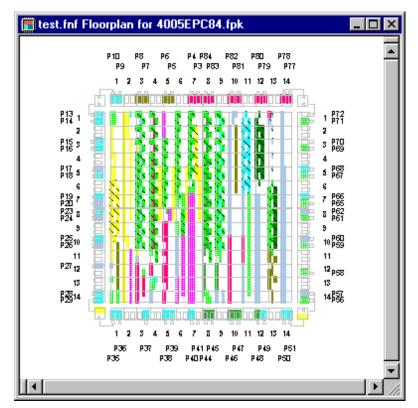
scrollable, scalable view of a resource map of the device that is specified in the design.
