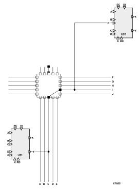
Figure 6-1 Routing Example
