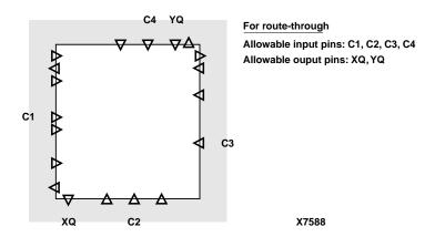
Figure 3-7 CLB Pins for Route-Throughs in XC4000/4000E Designs
