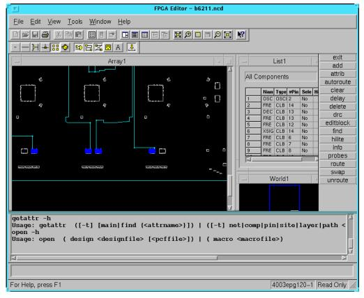
Figure 2-2 FPGA Editor Main Window
