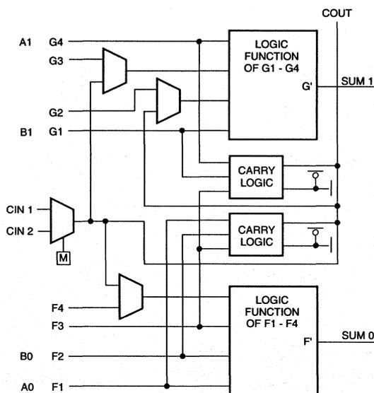
**Figure 2. XC4000 Fast Carry Logic in Each CLB**
