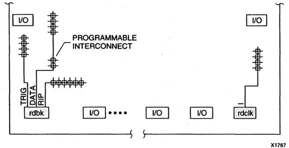
Figure 5. The XACT Readback Primitive
