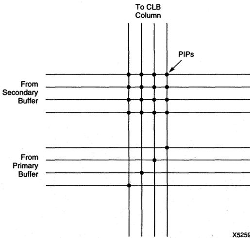
Figure 6. XC4000 Global Net Interconnection Matrix
