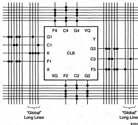
Figure 9. Longline Routing Resources with Typical CLB Connections
