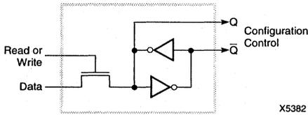
**Figure 2. Static Configuration Memory Cell.**
