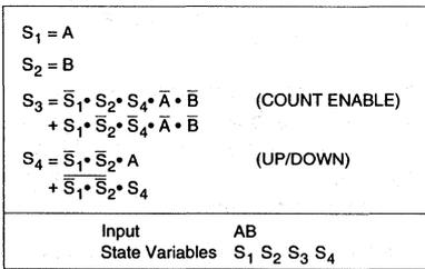
beam, the Count state is entered (S3 High) and the counter is enabled. One clock later, the state machine automatically moves out of the Count state and into the Wait state. If a new object is sensed from either direction during the Count state, the Wait state is omitted and the appropriate sequence commenced.
