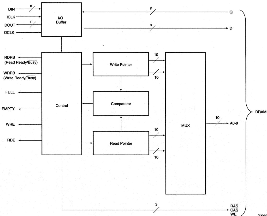
**Figure 1. Megabit FIFO Controller in an XC3020**
