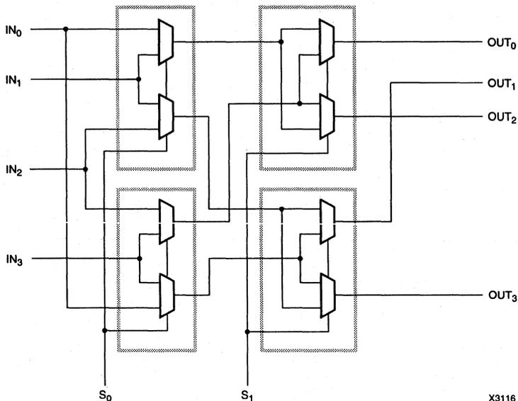
Figure 5. 4-Bit Barrel Shifter
