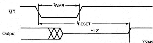
Figure 4. Global Reset Waveform
