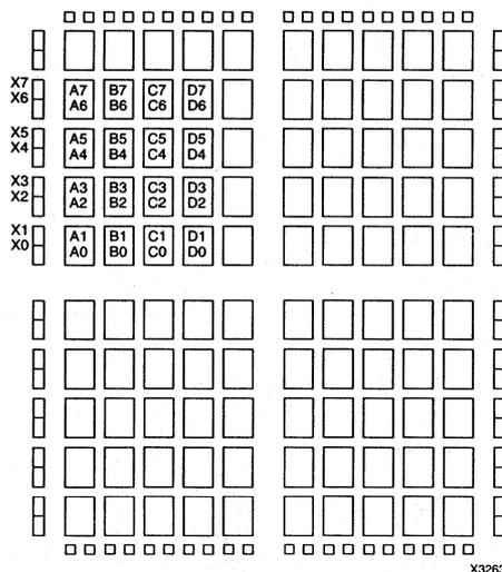
Figure 15. Efficient Placement in an XC4003
