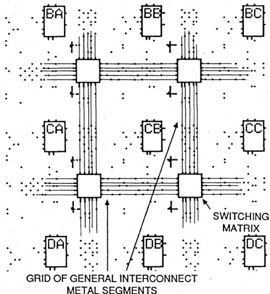
**Figure 9. LCA General-Purpose Interconnect.**
