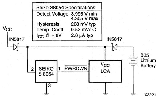
Figure 9. Battery Back-up Circuit
