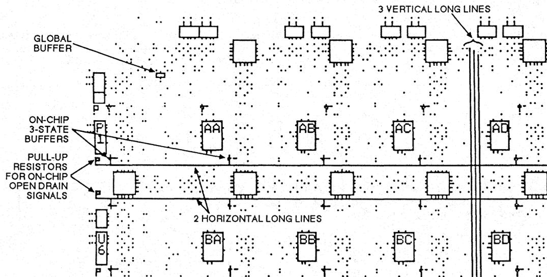
**Figure 13. Horizontal and Vertical Longlines.** These Longlines provide high fan-out, low-skew signal distribution in each row and column. The global buffer in the upper left die corner drives a common line throughout the LCA device.
