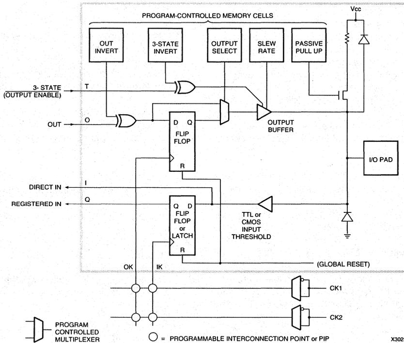
**Figure 3. Input/Output Block.**
