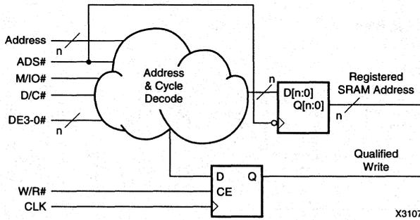
Figure 14. Modified Write Cycle Logic
