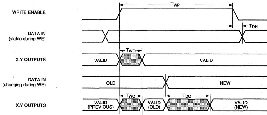
READ DURING WRITE, CLOCKING DATA INTO FLIP-FLOP
