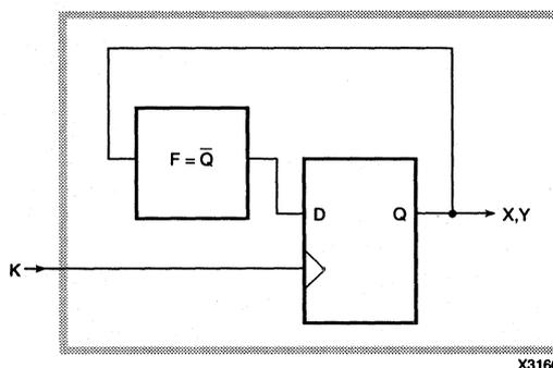
**Figure 17. Logic Block Configuration for Toggle Rate Measurement**
