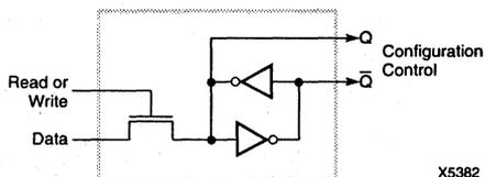
Figure 2. Configuration Memory Cell
