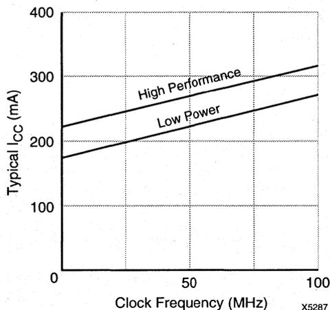
Figure 2. Typical  $I_{CC}$  vs Frequency for XC7372
