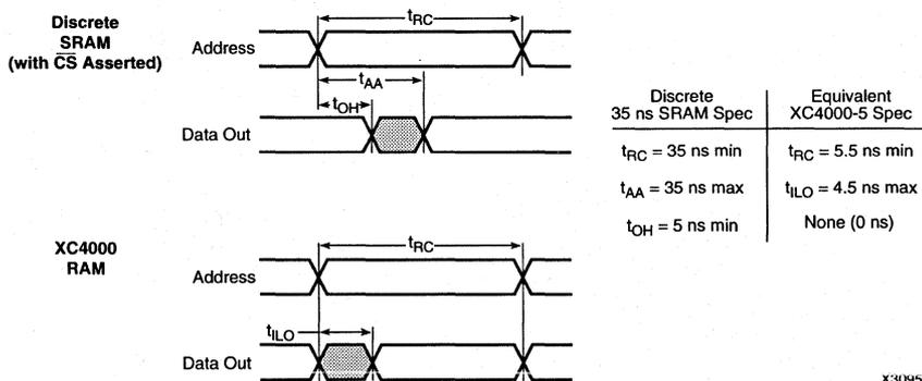
**Figure 2. XC4000 RAM and Discrete SRAM Read Cycles**
