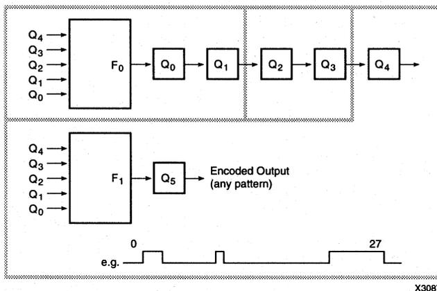
Figure 2. Synchronous 5-Bit Waveform Generator in 3 CLBs
