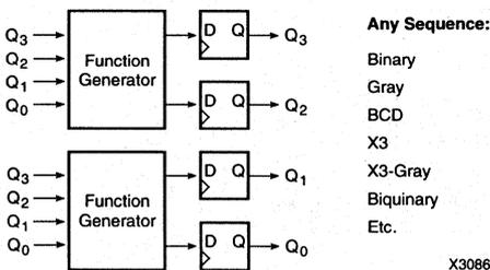
Figure 1. Synchronous 4-Bit Counter in 2 CLBs
