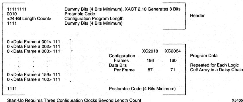
Figure 12. XC2064 Internal Configuration Data Arrangement
