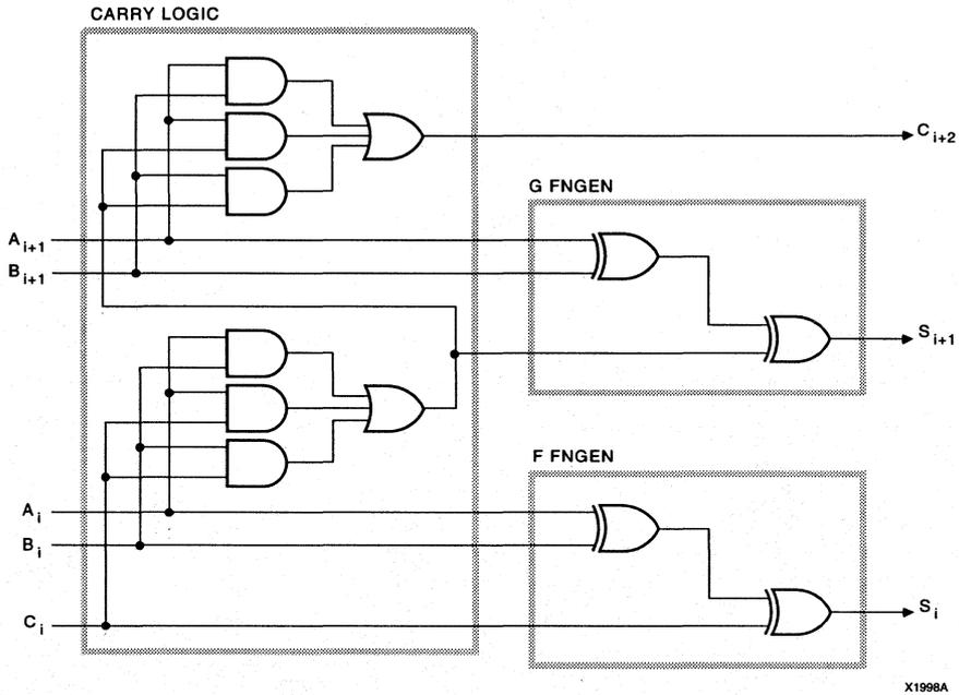
Figure 2. Conceptual Diagram of a Typical Addition (2 Bits/CLB)
