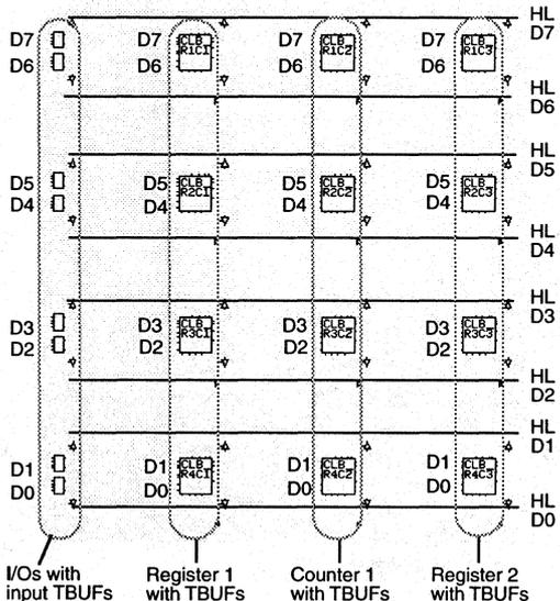
Figure 14. Bit Alignment for 3-State Bussing
