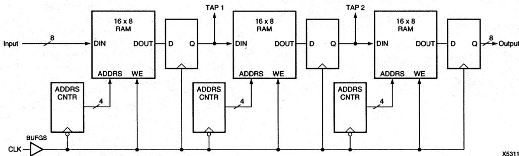
Figure 3. Byte-wide RAM-based Shift Register
