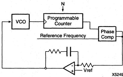
Figure 1. Typical Digital Phase-Locked Loop
