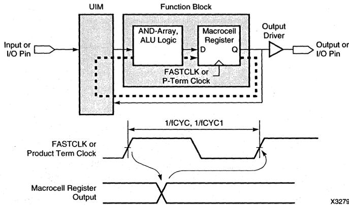
Figure 6. Delay Path Specifications for  $f_{CYC}$  and  $f_{CYC1}$
