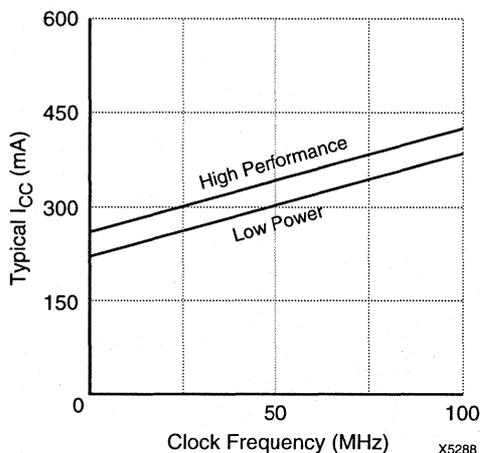
Figure 2. Typical  $I_{CC}$  vs Frequency for XC73108
