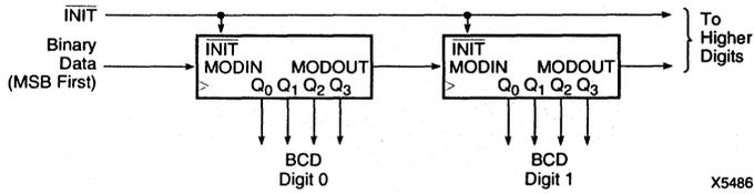
Figure 1. Binary-to-BCD Converter
