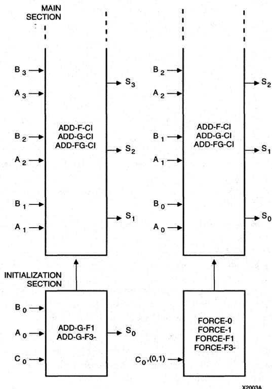
Figure 6. Main and Initialization Sections of Adder
