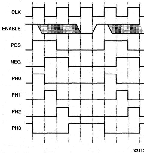
Figure 17. Waveforms for the Glitch-Free Sequencer
