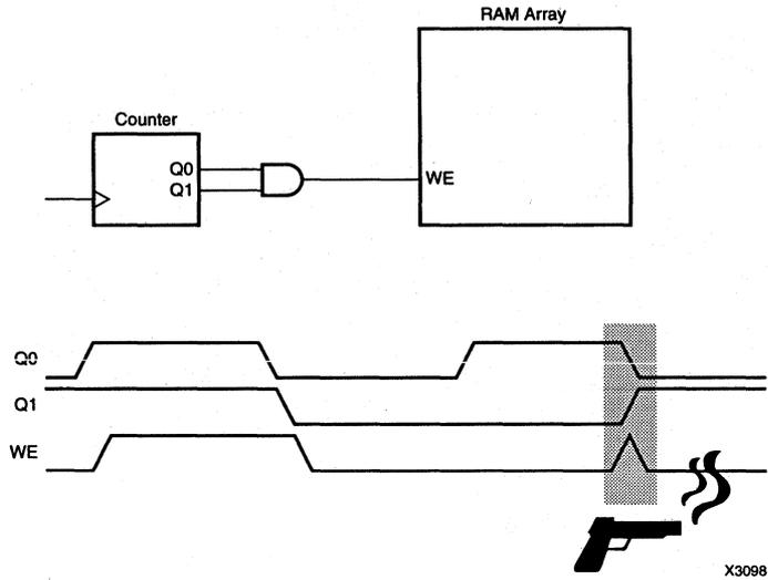
Figure 5. Example of a Marginal WE Generation Circuit
