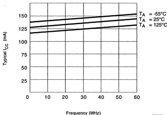
**Figure 4. Typical  $I_{CC}$  vs Frequency for XC7236A Configured as Eight 4-bit Counters**
