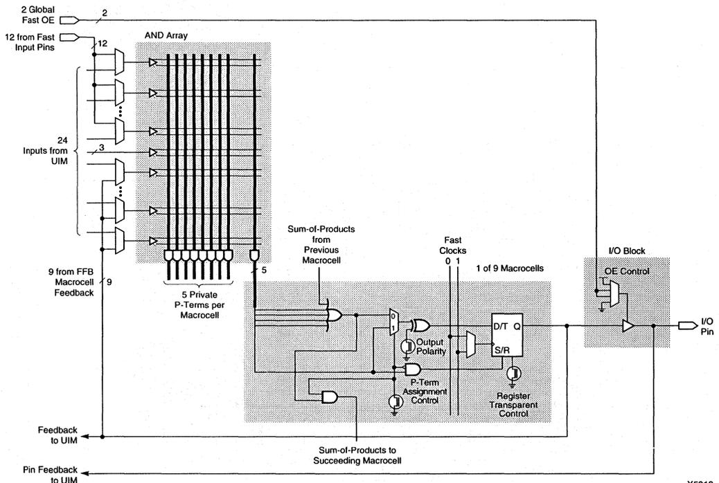
Figure 2. Fast Function Block and Macrocell Schematic
