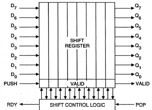
Figure 1. 8-Word x 8-Bit Synchronous FIFO (40 CLBs)
