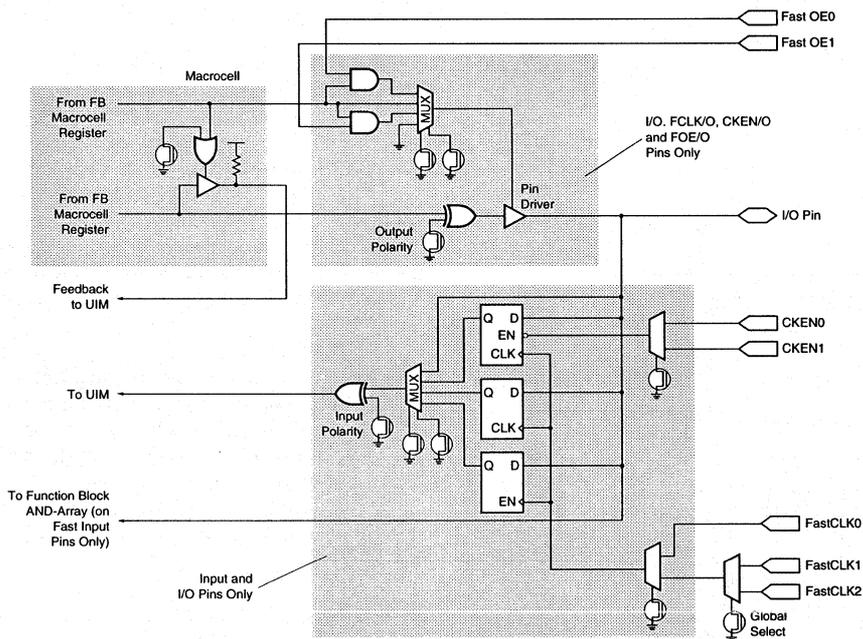
Figure 7. Input/Output Schematic
