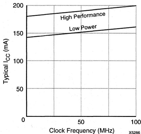
Figure 2. Typical  $I_{CC}$  vs Frequency for XC7354
