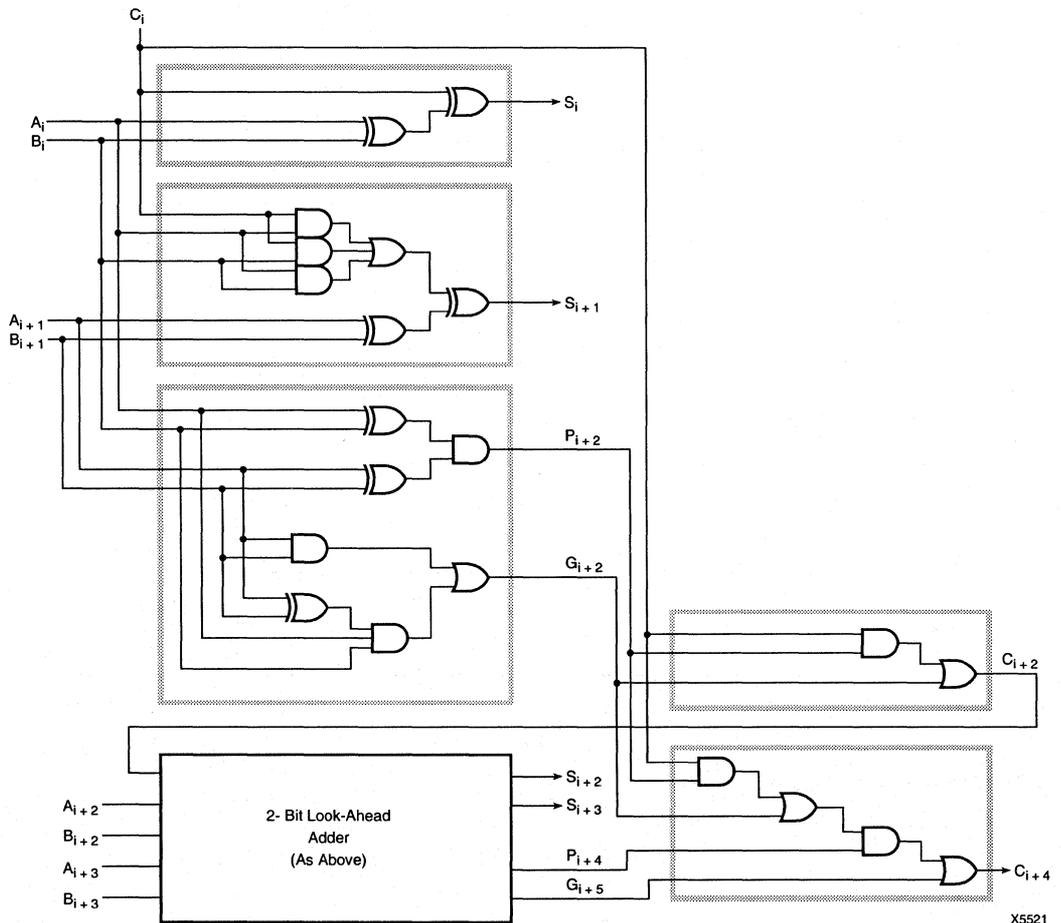
Figure 7. Four-Bits-at-a-time Adder Block with Internal Look-Ahead Carry
