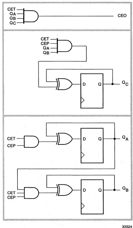
Figure 2b. All More Significant Tri-bits Use Three CLBs
