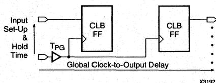
Timing is measured at pin threshold, with 50 pF external capacitive loads (incl. test fixture).
