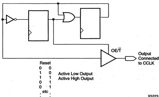
the extra CCLK pulse. This solution requires one CLB, one IOB and pin, and an internal oscillator with a frequency of up to 5 MHz as available clock source. Obviously, this XC3000 master device must be configured with late Internal Reset, which happens to be the default option.
