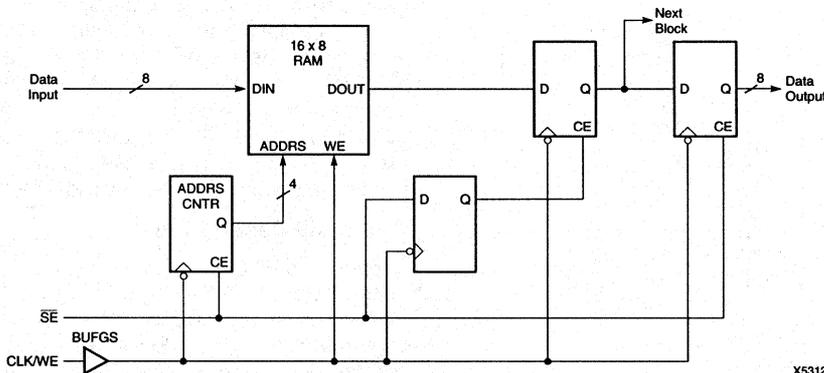
Figure 4. RAM-Based Shift Register with Shift Enable
