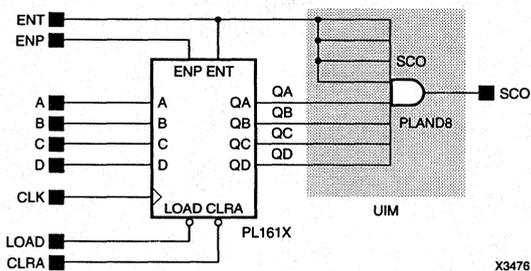
Figure 1. Typical 4-Bit Up-Counter Component
