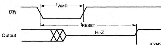
Figure 4. Global Reset Waveform
