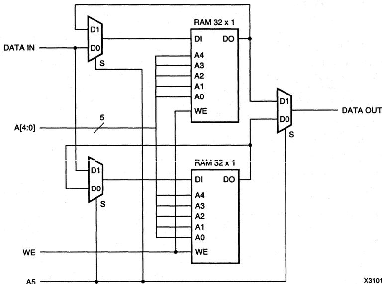
Figure 8. Alternative 64 x 1 RAM Array
