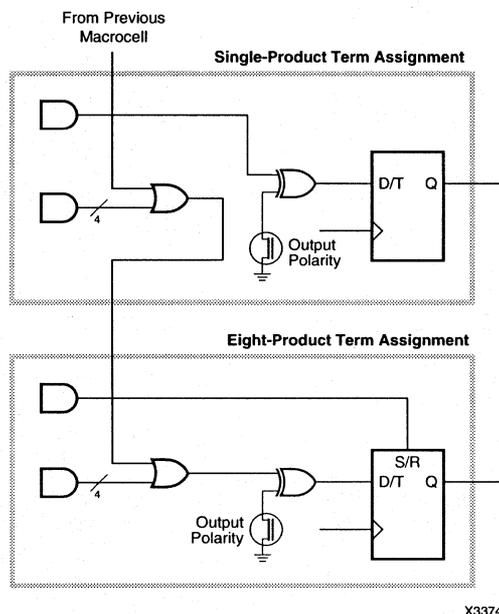
Figure 3. Fast Function Block Product Term Assignment
