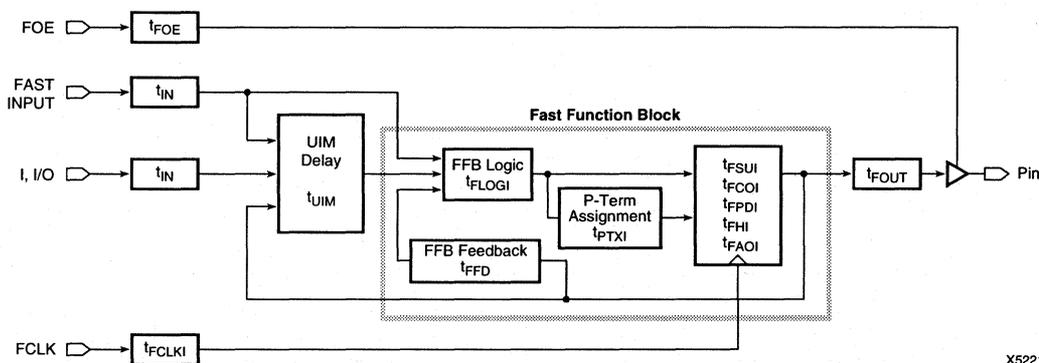
Figure 7. XC7318 Timing Model
