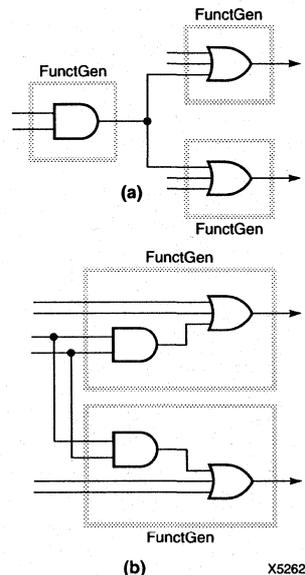
Figure 11. Improving Logic Partitioning by Gate Duplication
