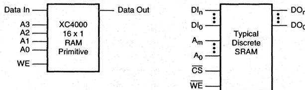
Figure 1. XC4000 RAM and Discrete SRAM Connections
