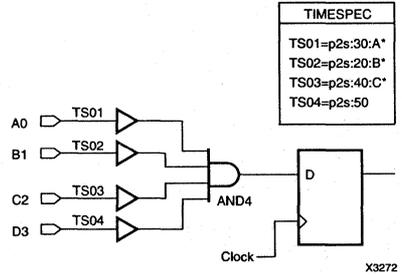
Figure 18. TIMESPEC Placement Where Some Specifications are Lost
