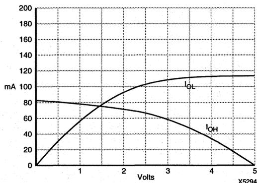
Figure 4. Output Current/Voltage Characteristics for XC3020
