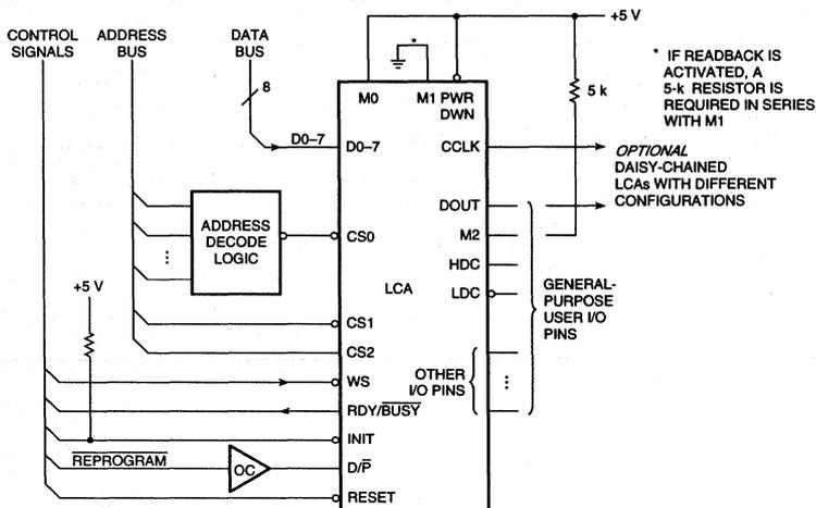
Figure 23. Peripheral Mode.
