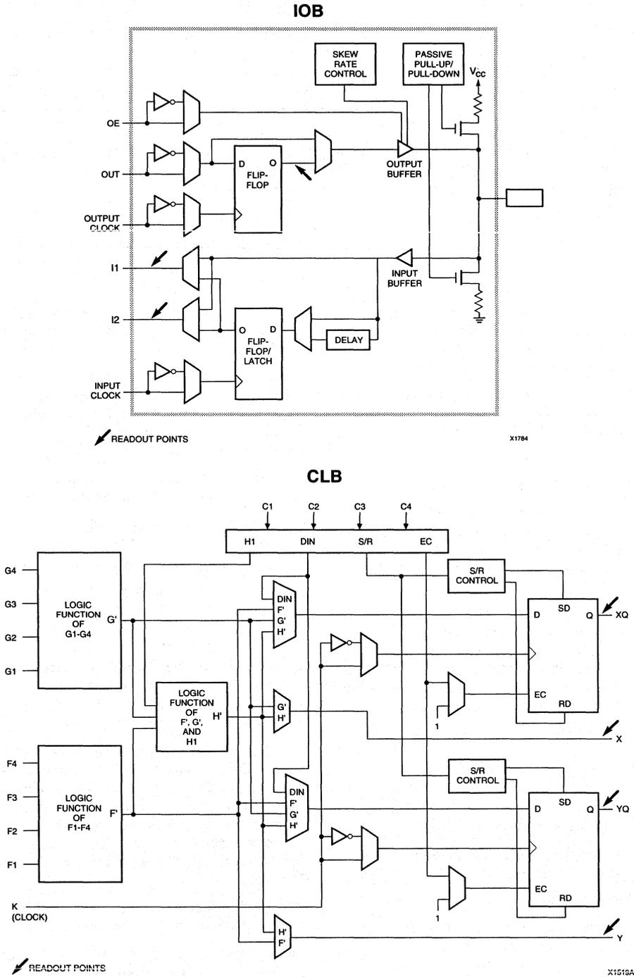
Figure 1. Readback Capture Enable
