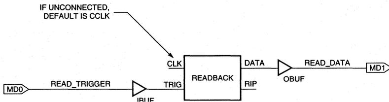
Figure 4. Readback Symbol on the Design Schematic
