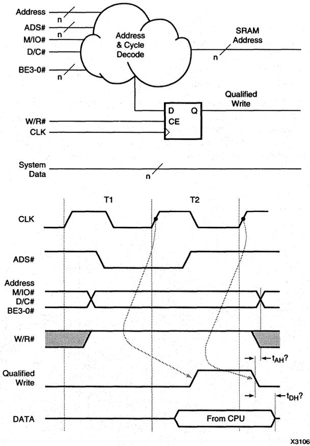
Figure 13. Write Cycle Control Logic and Timing
