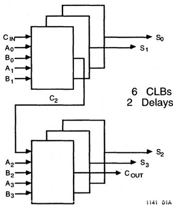
Figure 10. 4-Bit Adder
