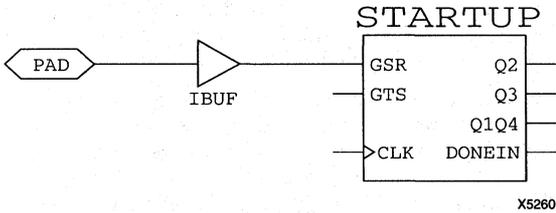
Figure 9. Schematic Symbols for Global Set/Reset
