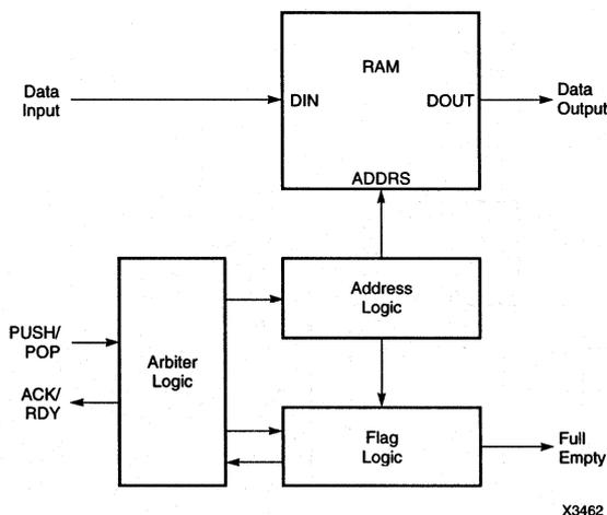
Figure 1. FIFO Block Diagram
