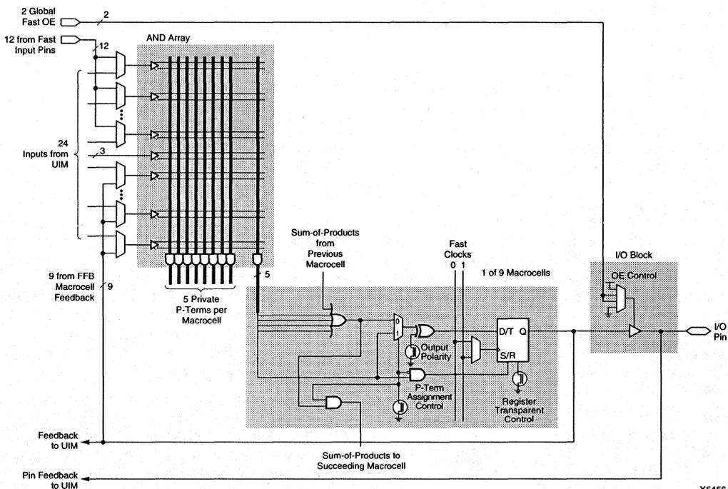
Figure 2. Fast Function Block and Macrocell Schematic for the XC7318/XC7336/XC73144
