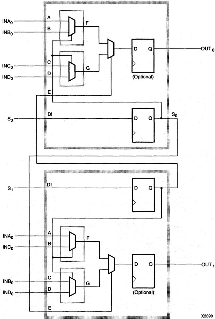
Figure 1. Dual 4:1 Multiplexer with Pipelined Select (Two CLBs)
