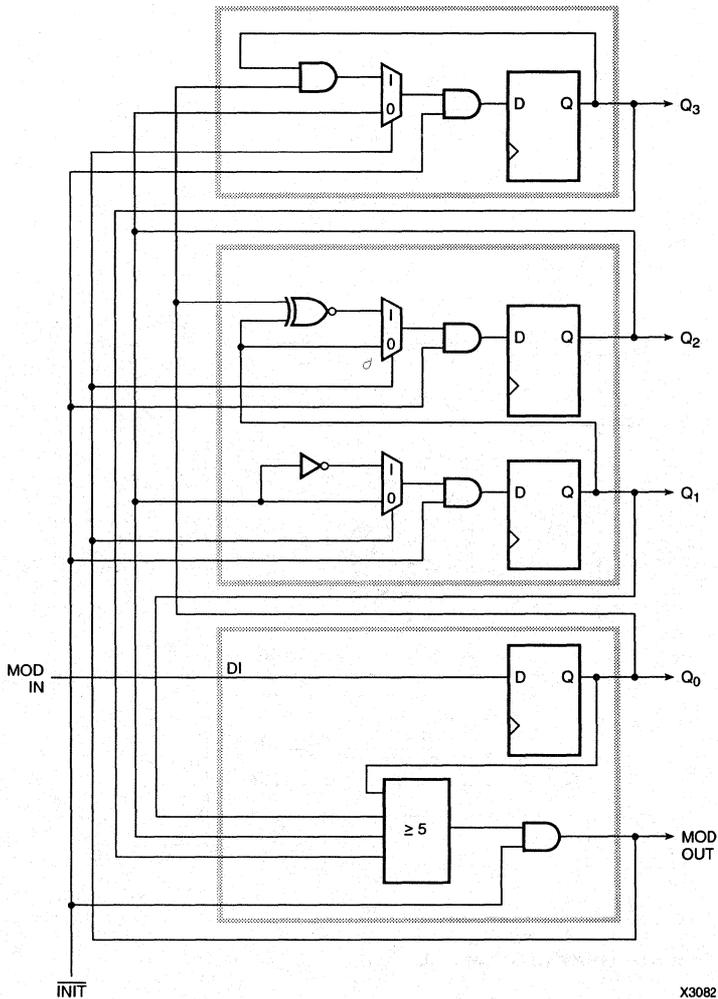
Figure 2. Binary-to-BCD Converter (Three CLBs per BCD Digit)
