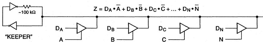
**3-State Buffers Implement a Multiplexer.** The selection is accomplished by the buffer 3-state signal. X1007
