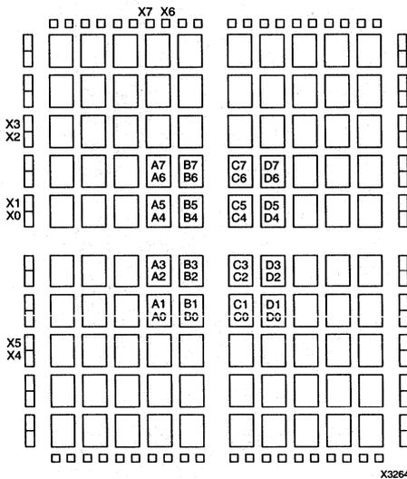
Figure 16. Inefficient Placement in an XC4003
