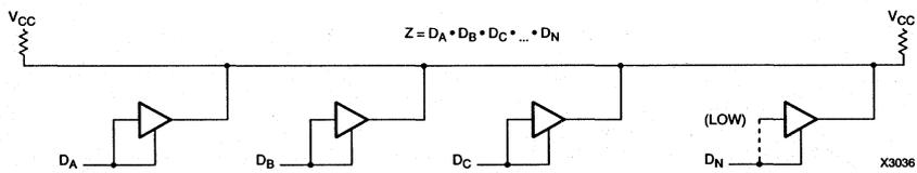
**Figure 15a. 3-State Buffers Implement a Wired-AND Function.** When all the buffer 3-state lines are High, (high impedance), the pull-up resistor(s) provide the High output. The buffer inputs are driven by the control signals or a Low.
