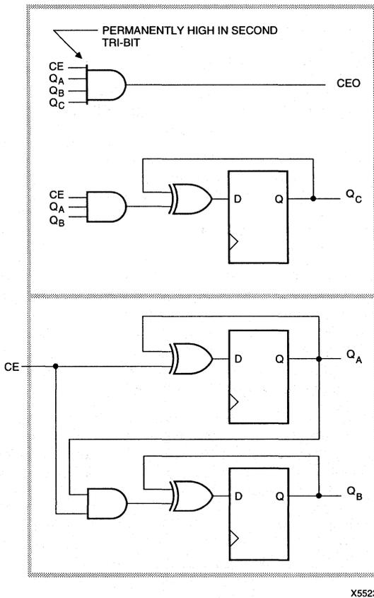
Figure 2a. First and Second Tri-bits Use Two CLBs Each
