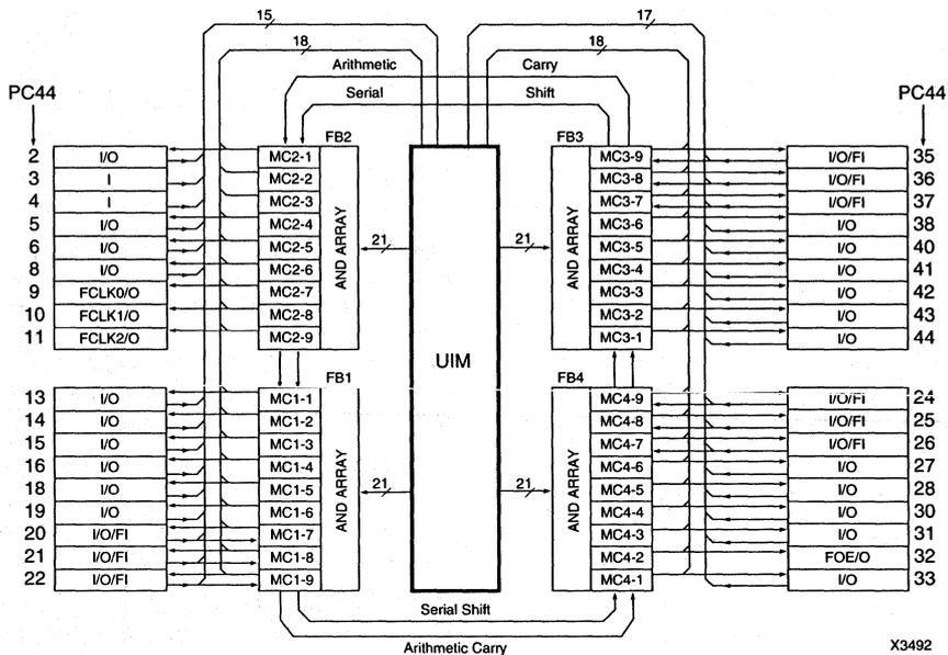
Figure 1. XC7236A Architecture
