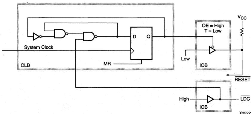
**Figure 5. Synchronous Reset**
