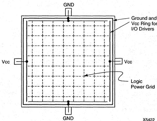
Figure 21. LCA Power Distribution
