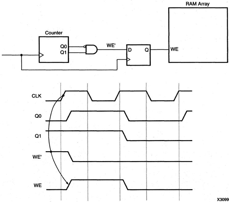
Figure 6. Example of a Glitch-Free WE Generation Circuit
