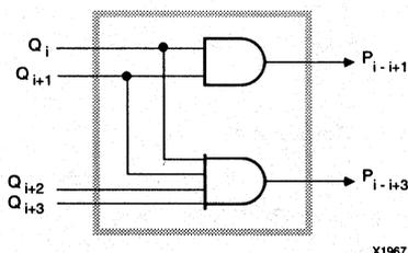
Figure 3. Propagate Cell
