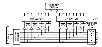
Figure 2) Typical DIP switch interface for multiple packages.
