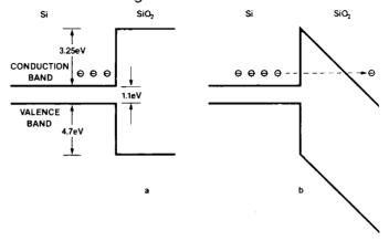
Figure 7. Energy band diagrams of the  $Si/SiO_2$  system in the neutral state (a), and during the store operation (b).
