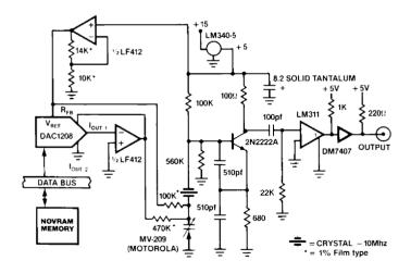
Figure 10) Tuneable crystal oscillator.
