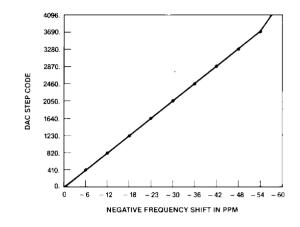
Figure 11) Tuning range of the tuneable crystal oscillator of Figure 10.
