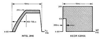
Figure 6) Comparison of timing and level requirements of the high voltage pulse between the Intel 2816 and the Xicor X2816A. The shaded portion indicates the operating range of each part.
