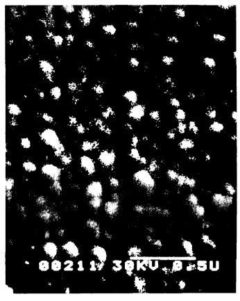
Figure 9. Scanning electron microscope (S.E.M.) photograph of top emitting textured poly surface with oxide removed. The 0.5  $\mu$ -long bar gives the scale
