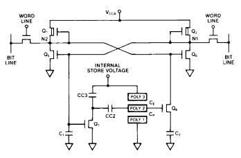
Figure 6. Schematic diagram of a NOVRAM memory cell showing how a standard six-transistor static RAM cell is merged with a floating gate  $E^2$ PROM cell.
