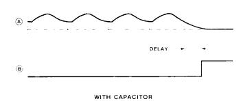
Figure 6) A capacitor in the circuit of Figure 4 fills in the valley in the rectified ac to produce a pulse only when ac disappears.
