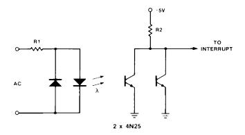
Figure 7) Two optoelectronic isolators are connected with their diodes back to back to provide an interupt signal.
