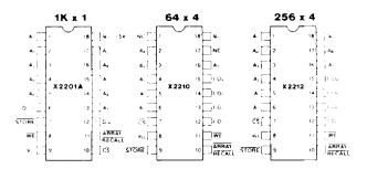
Figure 3) Pin configuration of the XICOR NOVRAM family.
