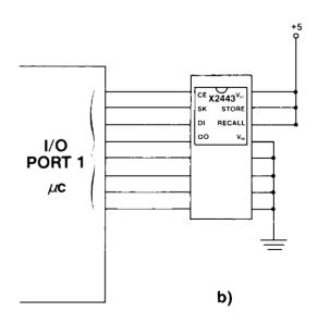
Figure 1. Microcomputer with Internal Pullups
