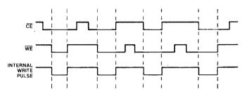
Figure 4) The internal write pulse is generated by the simultaneous LOW of both  $\overline{CE}$  and  $\overline{WE}.$
