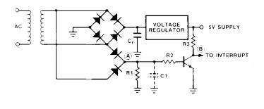
Figure 4) A circuit to detect the absence of ac.
