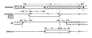
Figure 5) Timing diagram for the Xicor EEPROM byte write cycle.
