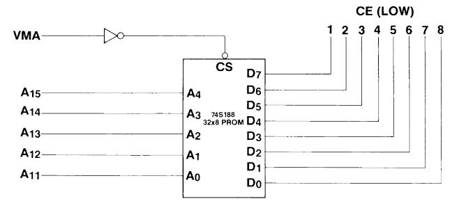
One simply changes the program in the PROM to go from using X2816A's to X2864A's. The listing on the following page shows the PROM program for the X2816A's and the X2864A's.
