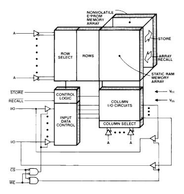
Figure 1) NOVRAM memory block diagram.
