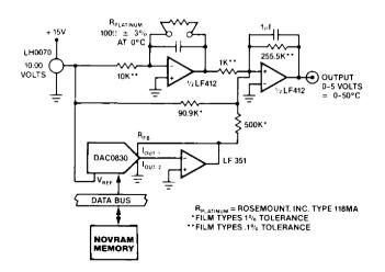
The NOVRAM memory/DAC combination is used to modify the offset voltage of the amplifier to allow full interchangeability of probes in the field.
