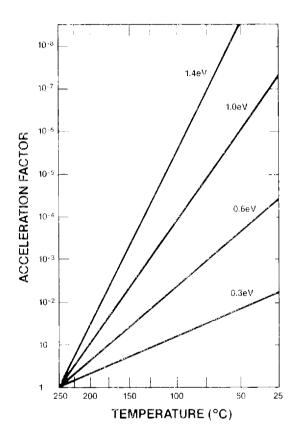
Figure 18. Acceleration factor vs. temperature calculated for various activation energies from Arrhenius relation.
