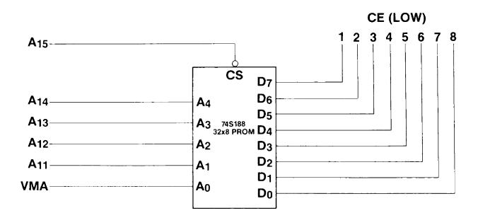
One simply changes the PROM for replacing the X2816A's with X2864A's.
