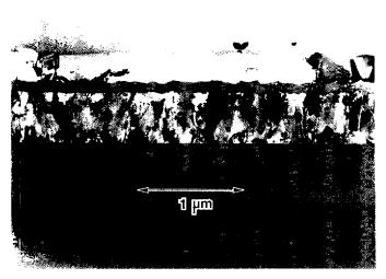
Figure 10. Transmission electron microscope photograph of a crosssection through a textured tunneling structure. The one micron-long arrow shows the scale.
