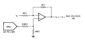
Figure 5) The DAC output provides up to 100 millivolts of trim for the operational amplifier output voltage.
