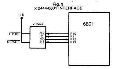
lines and software. Housed in an eight-pin mini-DIP, the X2444 provides inexpensive non-volatile data storage for both operational and configuration parameters. Its low cost (less than \$4.00 in unit quantities) makes it the least expensive non-volatile storage on the market, even rivalling the DIP switch in unit cost, while providing the equivalent of 32 DIP switches in terms of data capacity.
