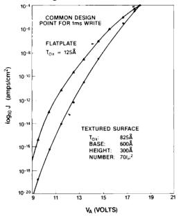
Figure 14. Comparison of calculated tunneling J-V curves for emission from a planar and a textured structure. The devices were designed to have the same emission in the high current regime where programming takes place.
