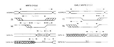
Figure 4) Timing diagram for Writing to the RAM.
