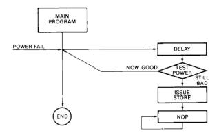
Figure 17: The program branches to a STORE subroutine when a power failure is detected.
