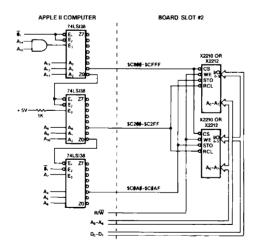
Figure 8) Connections for operating the NOVRAM on the I/O Bus of an APPLE II computer.
