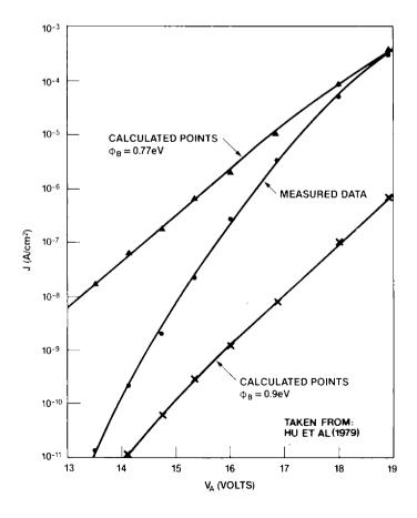
Figure 8. Current vs. applied voltage for current from textured poly surface emitted through 1760 Å of thermal Si0<sub>2</sub> compared with calculations based on previously available theory.
