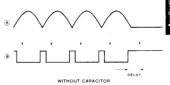
Figure 5) Waveforms in the circuit of Figure 4 without the capacitor. The microprocessor is interupted every 8.3ms and must check 2ms later to determine if the power loss is real.
