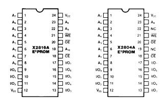
Figure 1) Pinouts of the Xicor family of EEPROMs.
