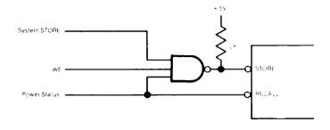
Figure 9) A power supply status line held LOW can insure that both the RECALL pin is held LOW and the STORE pin is held HIGH.
