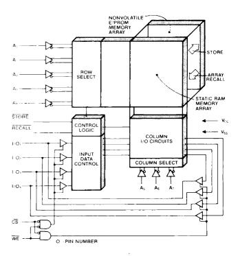
Figure 2. Functional diagram of X2212 memory
