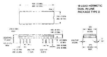
Figure 3. Package outline drawing for memories in cerdip
