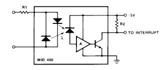
Figure 10) The MID400 requires only two resistors to connect directly to the ac power line.
