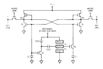
Figure 2) Circuit diagram of a NOVRAM cell.
