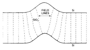
Figure 11. Sketch illustrating the manner in which field lines converge near convex feature and diverge near concave features.
