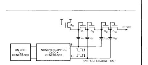
**Fig B—A 32-stage charge pump** internally generates a NOVRAM's high Store voltage, allowing the device's NOVRAM and EEPROM sections to operate from 5V.
