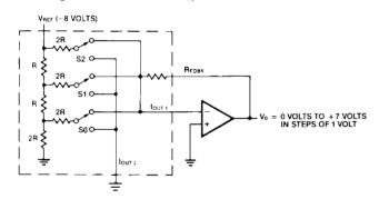
Figure 7) A simplified 3-switch CMOS DAC.
