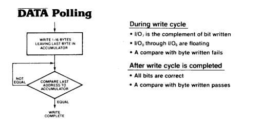
Since, prior to nonvolatile write cycle completion, the MSB is inverted, the comparison test will fail and the loop will continue. When the write cycle is complete, the comparison test will succeed and control will fall out of the loop. The user may then access the memory for the next read or write operation.
