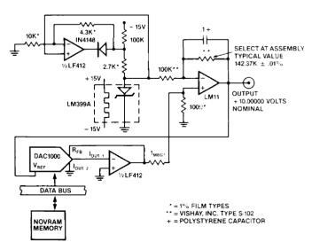
Figure 12) Software programmable voltage reference.
