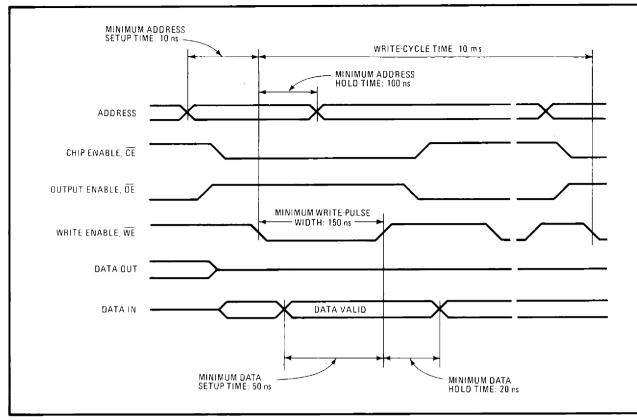
2. Like a static RAM. The write-cycle timing for the X2816A EE-PROM looks much like that for a static random-access memory. Although the write cycle takes a maximum of 10 ms, latches hold the address and data signals, freeing the processor for other tasks.
