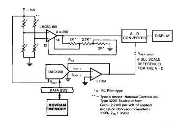
Figure 13) Self-calibrating, interchangeable probe thermometer.
