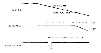
Figure 3) Falling dc is detected to trigger a STORE pulse at least 10ms before the  $\pm$  5 Volt supply drops below 4.5 Volts.
