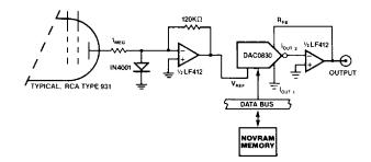
Figure 15) Gain trimming for photomultiplier tubes.
