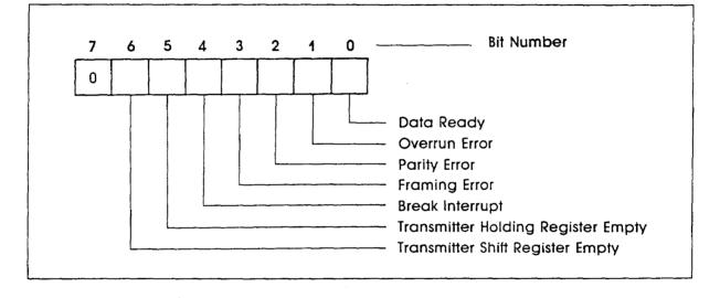
**Bit 0:** This bit is the receiver data ready (DR) indicator. It is set to logical 1 whenever a complete incoming character has been received and transferred into the Receiver Buffer register. Bit 0 may be reset to logical 0 by the processor either reading the data in the Receiver Buffer register or writing logical 0 in it.
