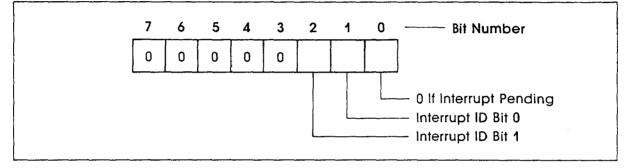
**Bit 0:** The bit can be used in either a hardwired prioritized or polled environment to indicate whether an interrupt is pending. When bit 0 is logical 0, an interrupt is pending, and the IIR contents may be used as a pointer to the appropriate interrupt service routine. When bit 0 is logical 1, no interrupt is pending, and polling (if used) continues.
