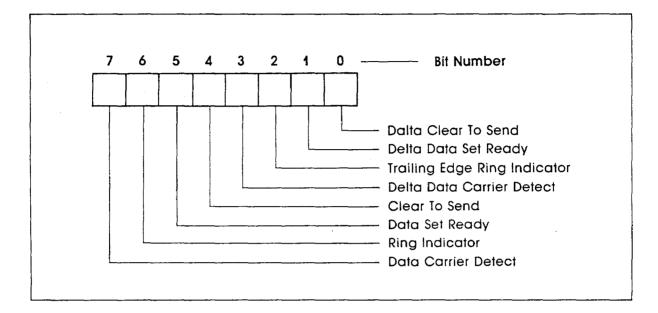
Bit 0: This bit is the delta clear-to-send indicator. It indicates the  $\overline{\text{CTS}}$  input to the chip has changed state since the last time it was read by the processor.
