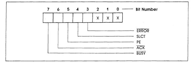
Bit 7: BUSY—This signal may become active during data entry, while the printer is offline, during printing, when the print head is changing positions, or while in an error state. When it is active, the printer is busy and can not accept data.
