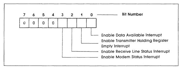
Bit 0: When set to logical 1, enables the received-data-available interrupt.
