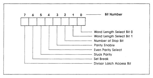
Bits 0, 1: These two bits specify the number of bits in each serial character that is sent or received. The encoding of bits 0 and 1 is as follows:
