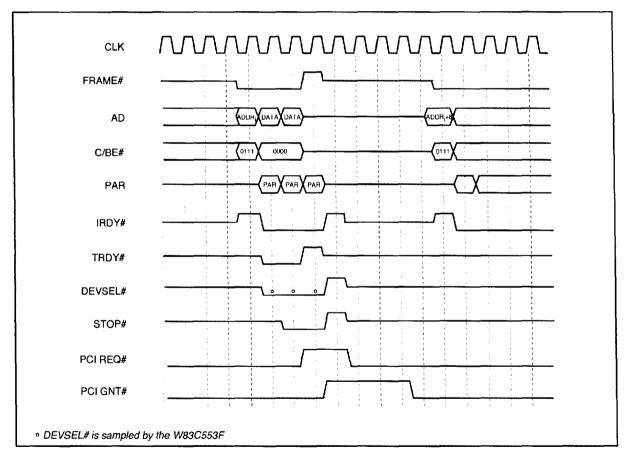
Figure 3-9. Disconnect With Data Transfer Timing
