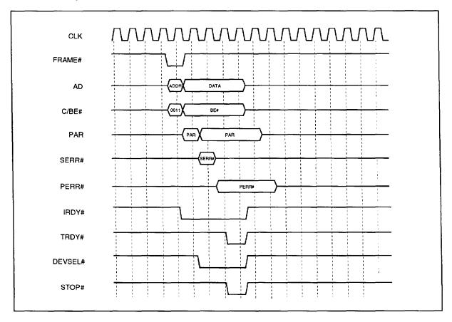
Figure 3-3. Slave I/O Write Timing
