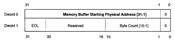
Bit 31 of Dword 1 is the end of Link Flag. Bus master operation terminates upon completion of the description entry that has EOL set.
