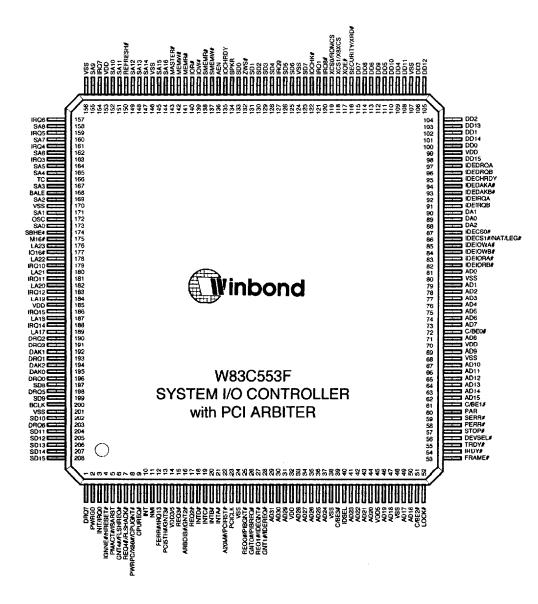
Figure 2-1. Pin Assignments for the W83C553F
