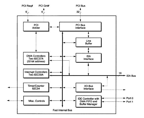
Figure 1-1. W83C553F Enhanced System I/O Controller Block Diagram
