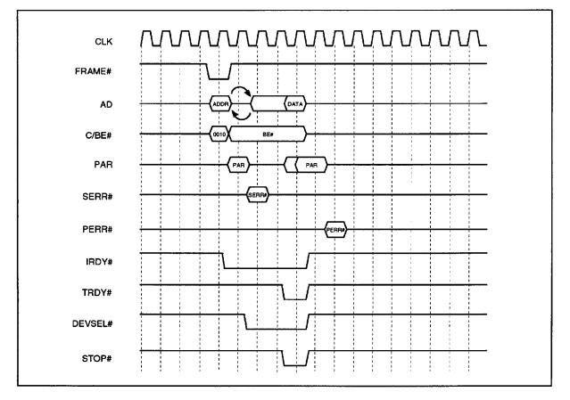
Figure 3-2. Slave I/O Read Timing
