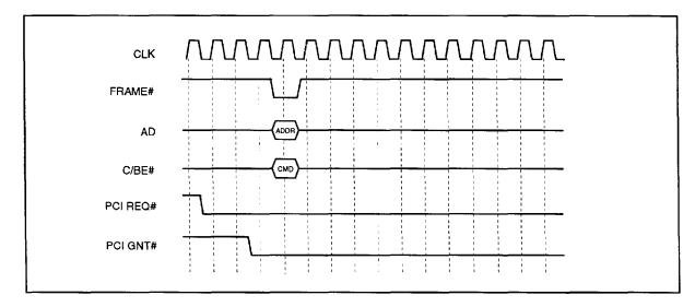
Refer to Figure 3-1. Bus acquisition timing cycles are defined by the CBE[3:0]# command lines during the address (AD) phase of each PCI cycle.
