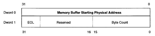
For a 16-bit DMA I/O device, bit 0 of the Memory Buffer Starting Address and byte count must be 0.
