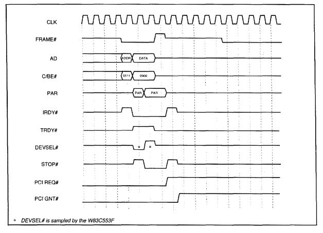
Figure 3-11. Target Abort Timing
