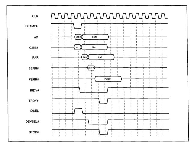
Figure 3-5. Slave Configuration Write Timing
