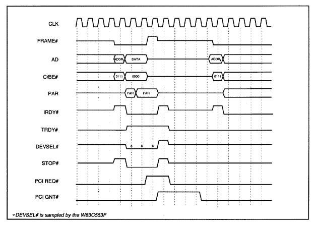
Figure 3-10. Disconnect Without Data Transfer Timing
