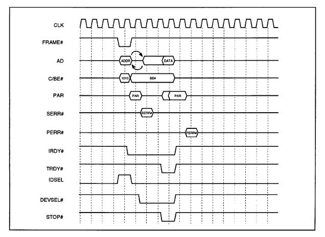
Figure 3-4. Slave Configuration Read Timing
