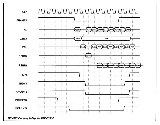
Figure 3-8. Master Memory Read Line Timing
