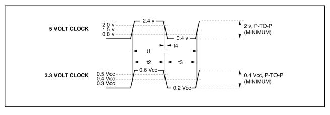
Note: For 5V PCI Bus, measurements were taken from 0.4V to 2.4V. All  $V_{DD}$  are 4.75V to 5.25V
