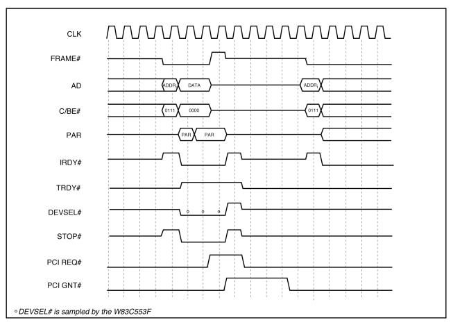
Figure 3-10. Disconnect Without Data Transfer Timing
