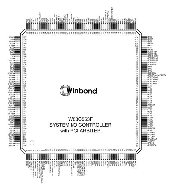
Figure 2-1. Pin Assignments for the W83C553F
