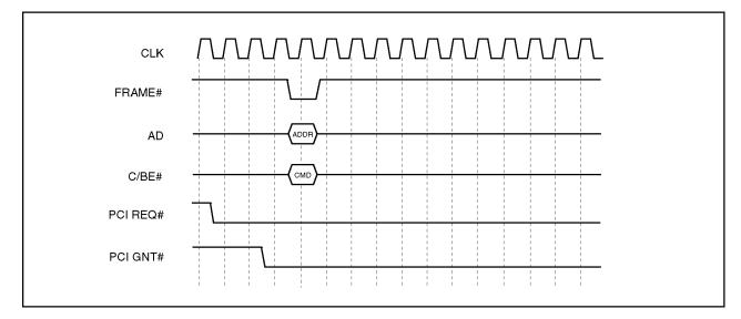
Figure 3-1. Bus Acquisition Timing
