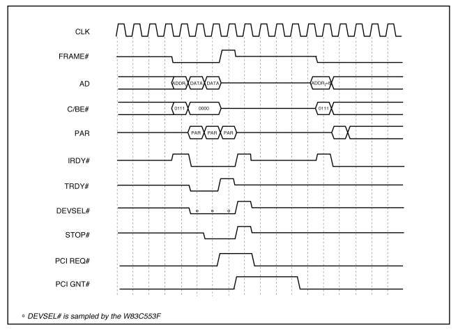
Figure 3-9. Disconnect With Data Transfer Timing
