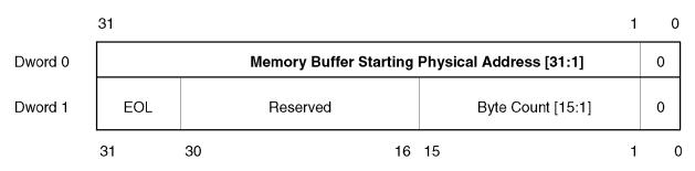
Bit 31 of Dword 1 is the end of Link Flag. Bus master operation terminates upon completion of the description entry that has EOL set.
