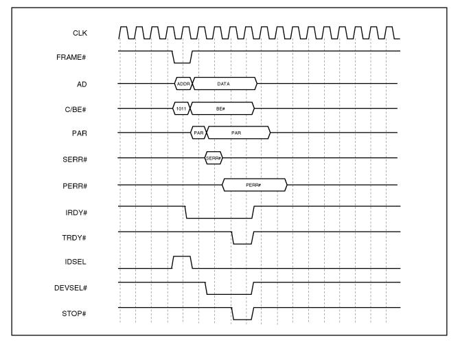
Figure 3-5. Slave Configuration Write Timing
