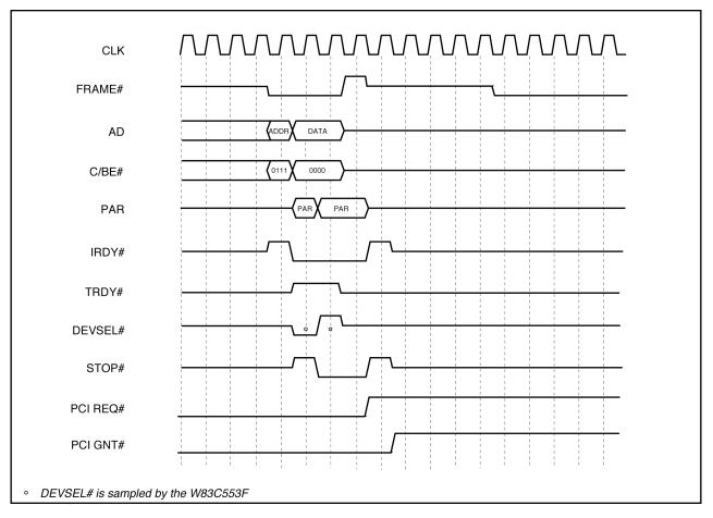
Figure 3-11. Target Abort Timing
