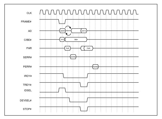
Figure 3-4. Slave Configuration Read Timing
