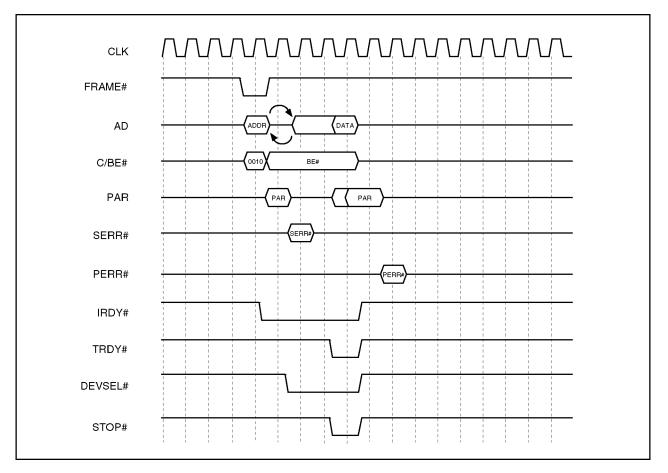
Figure 3-2. Slave I/O Read Timing
