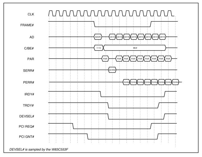
Figure 3-8. Master Memory Read Line Timing
