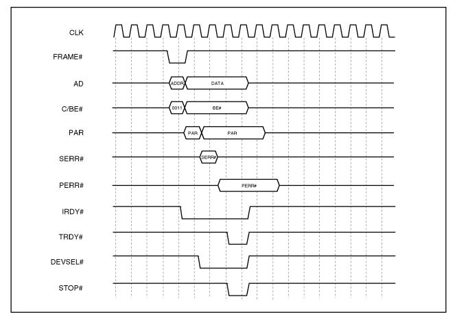
Figure 3-3. Slave I/O Write Timing
