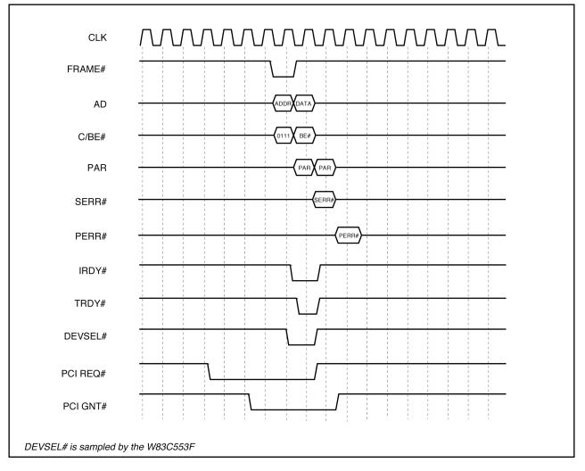
Figure 3-7. Master Memory Write Timing
