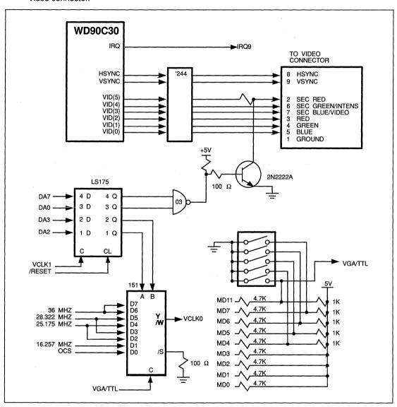
FIGURE 22, WD90C30 AND TTL MONITOR CONNECTIONS
