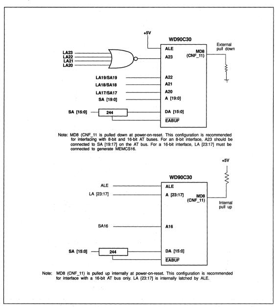
FIGURE 18. WD90C30 INTERFACE FOR 286 OR 386-BASED SYSTEMS
