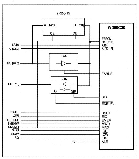
FIGURE 14. 8-BIT PC AT INTERFACE WITH 8-BIT BIOS
