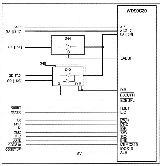
FIGURE 17, 16-BIT MICRO CHANNEL INTERFACE
