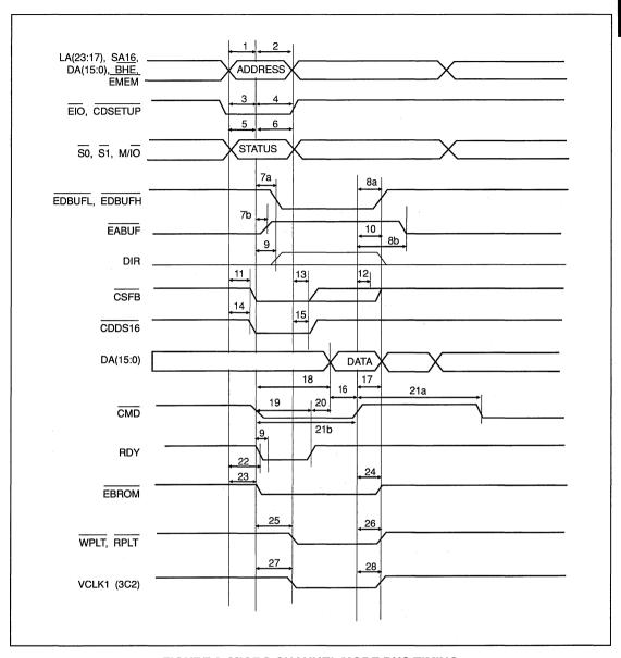
FIGURE 8. MICRO CHANNEL MODE BUS TIMING
