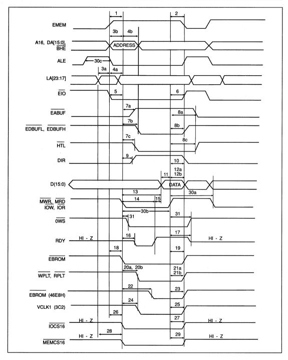
FIGURE 7. AT MODE BUS TIMING
