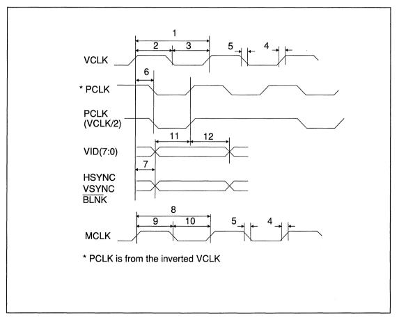
FIGURE 6. CLOCK AND VIDEO TIMING
