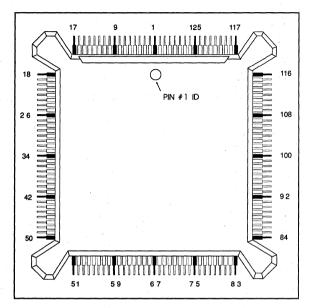
**FIGURE 3. 132-PIN JEDEC PACKAGE**
