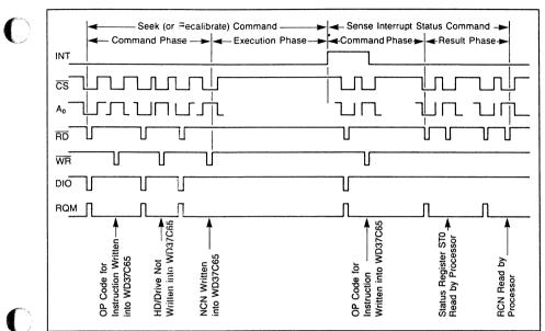
FIGURE 14. SEEK, RECALIBRATE AND SENSE INTERRUPT
