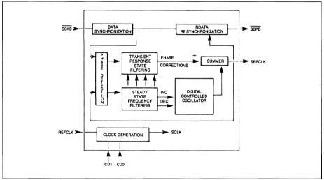
FIGURE 3. WD92C32 SIMPLIFIED BLOCK DIAGRAM
