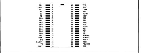
FIGURE 4. WD57C65 40-PIN DIP
