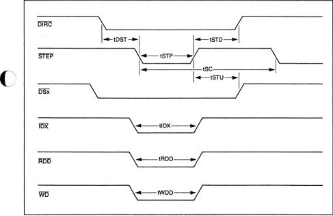
FIGURE 12. DISK DRIVE TIMING
