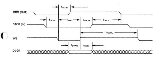
NOTE: External load on  $\overline{DRQ}$  &  $\overline{DACK}$  is assumed to be 1K $\Omega$ .
