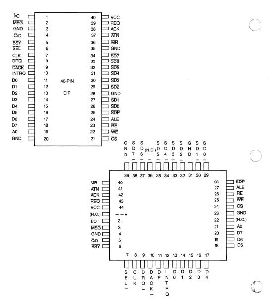
NOTE: Pin labeled N.C. should be left not connected.
