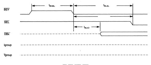
NOTE: Tgroup = signals driven by a Target =  $\overline{I/O}$ ,  $\overline{C/D}$ ,  $\overline{MSG}$ ,  $\overline{REQ}$  lgroup = signals driven by an Initiator =  $\overline{ATN}$ ,  $\overline{ACK}$
