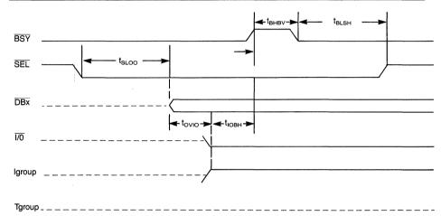
NOTE: Tgroup = signals driven by a Target =  $\overline{C/D}$ ,  $\overline{MSG}$ ,  $\overline{REQ}$ Igroup = signals driven by an Initiator =  $\overline{ATN}$ ,  $\overline{ACK}$
