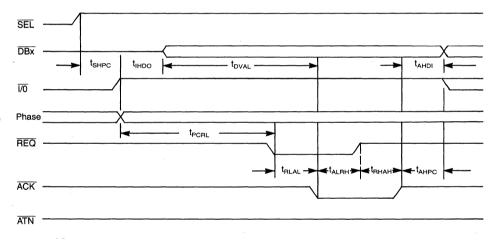
NOTE: Phase = signals that define the bus phase  $\overline{C/D}$ ,  $\overline{MSG}$
