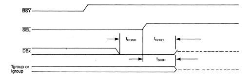
NOTE: Tgroup = signals driven by a Target =  $\overline{I/O}$ ,  $\overline{C/D}$ ,  $\overline{MSG}$ ,  $\overline{REQ}$  lgroup = signals driven by an Initiator =  $\overline{ATN}$ ,  $\overline{ACK}$
