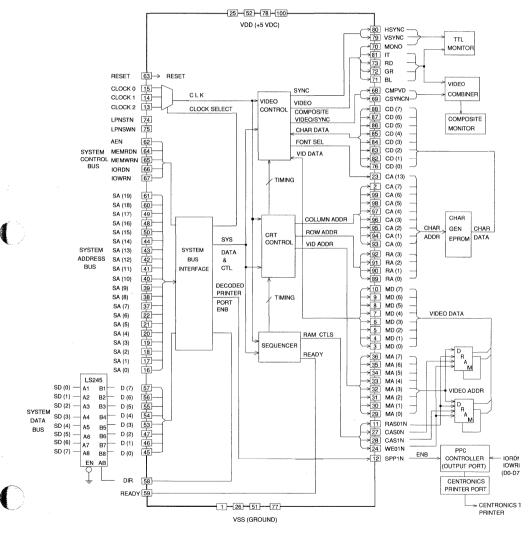
PVC4A FUNCTIONAL DIAGRAM (Pin numbers for the PLCC and JEDEC PFP)
