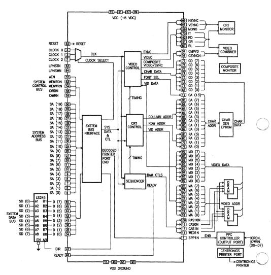
PVC4A FUNCTIONAL DIAGRAM (Pin numbers for the SHENKO package)
