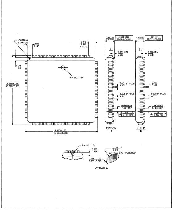
FIGURE 15-1. 84-PIN PLCC PACKAGE DIMENSIONS
