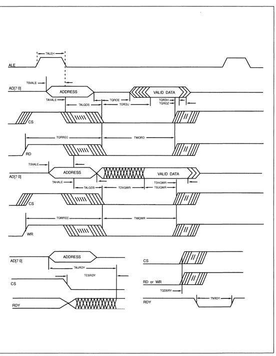
FIGURE 14-12. MICROPROCESSOR BUS TIMING
