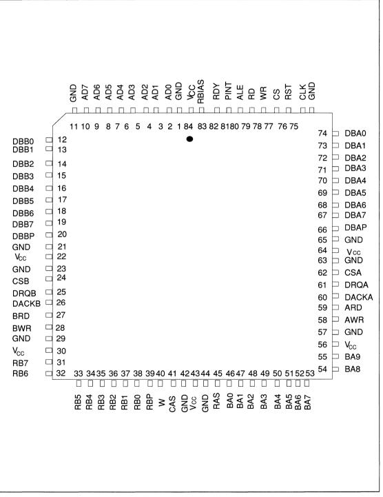
FIGURE 2-1. 84-PIN PLCC OR PQFP PIN ASSIGNMENTS
