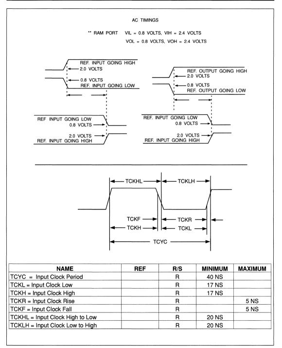
FIGURE 14-1. RISE/FALL AND MISC. TIMING
