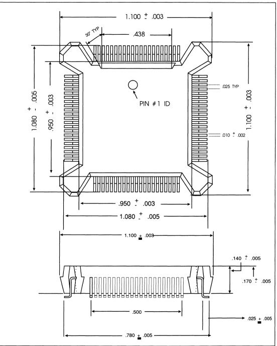
FIGURE 15-2. 84-PIN PQFP PACKAGE DIMENSIONS
