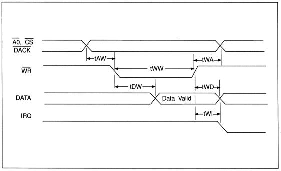
FIGURE 5-2. WRITE TIMING
