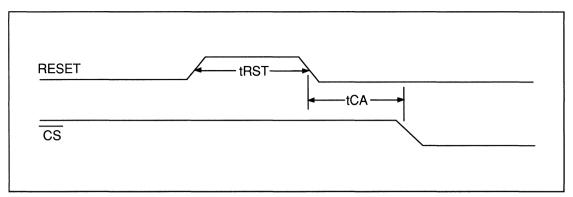
FIGURE 5-5. RESET TIMING
