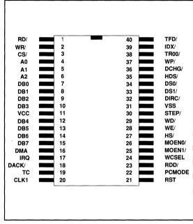
**FIGURE 3-2. WD57C65 40-PIN DIP**
