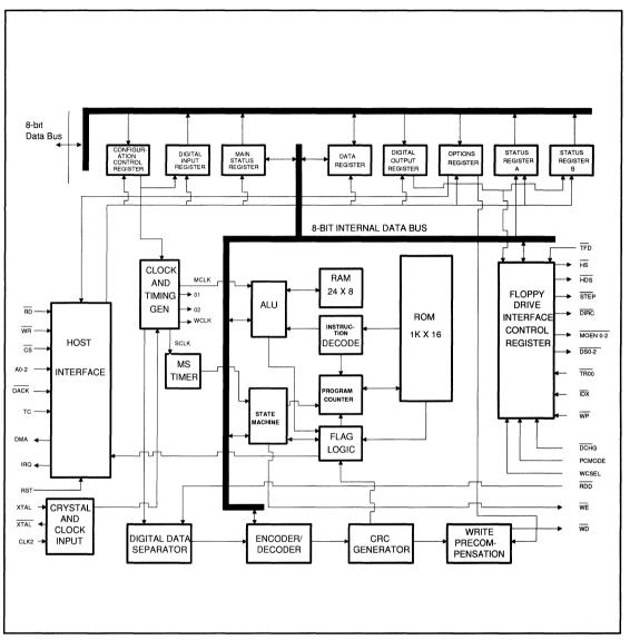
FIGURE 2-2. WD57C65 BLOCK DIAGRAM
