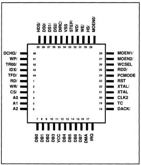
FIGURE 3-1. WD57C65 44-PIN PLCC
