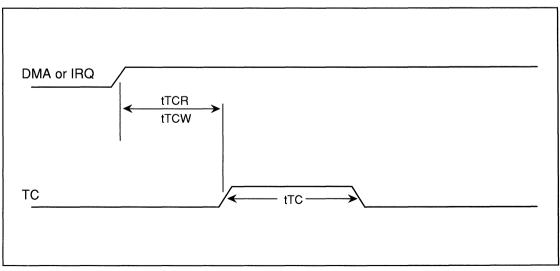
FIGURE 5-4. TERMINAL COUNT TIMING
