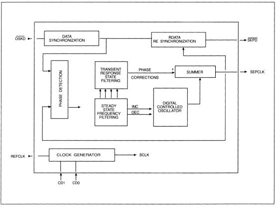
FIGURE 13-1. WD92C32 SIMPLIFIED BLOCK DIAGRAM
