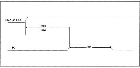
FIGURE 18-4. TERMINAL COUNT TIMING
