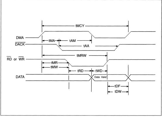
FIGURE 18-3. DMA TIMING
