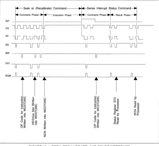
FIGURE 16-1. SEEK, RECALIBRATE, AND SENSE INTERRUPT
