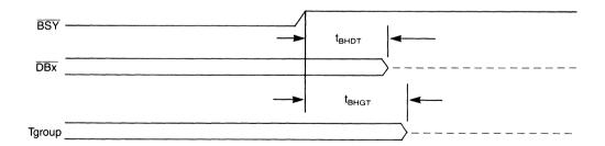
NOTE: Tgroup = signals driven by a Target =  $\overline{I/O}$ ,  $\overline{C/D}$ ,  $\overline{MSG}$ ,  $\overline{REQ}$
