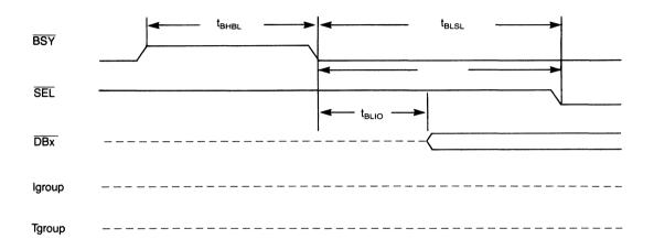
NOTE: Tgroup = signals driven by a Target =  $\overline{I/O}$ ,  $\overline{C/D}$ ,  $\overline{MSG}$ ,  $\overline{REQ}$  Igroup = signals driven by an Initiator =  $\overline{ATN}$ ,  $\overline{ACK}$
