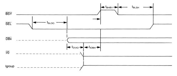
NOTE: Tgroup = signals driven by a Target =  $\overline{\text{C/D}}$ ,  $\overline{\text{MSG}}$ ,  $\overline{\text{REQ}}$  | Igroup = signals driven by an Initiator =  $\overline{\text{ATN}}$ ,  $\overline{\text{ACK}}$
