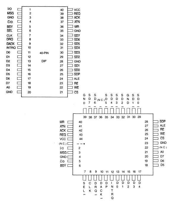
NOTE: Pin labeled N C. should be left not connected.
