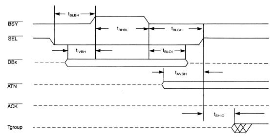
NOTE: Tgroup = signals driven by a Target =  $\overline{I/O}$ ,  $\overline{C/D}$ ,  $\overline{MSG}$ ,  $\overline{REQ}$
