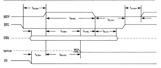
NOTE: Tgroup = signals driven by a Target =  $\overline{C/D}$ ,  $\overline{MSG}$ ,  $\overline{REQ}$  | Igroup = signals driven by an Initiator =  $\overline{ATN}$ ,  $\overline{ACK}$
