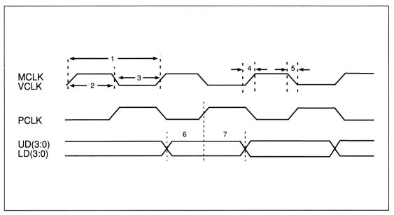
FIGURE C-14. CRT CLOCK TIMING
