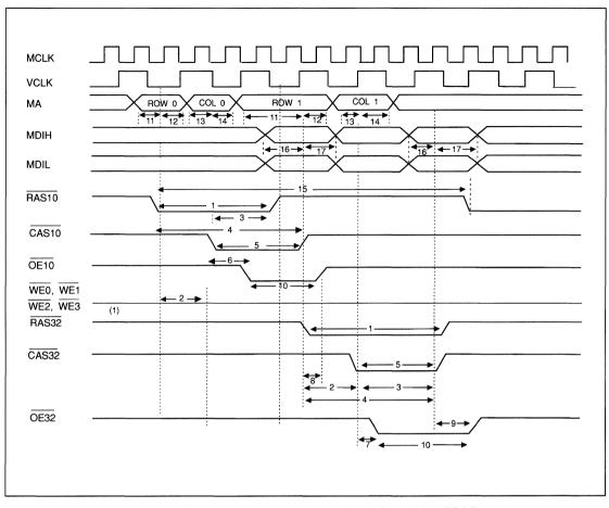
FIGURE C-10. CPU READ NON-PAGE MODE, CRT READ
