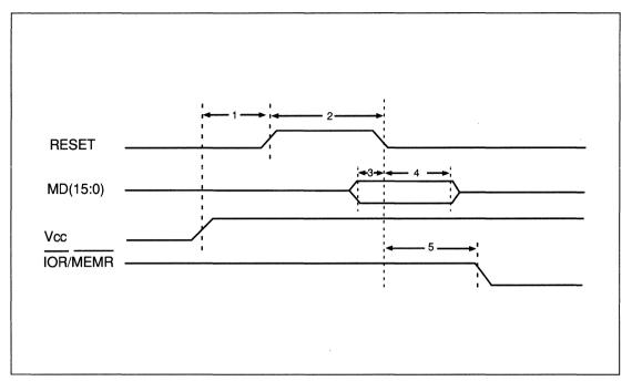
FIGURE C-15. RESET TIMING
