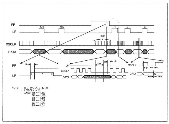
FIGURE C-19. STN COLOR LCD INTERFACE TIMING
