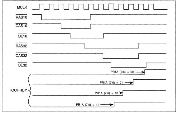
FIGURE C-20. IOCHRDY RELEASE TIMING IN MEMORY READ CYCLE
