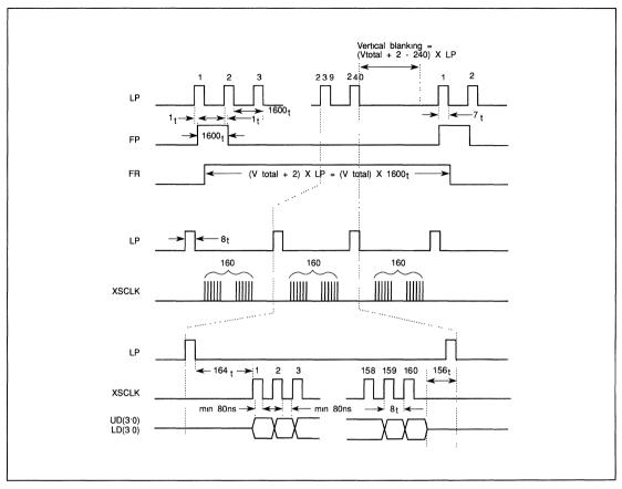
FIGURE C-12. WD90C22 LCD TIMING DIAGRAM (t=VCLK)
