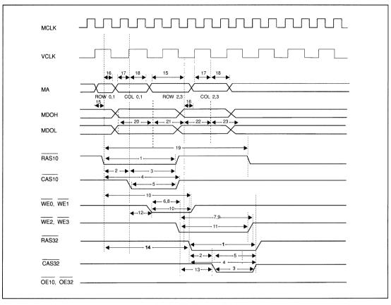
FIGURE C-9. CPU WRITE WITH NON-PAGE MODE
