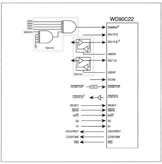
FIGURE A-2. MICRO CHANNEL INTERFACE
