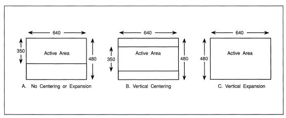
FIGURE 3-1. EXAMPLE OF SCREEN SIZE MAPPING
