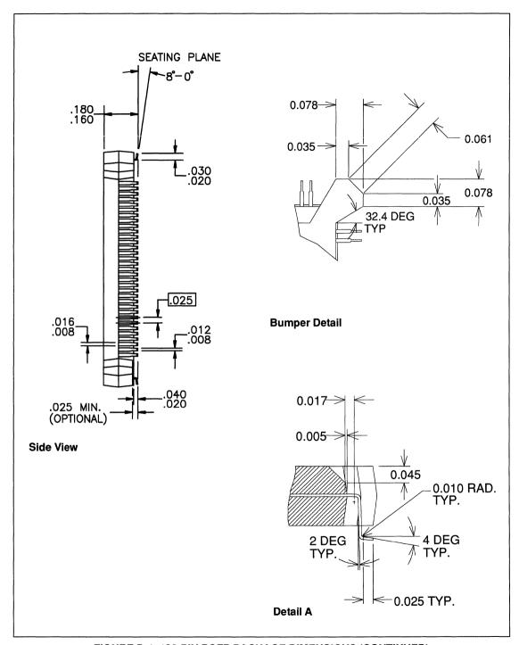
FIGURE D-1. 132-PIN PQFP PACKAGE DIMENSIONS (CONTINUED)
