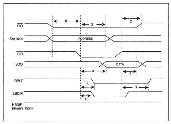
FIGURE C-2. I/O READ-AT MODE
