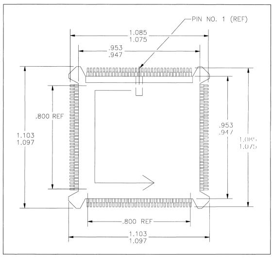
FIGURE D-1. 132-PIN PQFP PACKAGE DIMENSIONS
