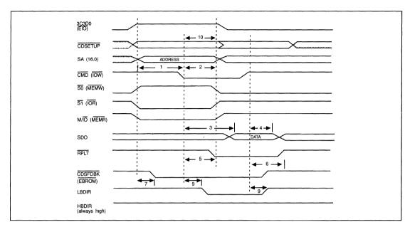
FIGURE C-6. I/O READ - MICRO CHANNEL MODE
