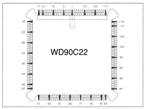
FIGURE 4-1. 132-PIN PQFP PIN ASSIGNMENTS
