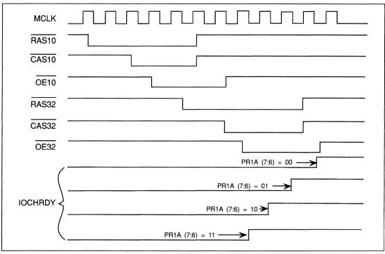
FIGURE C-20. IOCHRDY RELEASE TIMING IN MEMORY READ CYCLE
