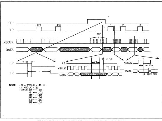
FIGURE C-19. STN COLOR LCD INTERFACE TIMING
