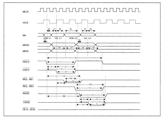
FIGURE C-9. CPU WRITE WITH NON-PAGE MODE
