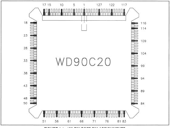
FIGURE 4-1. 132-PIN PQFP PIN ASSIGNMENTS
