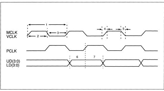
FIGURE C-14. CRT CLOCK TIMING
