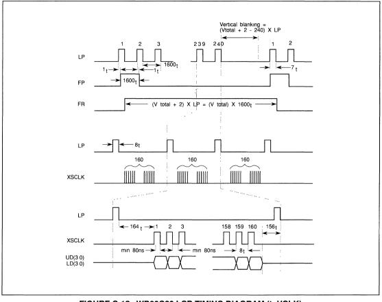
FIGURE C-12. WD90C20 LCD TIMING DIAGRAM (t=VCLK)
