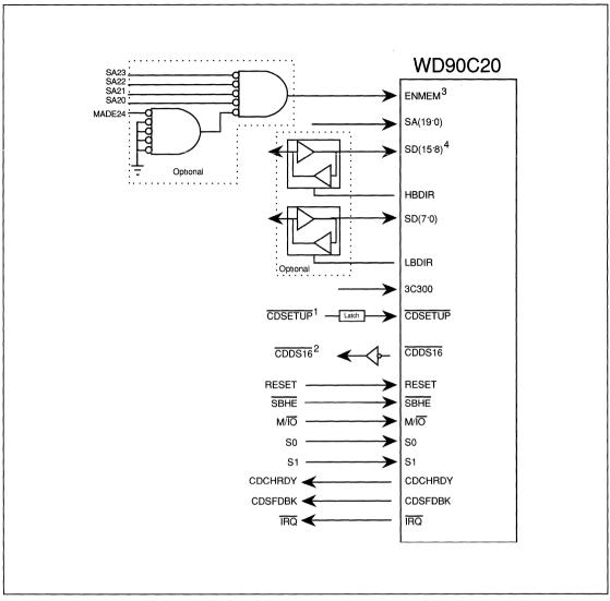
FIGURE A-2. MICRO CHANNEL INTERFACE
