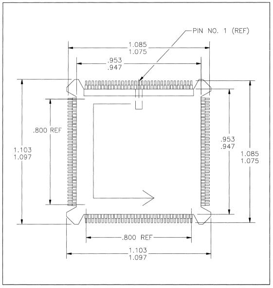
FIGURE D-1. 132-PIN PQFP PACKAGE DIMENSIONS
