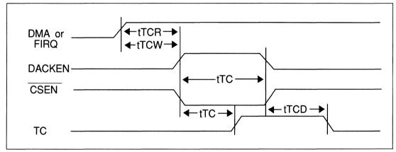
FIGURE 4-6. FDC TERMINAL COUNT TIMING DIAGRAM
