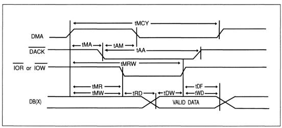
FIGURE 4-5. FDC DMA TIMING DIAGRAM
