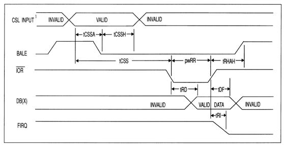
FIGURE 4-2. FDC READ W/BALE TIMING DIAGRAM
