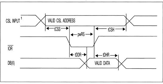
FIGURE 4-9. RTC AND RAM READ TIMING DIAGRAM
