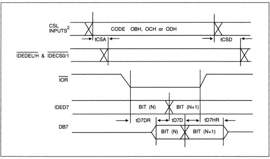
FIGURE 4-15. IDE INTERFACE TIMING DIAGRAM (IDED7 TO DB7)
