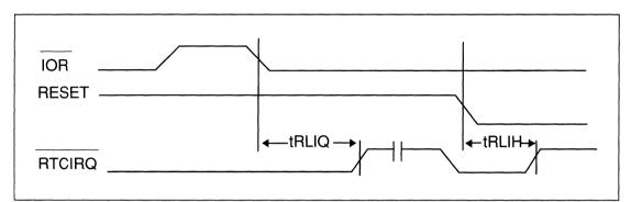
FIGURE 4-13. RTCIRQ RELEASE TIMING DIAGRAM
