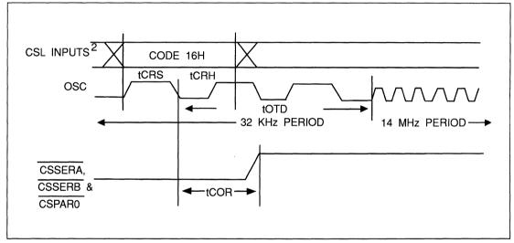
FIGURE 4-20. SUSPEND TO RESUME SUPPORT LOGIC
