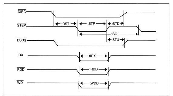
FIGURE 4-8. FDC DISK DRIVE TIMING DIAGRAM
