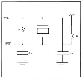
FIGURE 2-4. RTC CRYSTAL OSCILLATOR CONNECTIONS
