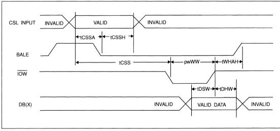
FIGURE 4-12. RTC AND RAM WRITE W/BALE TIMING DIAGRAM
