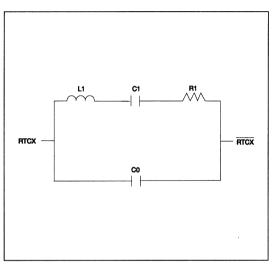
FIGURE 2-5. RTC CRYSTAL PARAMETERS
