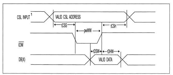
FIGURE 4-11. RTC AND RAM WRITE TIMING DIAGRAM
