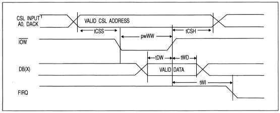
FIGURE 4-3. FDC WRITE TIMING DIAGRAM
