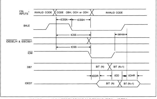
FIGURE 4-18. IDE INTERFACE W/BALE TIMING (DB7 to IDED7)
