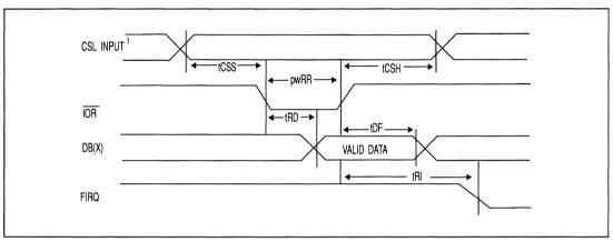
FIGURE 4-1. FDC READ TIMING DIAGRAM
