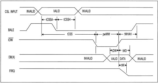
FIGURE 4-4. FDC WRITE W/BALE TIMING DIAGRAM
