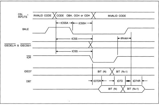
FIGURE 4-16. IDE INTERFACE W/BALE TIMING (IDED7 to DB7)
