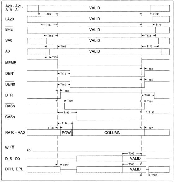
FIGURE 11-47. AT BUS MASTER, READ FROM ON-BOARD MEMORY
