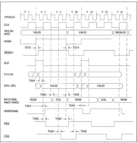
FIGURE 11-19. 80386SX - NON-PAGE MODE 00, 1 WAIT STATE WRITE (PIPELINE) (4072H = 0001)
