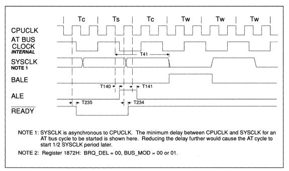
FIGURE 11-33. 80286 CPU - ASYNCHRONOUS CPUCLK TO SYSCLK, BREQ DELAY = 1 CLOCK
