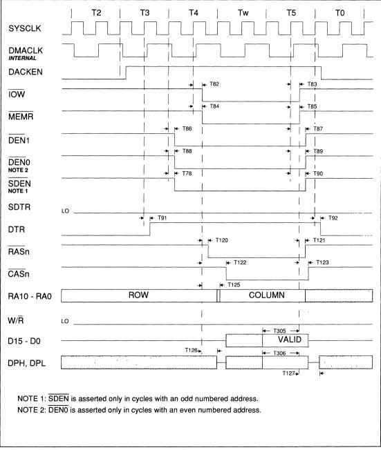
FIGURE 11-44. DMA CYCLE, ON-BOARD MEMORY TO 8-BIT I/O
