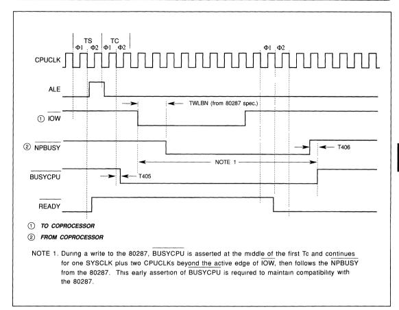
FIGURE 11-52. 80286 - BUSYCPU ASSERTED DURING COPROCESSOR ACCESS
