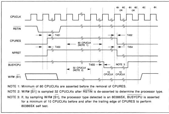
FIGURE 11-55. 80386SX - CPURES AND NPRST DURING POWER UP
