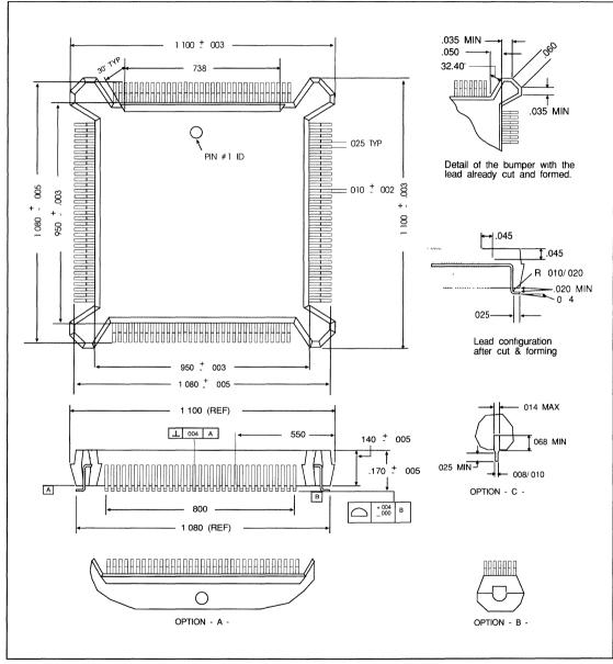
FIGURE 13-1. 132-PIN PQFP PACKAGE
