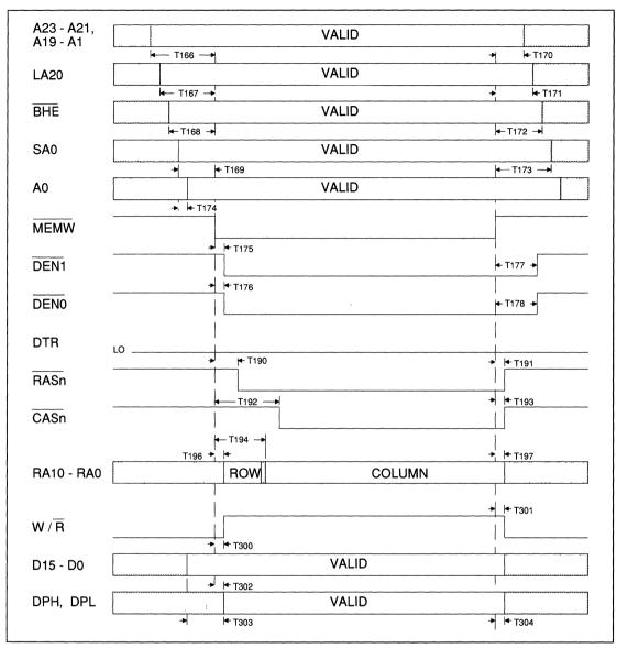
FIGURE 11-46. AT BUS MASTER, WRITE TO ON-BOARD MEMORY
