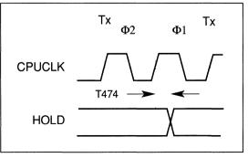
FIGURE 11-62. 80386SX - OUTPUT DELAY TIMING
