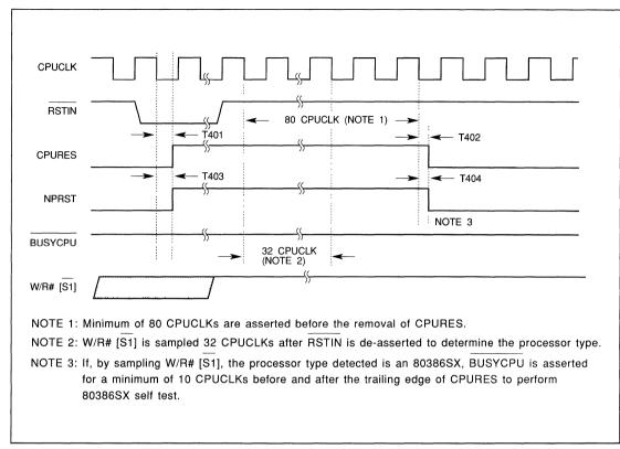
FIGURE 11-49. 80286 - CPURES AND NPRST DURING POWER UP
