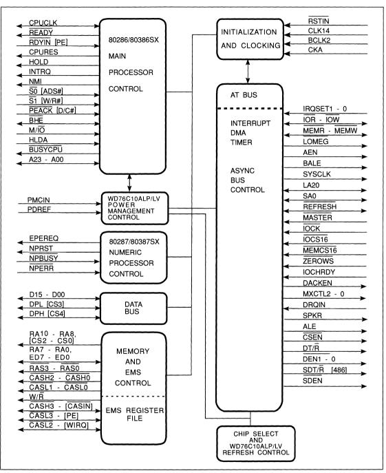
FIGURE 2-1. WD76C10A/LP/LV BLOCK DIAGRAM
