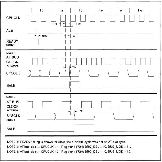
FIGURE 11-34. 80286 CPU - SYCNHRONOUS CPUCLK TO SYSCLK
