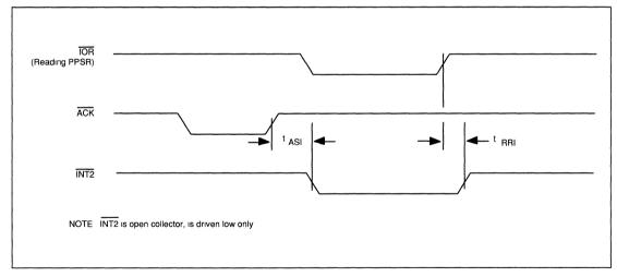
FIGURE 6-14. WD16C552 PARALLEL PORT INTERRUPT TIMING
