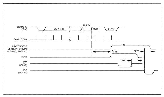
FIGURE 6-6. RCVR FIFO SIGNALING TIMING FOR FIRST BYTE
