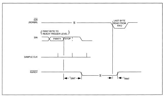
FIGURE 6-9. RECEIVER DMA MODE 1 TIMING (FCR0=1 AND FCR3=1)
