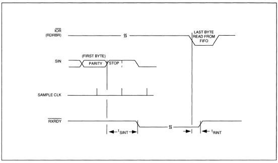
FIG. 6-8. RECEIVER DMA MODE 0 TIMING (FCR0=0 OR FCR0=1 AND FCR3=0)
