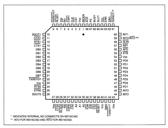
FIGURE 2-1. 68-PIN PLCC PIN ASSIGNMENTS
