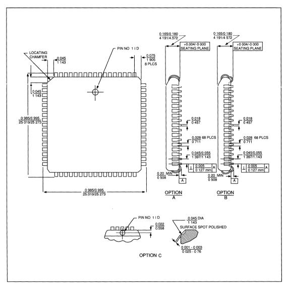
FIGURE 7-1. 68-PIN PLCC PACKAGE DIMENSIONS
