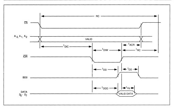
FIGURE 6-4. READ CYCLE TIMING
