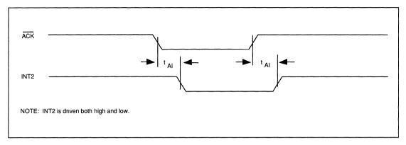
FIGURE 6-13. WD16C452 PARALLEL PORT INTERRUPT TIMING
