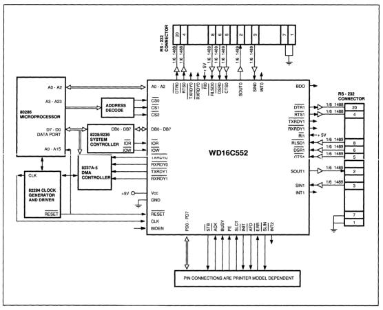
FIGURE 5-2. TYPICAL 16-BIT MICROPROCESSOR/RS-232 TERMINAL INTERFACE USING THE WD16C552
