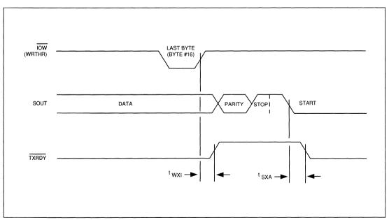
FIGURE 6-11. TRANSMITTER DMA MODE 1 (FCR0 = 1 and FCR3 = 1)
