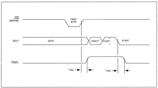
FIGURE 6-10. TRANSMITTER DMA MODE 0 TIMING (FCR0 = 0 or FCR0 = 1 and FCR3 = 0)
