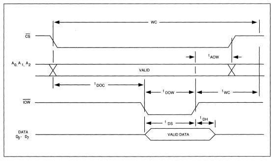
FIGURE 6-5. WRITE CYCLE TIMING
