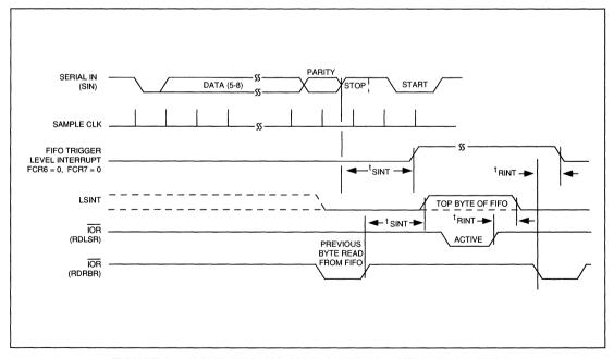
FIGURE 6-7. RCVR FIFO SIGNALING TIMING AFTER FIRST BYTE (RBR Already Set)
