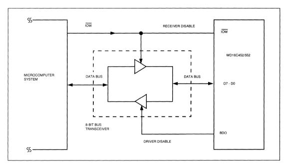
FIGURE 5-1. TYPICAL INTERFACE FOR A HIGH-CAPACITY DATA BUS
