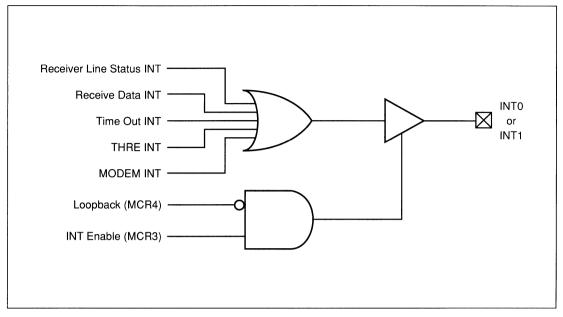
FIGURE 3-1. INTERRUPT SIGNAL LOGIC
