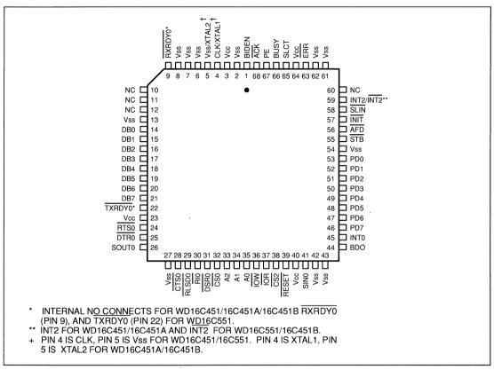
FIGURE 2-1. 68-PIN PLCC PIN ASSIGNMENTS
