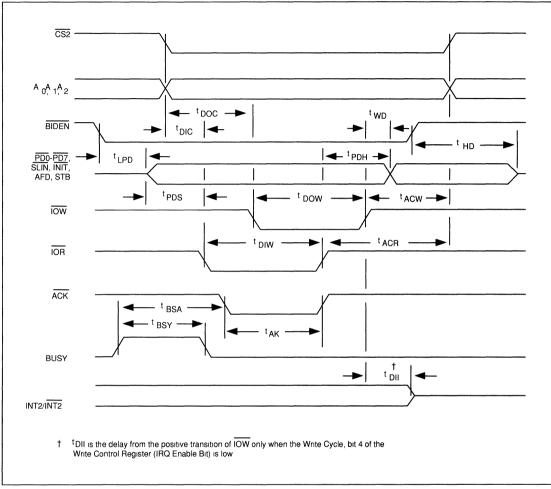
FIGURE 7-12. PARALLEL PORT TIMING
