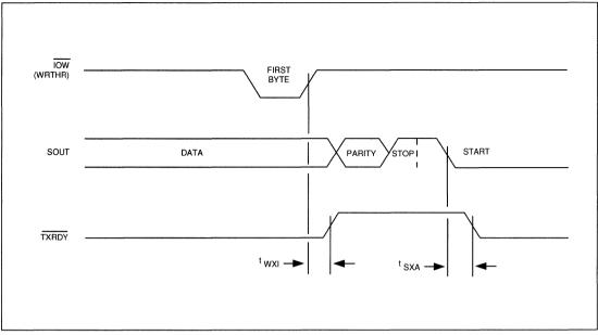
FIGURE 7-10. TRANSMITTER DMA MODE 0 TIMING (FCR0 = 0 or FCR0 = 1 and FCR3 = 0)
