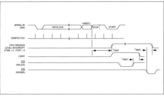
FIGURE 7-6. RCVR FIFO SIGNALING TIMING FOR FIRST BYTE
