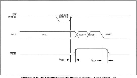
FIGURE 7-11. TRANSMITTER DMA MODE 1 (FCR0 = 1 and FCR3 = 1)
