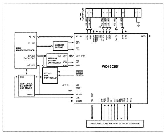
FIGURE 5-2. TYPICAL 16-BIT MICROPROCESSOR/RS-232 TERMINAL INTERFACE USING THE WD16C551
