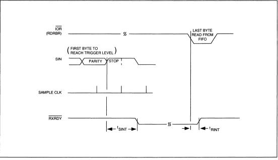
FIGURE 7-9. RECEIVER DMA MODE 1 TIMING (FCR0=1 and FCR3=1)
