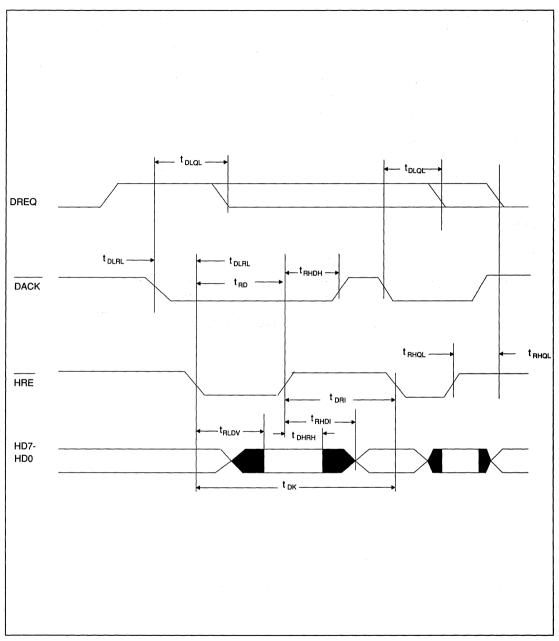
FIGURE 11. AT/XT HOST DMA READ TIMING
