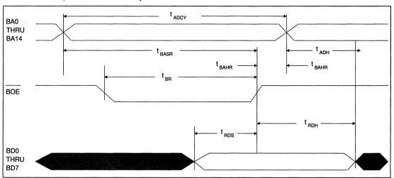
FIGURE 19. BUFFER RAM READ TIMING (EXTERNAL OSCILLATOR)
