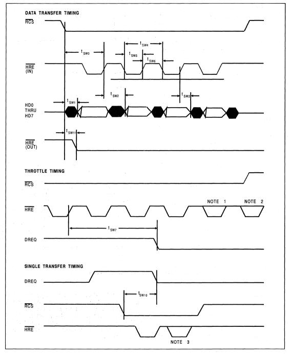
FIGURE 15. SLAVE HOST DMA READ TIMING
