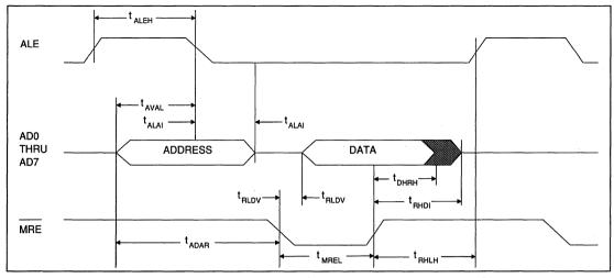
FIGURE 22. MICROPROCESSOR READ TIMING (INTEL BUS)
