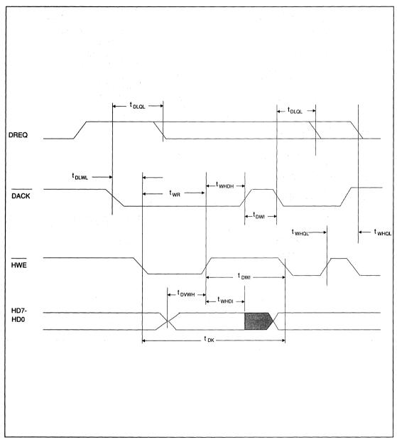
FIGURE 10. AT/XT HOST DMA WRITE TIMING
