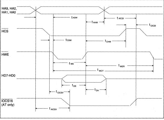
FIGURE 7. AT/XT HOST PROGRAMMED I/O WRITE TIMING
