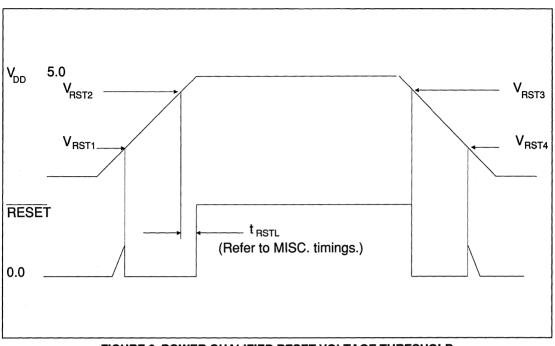
FIGURE 6. POWER QUALIFIED RESET VOLTAGE THRESHOLD
