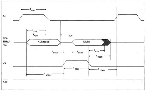
FIGURE 23. MICROPROCESSOR READ TIMING (MOTOROLA BUS)
