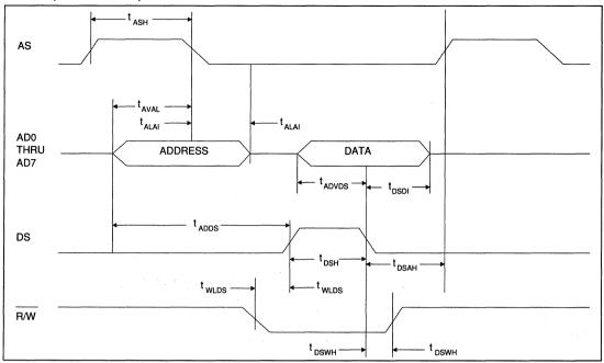
FIGURE 21. MICROPROCESSOR WRITE TIMING (MOTOROLA BUS)
