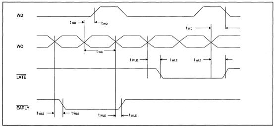
FIGURE 24. WRITE DATA TIMING (MFM/RLL MODE)
