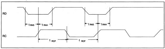
FIGURE 27. READ DATA TIMING (NRZ MODE)
