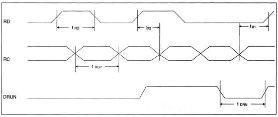
FIGURE 26. READ DATA TIMING (MFM/RLL)
