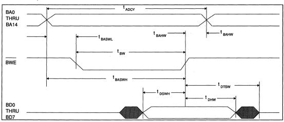
FIGURE 16. BUFFER RAM WRITE TIMING (INTERNAL OSCILLATOR)
