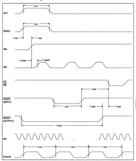
FIGURE 28. MISCELLANEOUS TIMING
