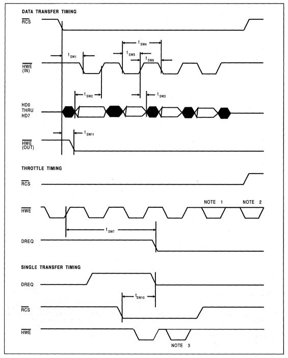
FIGURE 14. SLAVE HOST DMA WRITE TIMING
