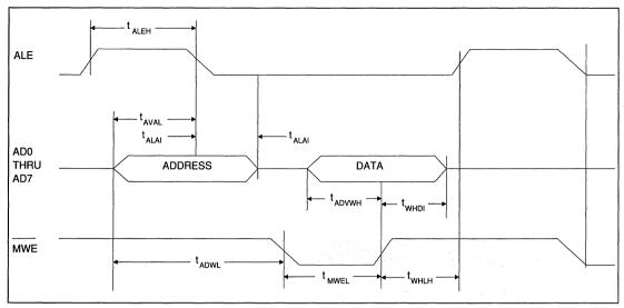
FIGURE 20. MICROPROCESSOR WRITE TIMING (INTEL BUS)
