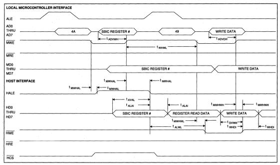
FIGURE 12. SLAVE HOST WRITE TIMING
