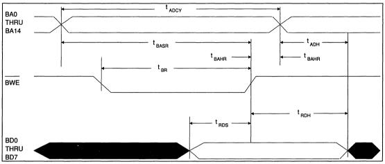
FIGURE 17. BUFFER READ TIMING (INTERNAL OSCILLATOR)
