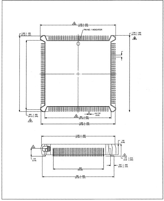
FIGURE 36. 84 LEAD PQFP
