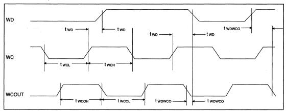
FIGURE 25. WRITE DATA TIMING (NRZ MODE)
