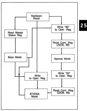
FIGURE 9-1. FLOW DIAGRAM BASE, SPECIAL & AT/EISA MODES
