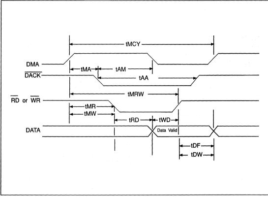
FIGURE 18-3. DMA TIMING
