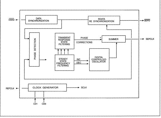
FIGURE 13-1. WD92C32 SIMPLIFIED BLOCK DIAGRAM
