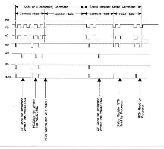
FIGURE 16-1. SEEK, RECALIBRATE, AND SENSE INTERRUPT
