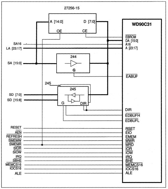
FIGURE 12-3. 16-BIT PC AT INTERFACE WITH 8-BIT BIOS
