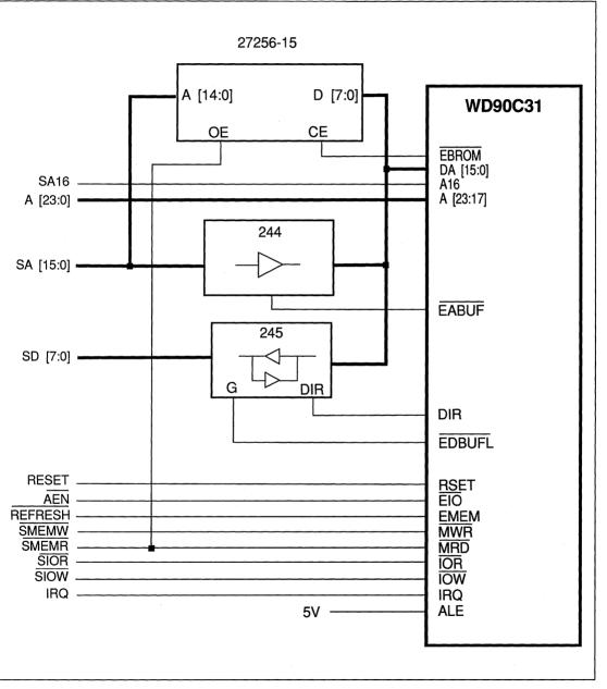
FIGURE 12-2. 8-BIT PC AT INTERFACE WITH 8-BIT BIOS
