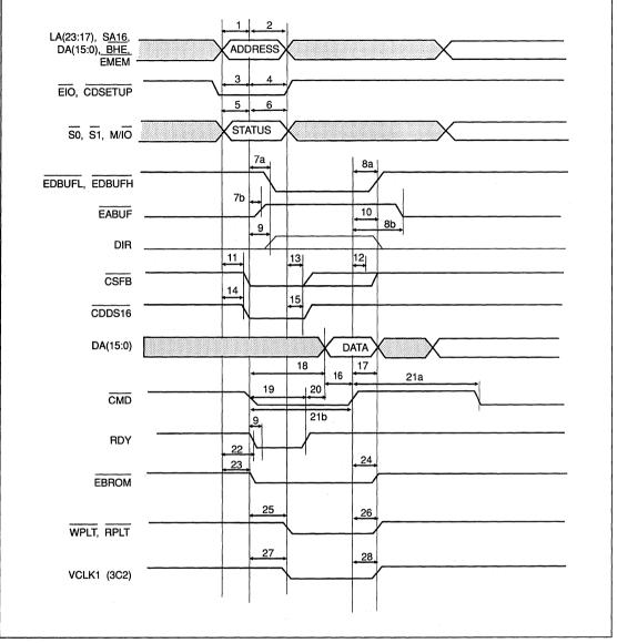
FIGURE 6-4. MICRO CHANNEL MODE BUS TIMING
