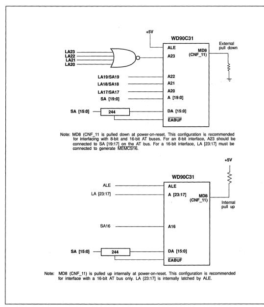
FIGURE 12-6. WD90C31 INTERFACE FOR 286 OR 386-BASED SYSTEMS
