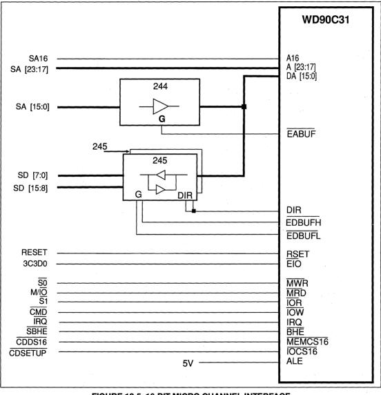
FIGURE 12-5. 16-BIT MICRO CHANNEL INTERFACE
