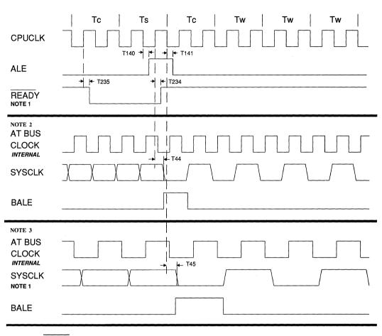
NOTE 1: READY timing is shown for when the previous cycle was not an AT bus cycle. NOTE 2: AT bus clock = CPUCLK + 1. Register 1872H: BRQ\_DEL = 10, BUS\_MOD = 11. NOTE 3: AT bus clock = CPUCLK + 2. Register 1872H: BRQ\_DEL = 10, BUS\_MOD = 10.
