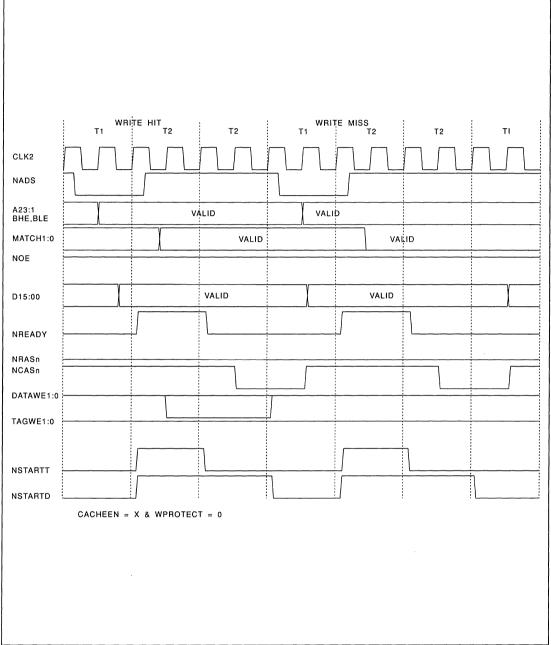
FIGURE 13-64. WRITE HIT/WRITE MISS CYCLE
