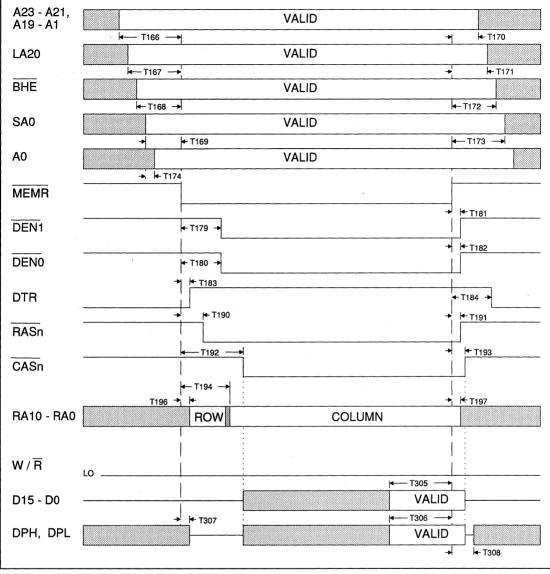
FIGURE 13-47. AT BUS MASTER, READ FROM ON-BOARD MEMORY
