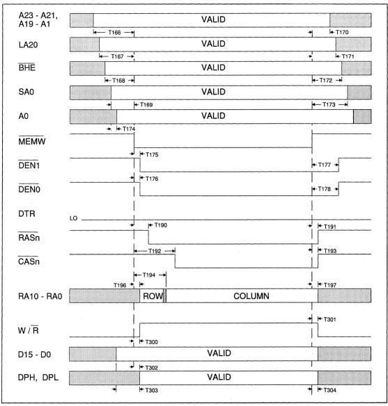
FIGURE 13-46. AT BUS MASTER, WRITE TO ON-BOARD MEMORY
