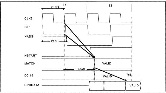
FIGURE 13-67. TAG RAM AND DATA RAM TIMING
