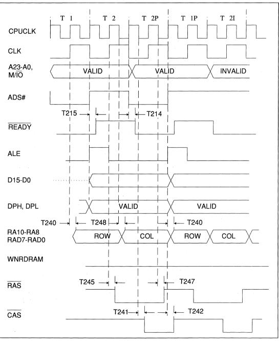
FIGURE 13-20. 80386SX - NON-PAGE MODE 01, 0 WAIT STATE READ (PIPELINE) (4072H = 3560H)
