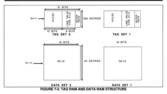
During the read block miss cycle, the address is written into the TAG RAM, the block valid bit is set, and the corresponding line valid bit is set.
