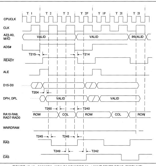
FIGURE 13-18. 80386SX - NON-PAGE MODE 00, 1 WAIT STATE READ (PIPELINE) (4072H = 0001)
