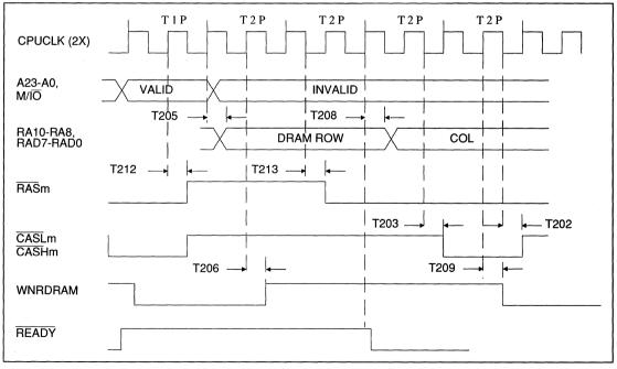
FIGURE 13-17. 80386SX - PAGE MODE, WRITE MISS CYCLE FOLLOWING A WRITE CYCLE
