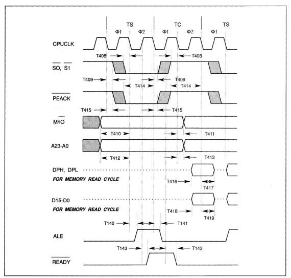
FIGURE 13-54. 80286 - MISCELLANEOUS TIMING
