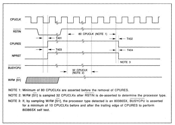
FIGURE 13-49. 80286 - CPURES AND NPRST DURING POWER UP
