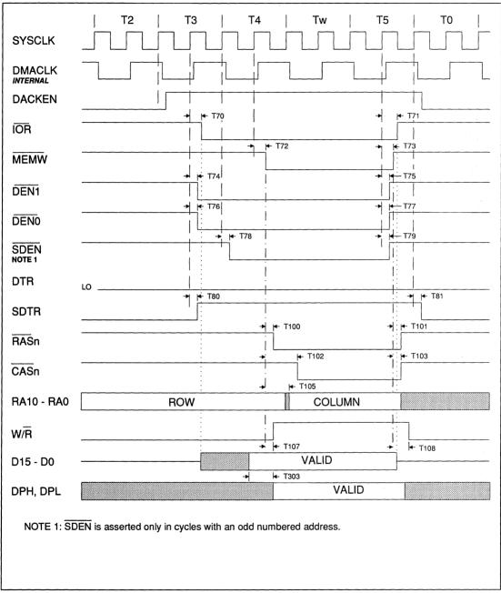
FIGURE 13-43. DMA CYCLE, 8-BIT I/O TO ON-BOARD MEMORY
