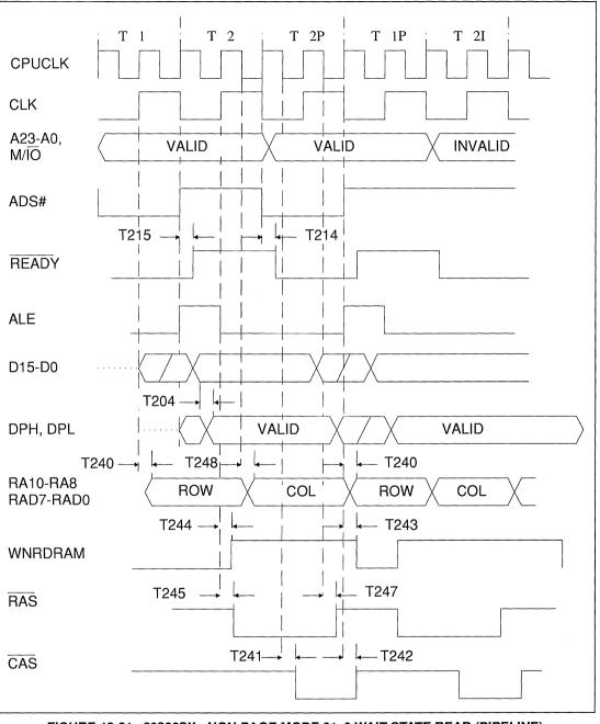
FIGURE 13-21. 80386SX - NON-PAGE MODE 01, 0 WAIT STATE READ (PIPELINE) (4072H = 3560H)
