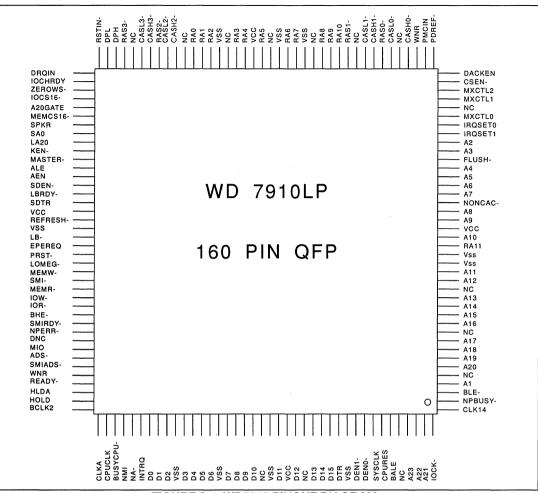
FIGURE 3-1. WD7910 PINOUT DIAGRAM
