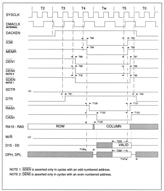
FIGURE 13-44. DMA CYCLE, ON-BOARD MEMORY TO 8-BIT I/O
