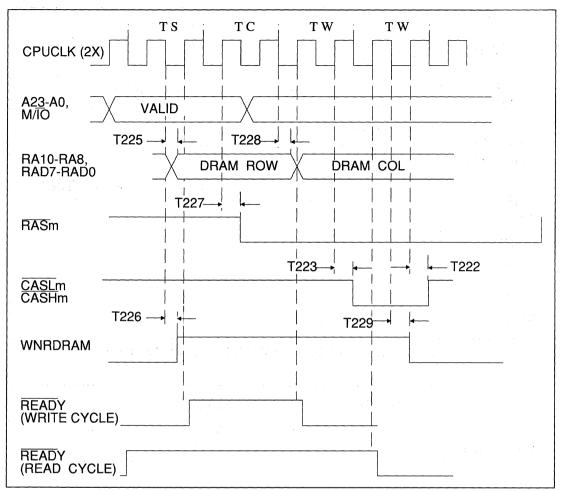
FIGURE 13-1. 80286 - PAGE MODE FIRST ACCESS READ/WRITE
