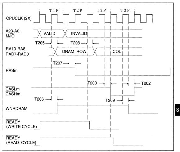
FIGURE 13-12. 80386SX - PAGE MODE, FIRST ACCESS READ/WRITE
