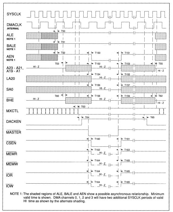
FIGURE 13-45. AT BUS MASTER, BUS ACQUISITION/RELEASE
