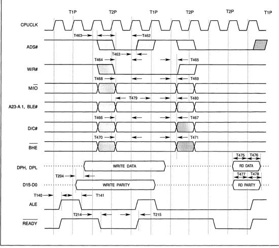
FIGURE 13-60. 80386SX - MISCELLANEOUS TIMING
