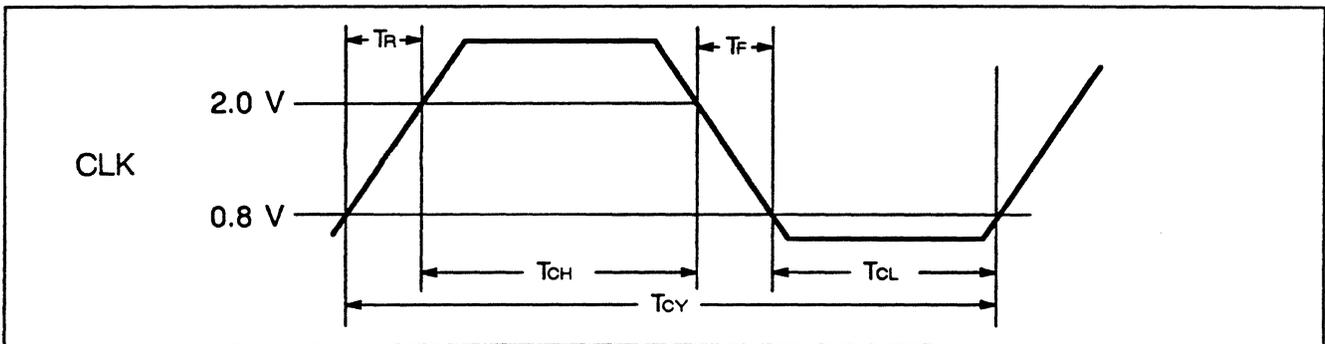
Figure 12. CLK Waveform diagram
