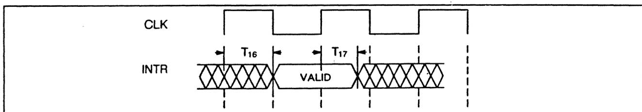
Figure 19. Interrupt timing
