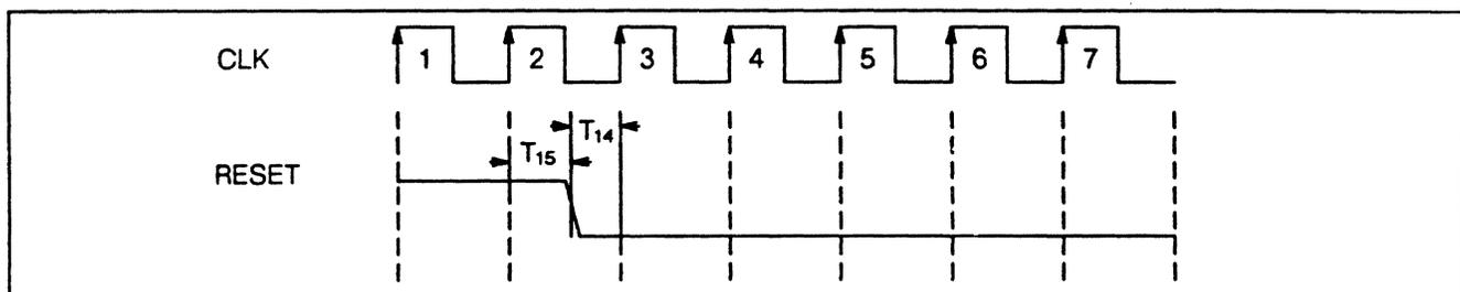
Figure 18. RESET timing
