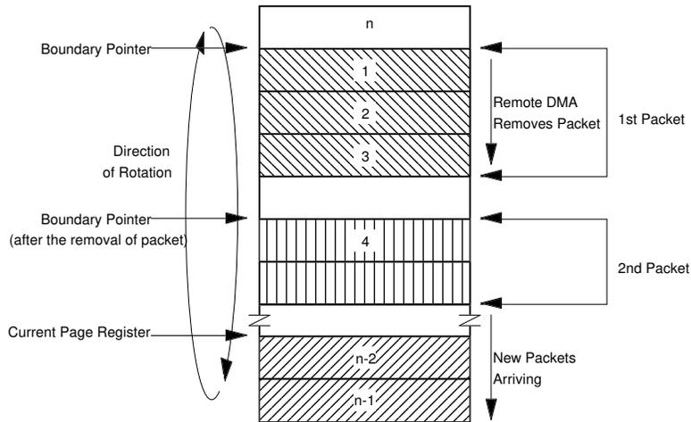
**Figure 10. Removing Packets from the Receive Buffer Ring**
