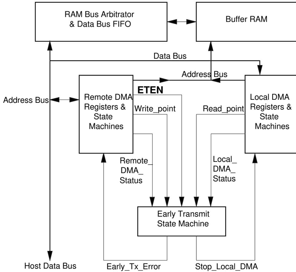
**Figure 13: Early Transmit Error Detect Block Diagram**
