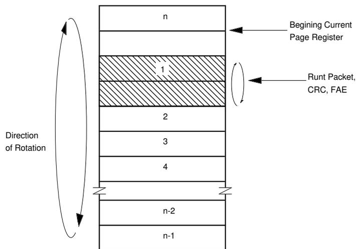
**Figure 9. Packet Rejection**
