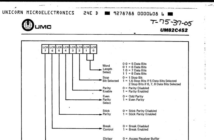
Figure 1. Line Control Register
