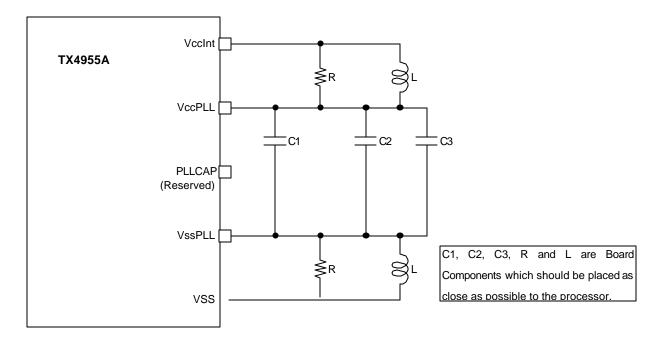
Figure 1 PLL Recommended Circuit
