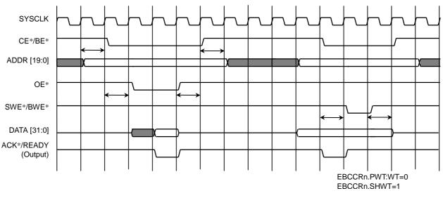
Figure 7.3.6 SHWT 1 Wait (Normal Mode, Single Read/Write Cycle)
