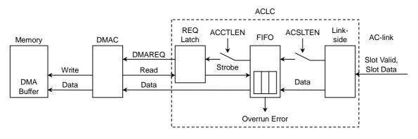
Figure 14.3.7 Sample-data Reception Mechanism
