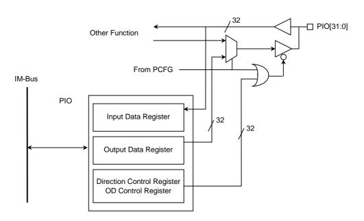
Figure 13.2.1 Parallel I/O Block Diagram
