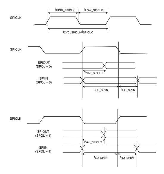
Figure 22.5.16 Timing Diagrams: SPI Interface
