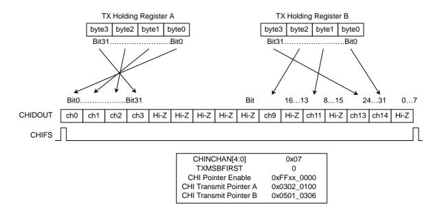
Figure 16.3.1 Transmit TDM Switch Example
