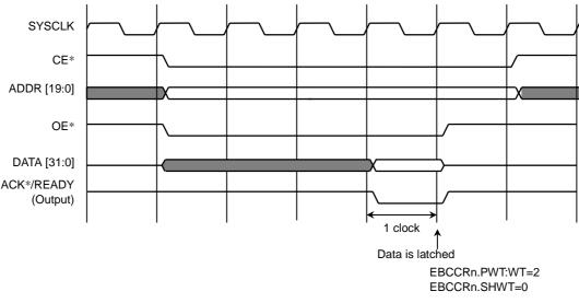
Figure 7.3.7 ACK\* Output Timing (Single Read Cycle)
