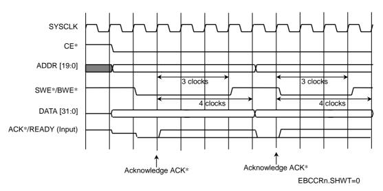
Figure 7.3.13 ACK\* Input Timing (Burst Write Cycle)
