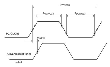
Figure 22.5.7 Timing Diagrams: PCI Clock Skew
