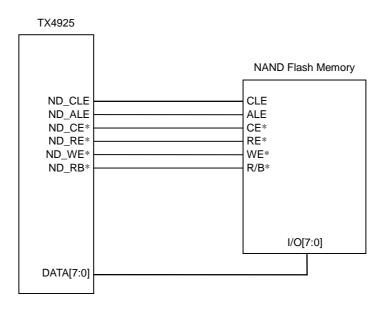
Figure 18.6.1 Example of Using NAND Flash Memory
