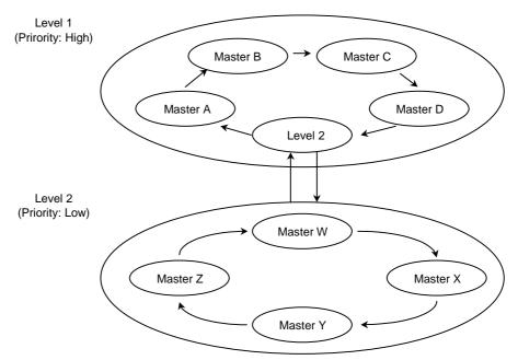
Figure 10.3.9 PCI Bus Arbitration Priority
