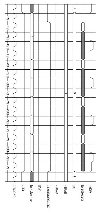
Figure 7.5.26 4-word Burst Read (0 Wait, SHWT=0, External ACK\*, 32-bit Bus)
