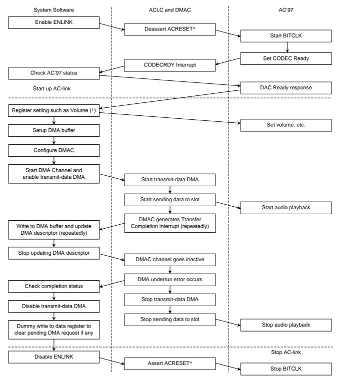
(\*) Register settings such as volume can be made during data playback.
