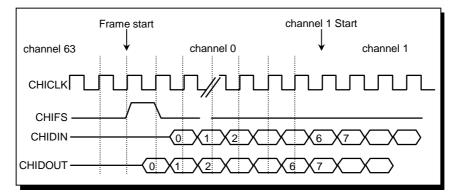
Figure 16.3.7 CHI Frame Structure Example
