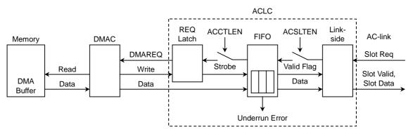
Figure 14.3.6 Sample-data Transmission Mechanism
