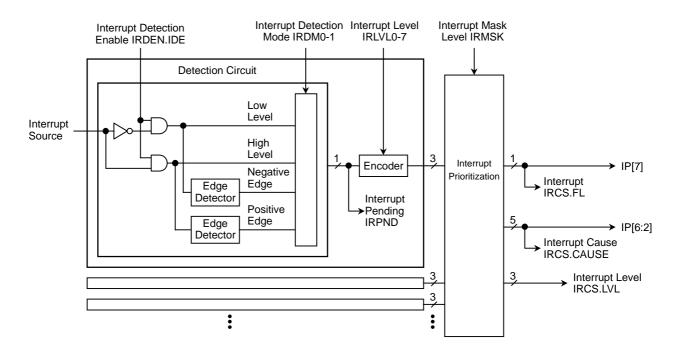
Figure 15.2.2 Internal Block Diagram of Interrupt Controller
