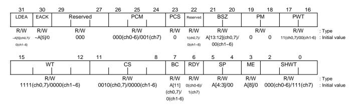
Only in the case of Channel 0 is fields with different defaults in the "Channel 0/Other channel" state. D[] represents the corresponding Data[] signal value when the RESET\* signal is deasserted. A[] represents the corresponding ADDR[] signal value when the RESET\* signal is deasserted.
