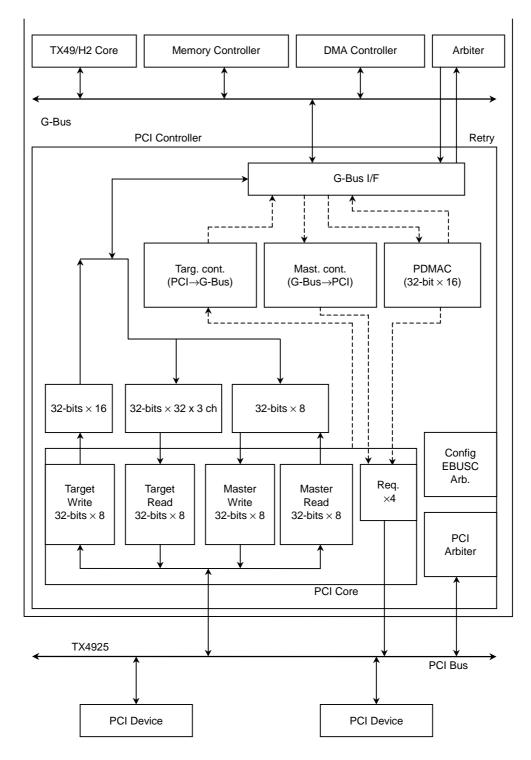
Figure 10.2.1 PCI Controller Block Diagram
