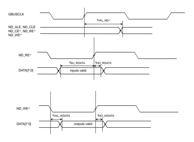
Figure 22.5.14 Timing Diagrams: NAND Flash Memory Interface
