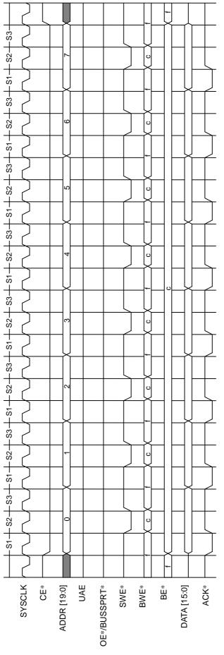
Figure 7.5.14 4-word Burst Write (PWT: WT=0, SHWT=0, Normal, 16-bit Bus)
