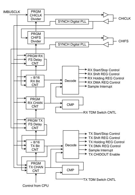
Figure 16.3.2 CHI Clock and Control Generation
