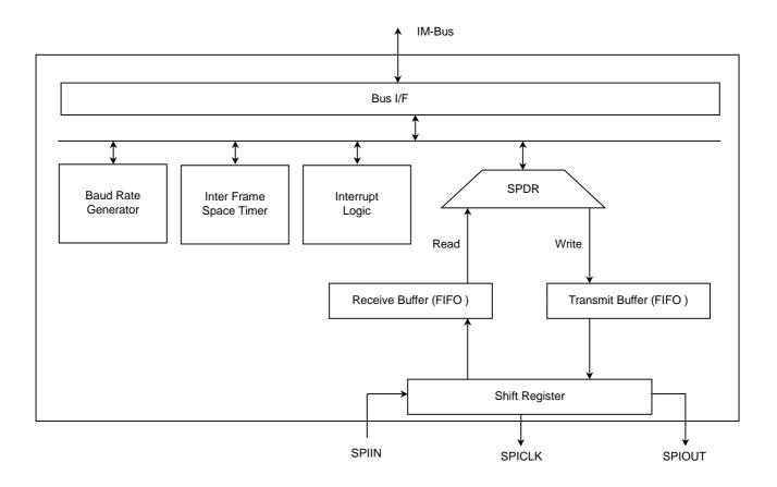
Figure 17.2.1 SPI Block Diagram
