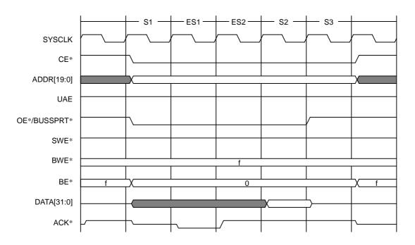
Figure 7.5.23 1-word Single Write (0 Wait, SHWT=0, External ACK\*, 32-bit Bus)
