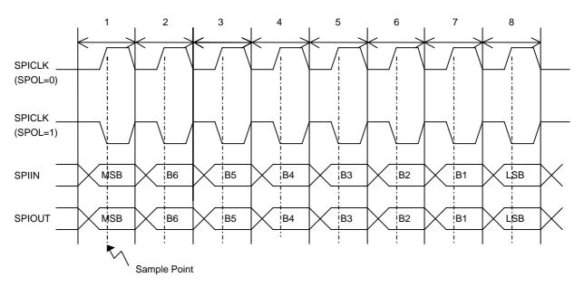
Figure 17.3.1 shows the transfer format for a SPHA=0 transfer.
