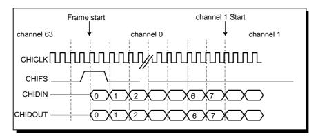
Figure 16.3.10 CHI Frame Structure Example
