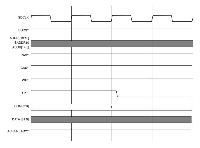
Figure 9.5.13 Transition to Power Down Mode
