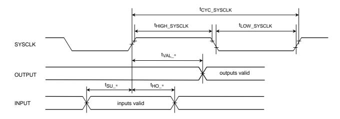
Figure 22.5.5 Timing Diagrams: External Bus Interface
