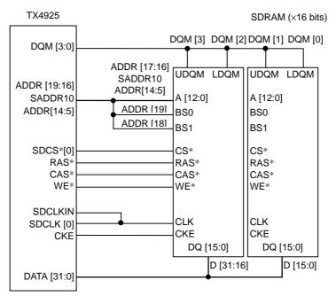
Figure 9.6.1 SDRAM (×16 bits) Connection Example
