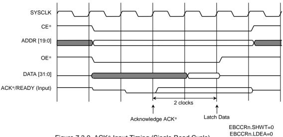
Figure 7.3.9 ACK\* Input Timing (Single Read Cycle)
