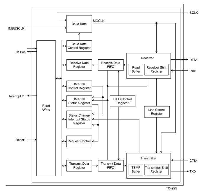
Figure 11.2.1 SIO Internal Block Diagram
