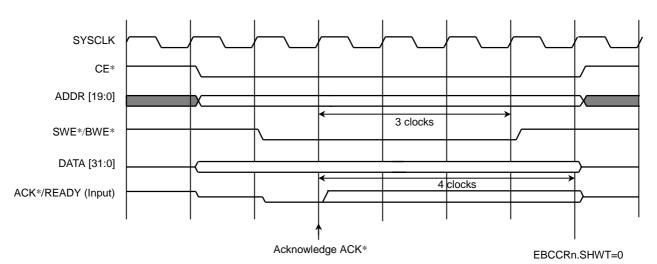
Figure 7.3.11 ACK\* Input Timing (Single Write Cycle)
