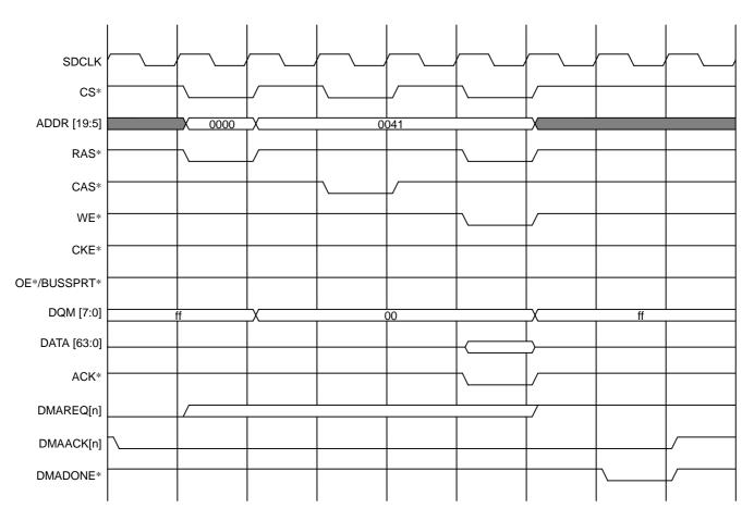
Figure 8.5.13 Single Address Single Transfer from Memory to I/O (Single Read of 64-bit Data from 64-bit SDRAM)
