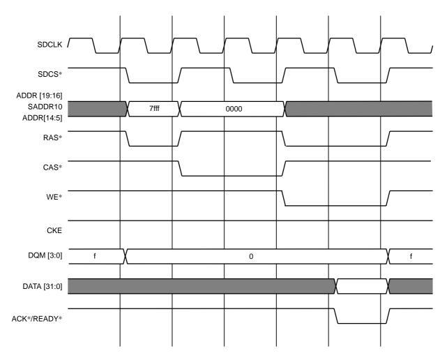
Figure 9.5.1 Single Read ( $t_{RCD} = 2$ ,  $t_{CASL} = 2$ ,  $t_{DA} = 0$ , 32-bit Bus)
