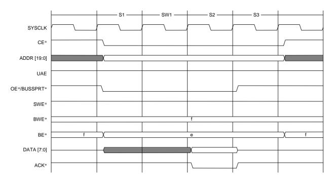
Figure 7.5.18 1-byte Single Read (PWT: WT=1, SHWT=0, Normal, 8-bit Bus)
