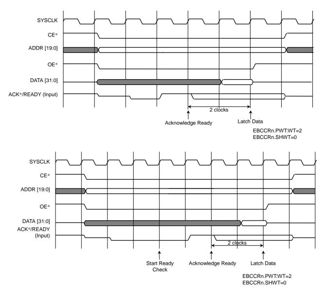
Figure 7.3.14 Ready Input Timing (Read Cycle)
