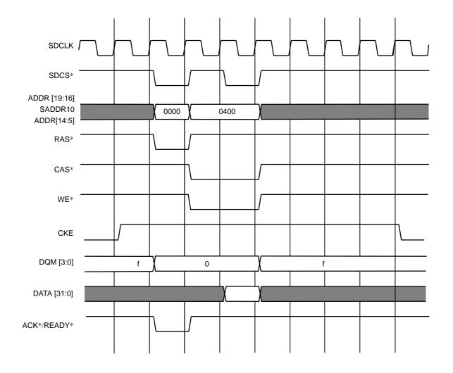
Figure 9.5.15 Power Down Auto Entry (SDCTR.PDAE=1, SDCTR.ACE=0)
