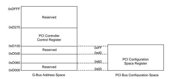
Figure 10.3.2 Register Map in the Satellite Mode
