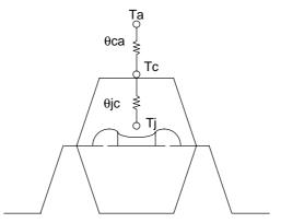
Figure 2 Thermal resistance of package
