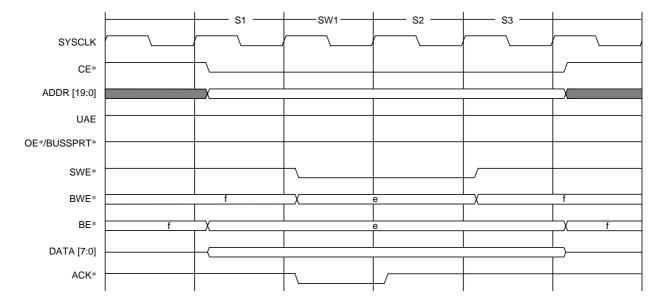
Figure 7.5.17 1-byte Single Write (PWT: WT=1, SHWT=0, Normal, 8-bit Bus)
