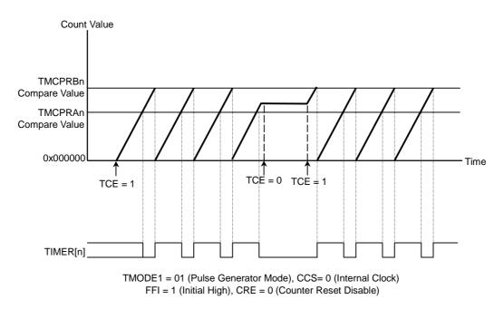
Figure 12.3.3 Operation Example of the Pulse Generator Mode
