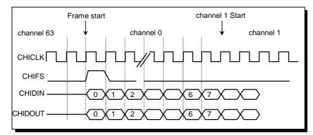
Figure 16.3.5 CHI Frame Structure Example
