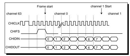
Figure 16.3.9 CHI Frame Structure Example
