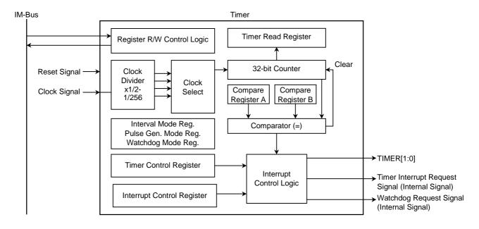
Figure 12.2.2 Timer Internal Block Diagram
