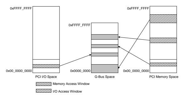
Figure 10.3.5 Target Access Memory Window
