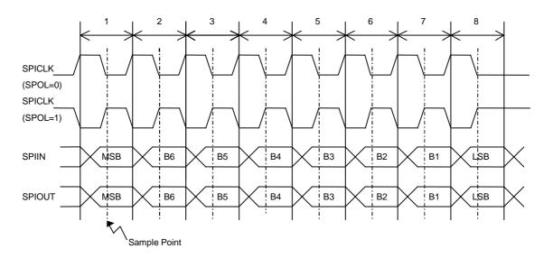
Figure 17.3.2 Transfer format when SPHA is "1".
