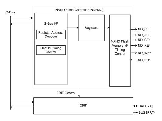
Figure 18.2.1 NAND Flash Memory Controller Block Diagram
