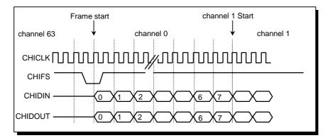
Figure 16.3.11 CHI Frame Structure Example
