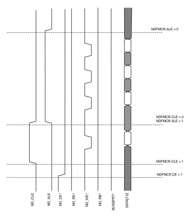
Figure 18.5.1 Command and Address Cycle (NDFMCR.BSPRT = 0)
