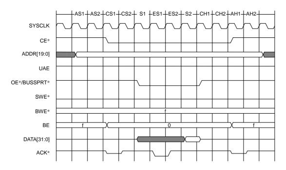
Figure 7.5.30 1-word Single Read (0 Wait, SHWT=2, External ACK\*, 32-bit Bus)
