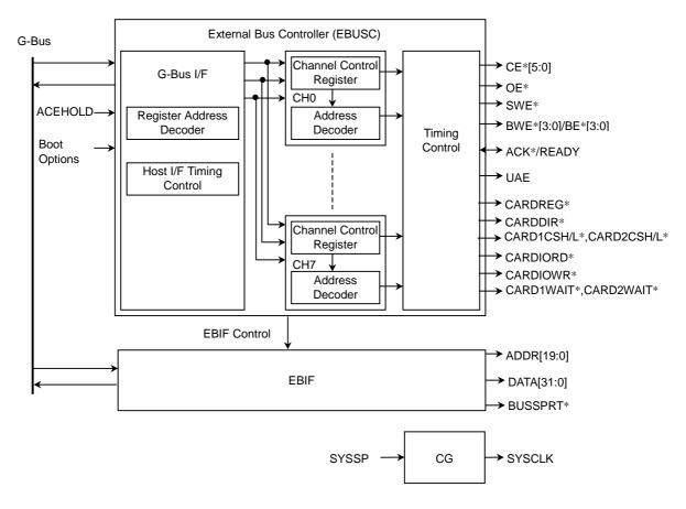
Figure 7.2.1 Block Diagram of External Bus Controller
