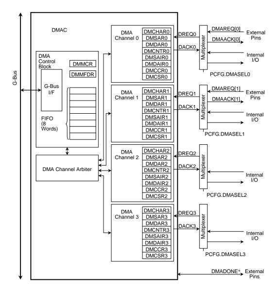
Figure 8.2.1 DMA Controller Block Diagram
