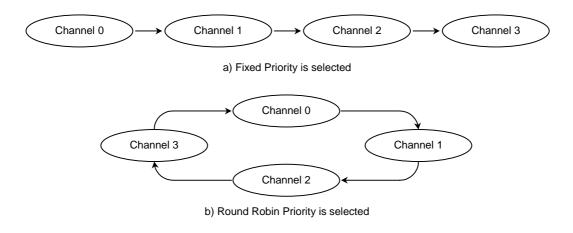
Figure 8.3.7 DMA Channel Arbitration
