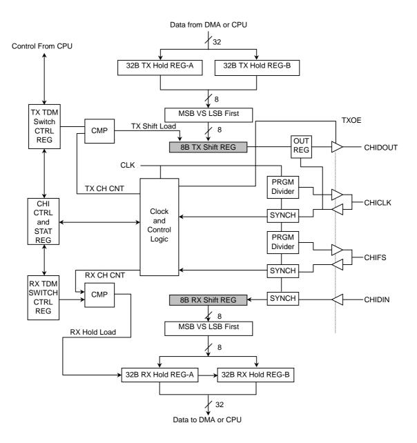
Figure 16.2.1 CHI Module Block Diagram
