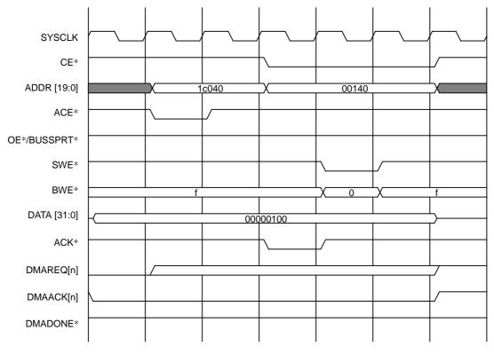
8.5.3 Single Address Single Transfer from I/O to Memory (32-bit SRAM)
