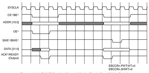
Figure 7.3.5 SWHT Disable (Normal Mode, Single Read/Write Cycle)
