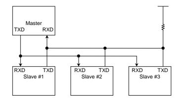
Figure 11.3.4 Example Configuration of Multi-Controller System
