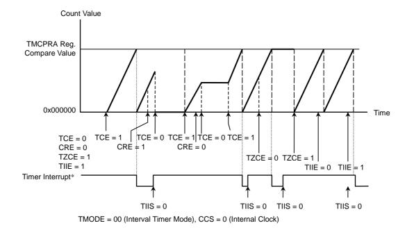
Figure 12.3.1 Operation Example of Interval Timer (Using Internal Clock)
