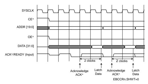
Figure 7.3.12 ACK\* Input Timing (Burst Read Cycle)
