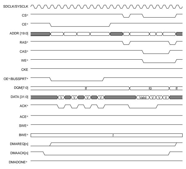
8.5.16 External I/O Device – SDRAM Dual Address Transfer
