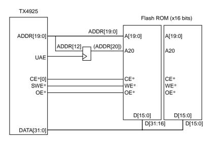
Figure 7.6.1 Flash ROM (x16 Bits) Connection Example (32-bit Data Bus)
