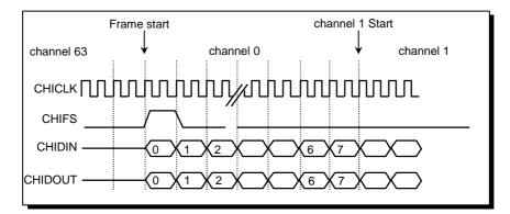
Figure 16.3.8 CHI Frame Structure Example
