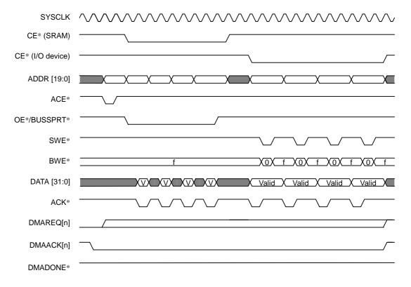
Figure 8.5.17 Dual Address Transfer from SRAM to External I/O Device (4-word Burst Transfer from 32-bit Bus SRAM)
