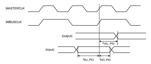
Figure 22.5.12 Timing Diagrams: PIO Interface
