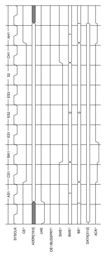
Figure 7.5.31 1-word Single Write (PWT: WT=2, SHWT=1, READY, 32-bit Bus)
