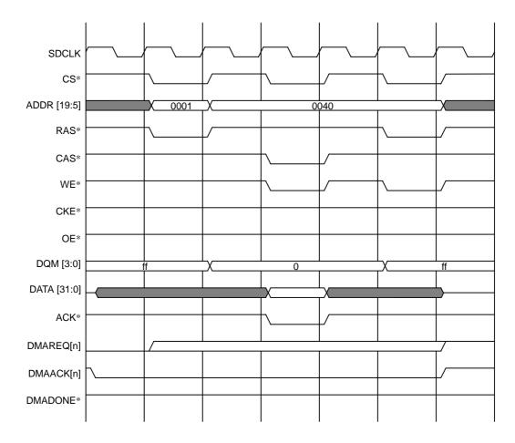
8.5.11 Single Address Single Transfer from I/O to Memory (32-bit SDRAM)
