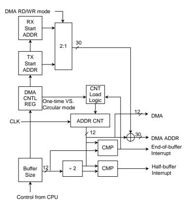
Figure 16.3.3 CHI DMA Address Generation
