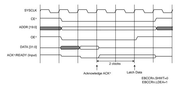
Figure 7.3.10 ACK\* Input Timing (Single Read Cycle)
