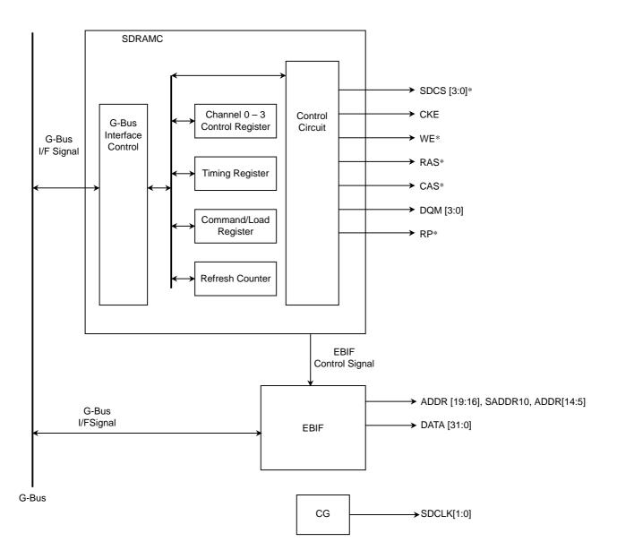
Note: Address signals for SDRAM are ADDR[19:16], SADDR10, and ADDR[14:5]. Don't use ADDR[15] for SDRAM.
