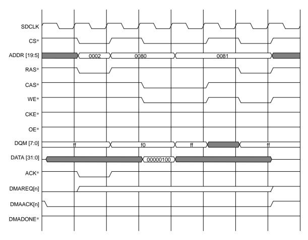
8.5.14 Single Address Single Transfer from I/O to Memory (32-bit SDRAM)
