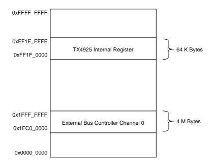
Figure 4.1.1 Physical Address Map at Initializing System
