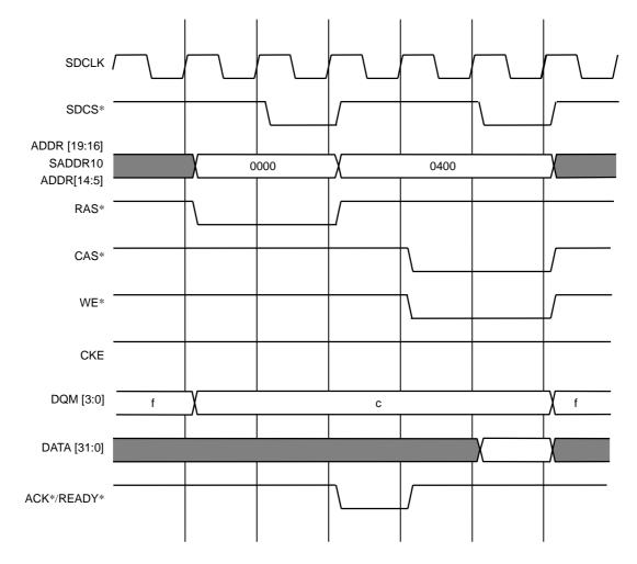
Figure 9.5.4 Half-Word Single Write ( $t_{RCD} = 3$ ,  $t_{DA} = 1$ , 32-bit Bus)
