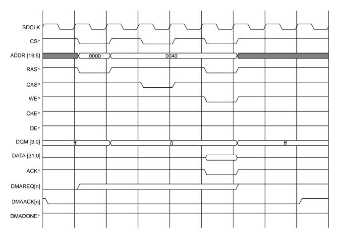
8.5.10 Single Address Single Transfer from Memory to I/O (32-bit SRAM)
