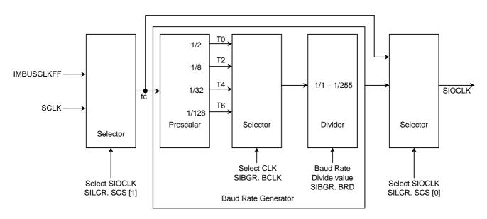
Figure 11.3.2 Baud Rate Generator and SIOCLK Generator
