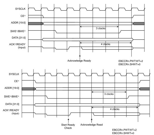
Figure 7.3.15 Ready Input Timing (Write Cycle)
