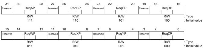
This register is only valid when using the on-chip PCI Bus Arbiter.
