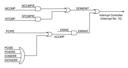
Figure 10.4.67 PDMAC Interrupt Signaling
