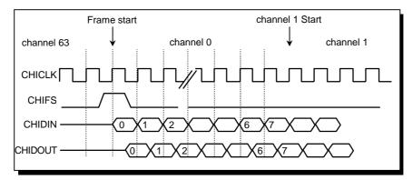
Figure 16.3.6 CHI Frame Structure Example
