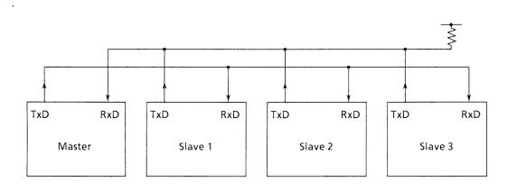
Note: TxD pin of the slave controllers must be in open drain output mode.
