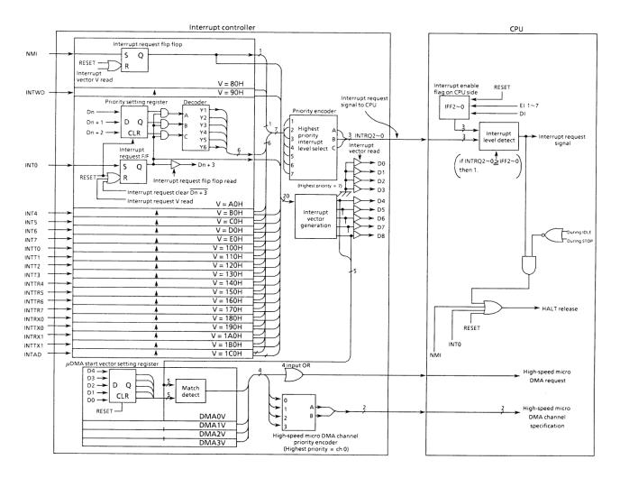
Figure 3.3.3 (1) Block Diagram of Interrupt Controller
