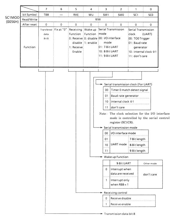
Figure 3.11 (6). Serial Mode Control Register (Channel 1, SC1MOD)
