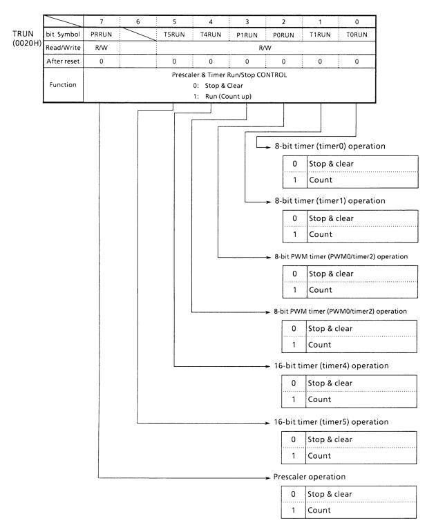
Figure 3.8 (7). Timer Operation Control Register (TRUN)
