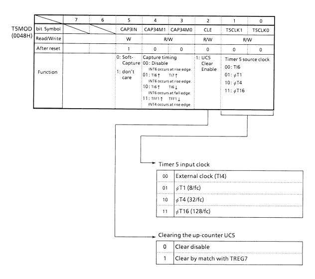
Figure 3.9 (6). 16-Bit Timer Mode Control Register (T5MOD) (1/2)
