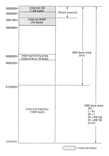
Note : The start address after reset is 8000H. Resetting sets the stack pointer (XSP) on the system mode side to 100H.
