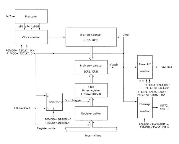
Figure 3.8 (12). Block Diagram of 8-Bit Timer Mode
