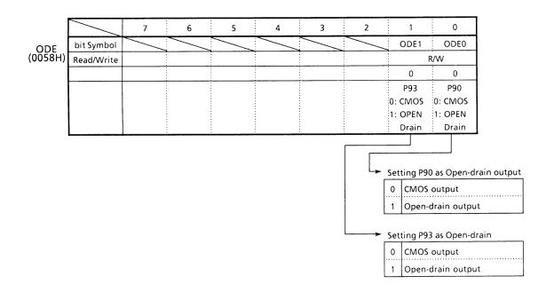
Port 3.11 (11). Port 9 Open Drain Enable Register (ODE)
