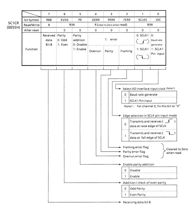
Note: As all error flags are cleared after reading, do not test only a single bit with a bit-testing instruction.
