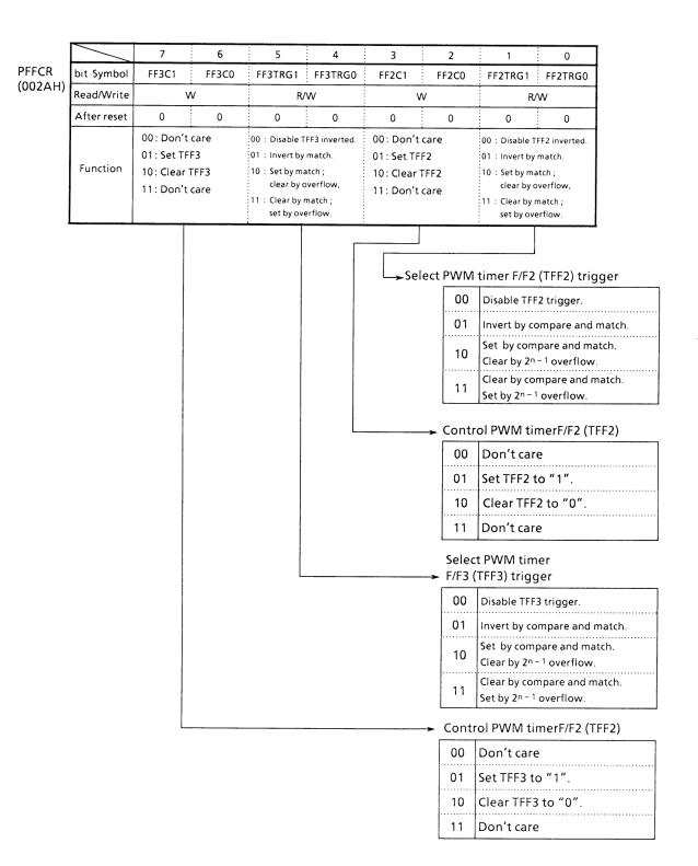
Figure 3.8 (6). 8-Bit PWM F/F Control Register
