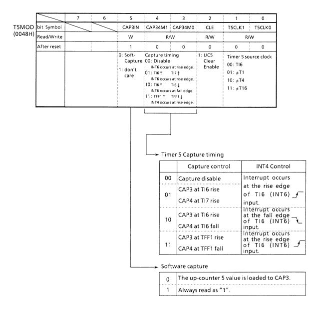
Figure 3.9 (7). 16-Bit Timer Control Register (T5MOD) (2/2)
