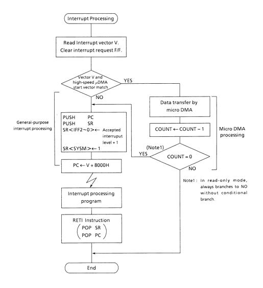
Figure 3.3 (1) Interrupt Processing Flowchart
