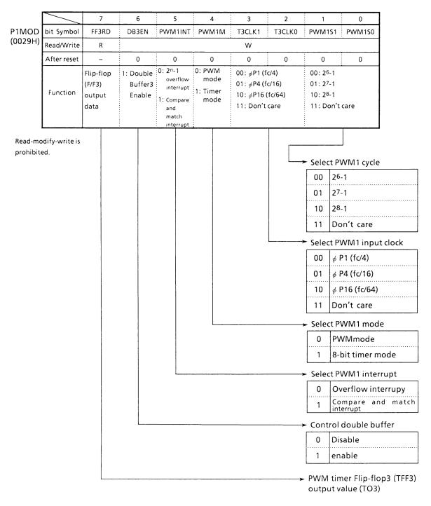
Figure 3.8 (5). 8-Bit PWM1 Mode Control Register
