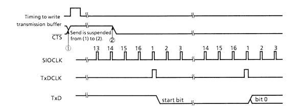
Note 1: If the CTS signal falls during transmission, the next data is not sent after the completion of the current transmission. Note 2: Transmission starts at the first TxDCLK clock fall after the CTS signal falls.
