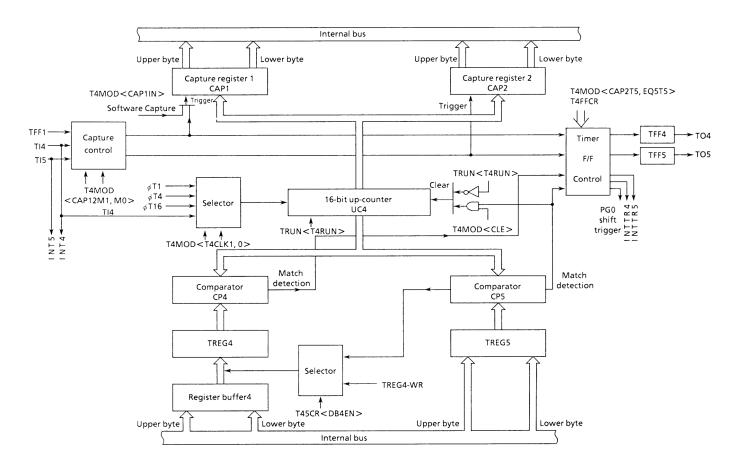
Figure 3.9 (1). Block Diagram of 16-Bit Timer (Timer 4)
