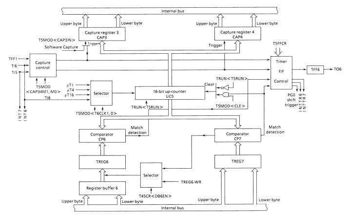
Figure 3.9 (2). Block Diagram of 16-Bit Timer (Timer 5)
