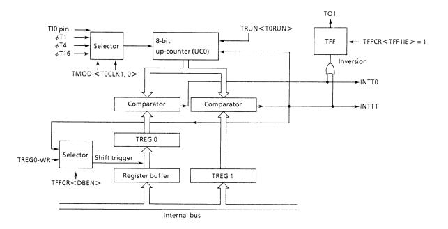
Figure 3.7 (11). Block Diagram of 8-Bit PPG Output Mode
