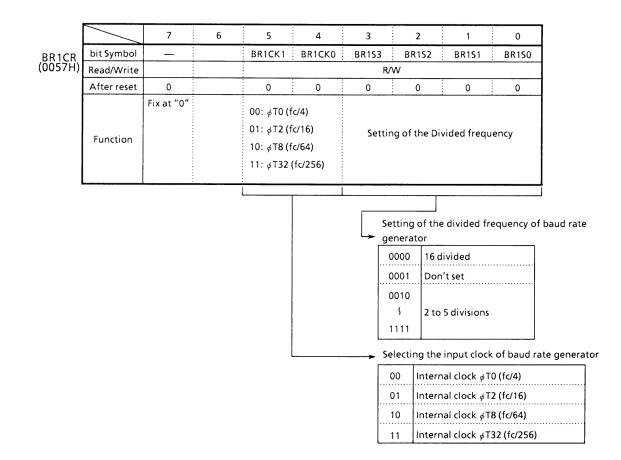
Note: To use baud rate generator, set TRUN < PRRUN> to "1", putting the prescaler in RUN mode.
