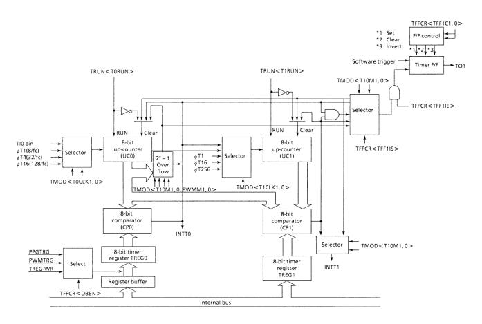
Figure 3.7 (1). Block Diagram of 8-Bit Timers (Timers 0 and 1)
