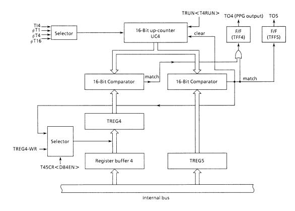
Figure 3.9 (13). Block Diagram of 16-Bit PPG Mode
