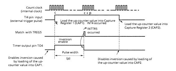
Figure 3.9 (15). One-Shot Pulse Output (without Delay)
