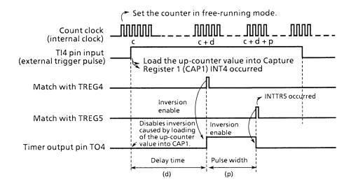
Figure 3.9 (14). One-Shot Pulse Output (with Delay)
