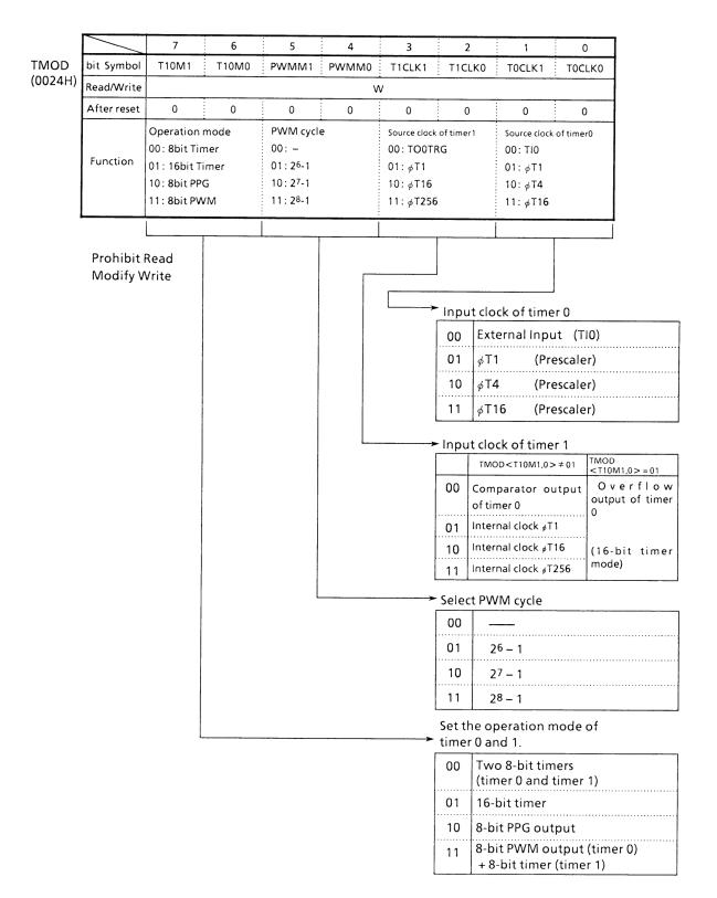
Figure 3.7 (5). Timer Mode Control Register (TMOD)
