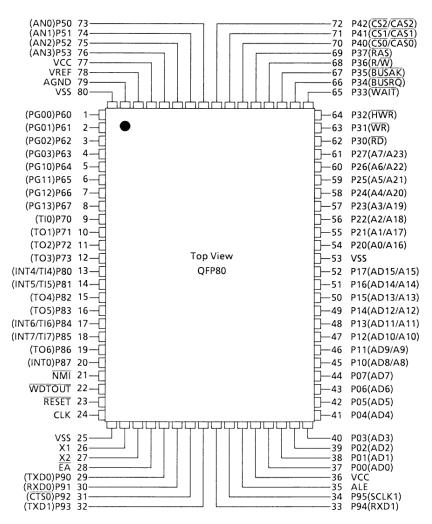
Note : Because the TMP96C141AF has an external ROM, P00 to P17 pins are fixed to AD0 to AD15; P30 to RD; and P31 to WR.
