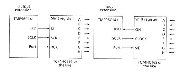
Figure 3.11 (17). Example of SCLK Output Mode Connection
