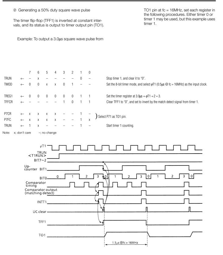
Figure 3.7 (7). Square Wave (50% Duty) Output Timing Chart
