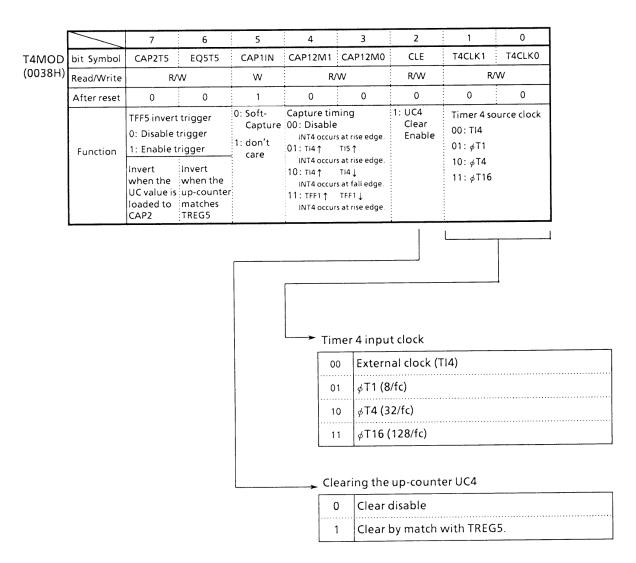
Figure 3.9 (3). 16-Bit Timer Mode Controller Register (T4MOD) (1/2)
