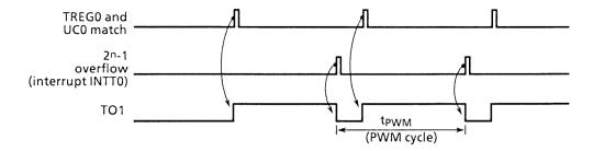
Figure 3.7 (13). 8-Bit PWM Waveforms
