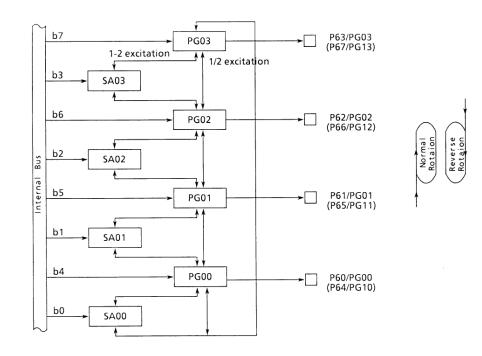
Figure 3.10 (1). Port 6/PG Circuit
