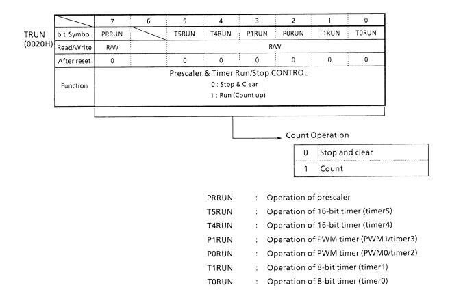
Figure 3.7 (4). Timer Operation Control Register (TRUN)
