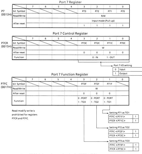
Note : P70/TI0 pin does not have a register changing PORT/FUNCTION.
