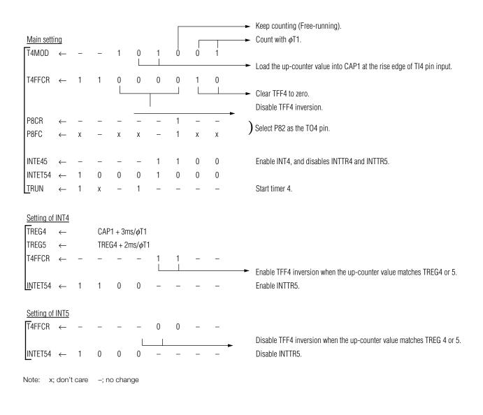
When delay time is unnecessary, invert timer flip-flop TFF4 when the up-counter value is loaded into capture register 1 (CAP1), and set the CAP1 value (c) plus the one-shot pulse width (p) to TREG5 when the interrupt INT4 occurs. The TFF4 inversion should be enabled when the up-counter (UC4) value matches TREG5, and disabled when generating the interrupt INTTR5.
