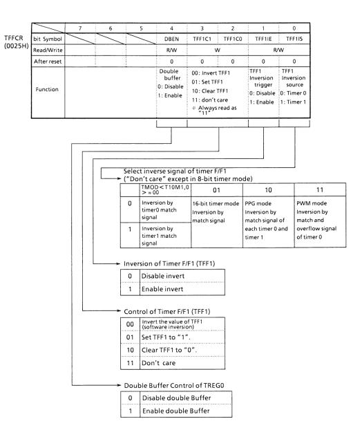
Figure 3.7 (6). Timer Flip-Flop Control Register (TFFCR)
