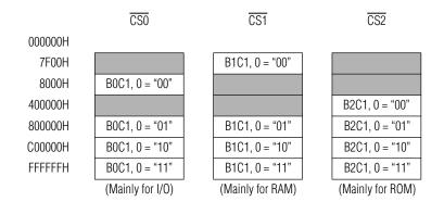
Supplement 1: Access priority is highest for built-in I/O, then built-in memory, and lowest for the chip select/wait controller.
