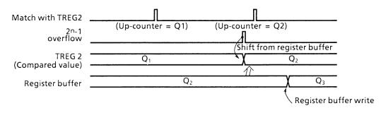
Figure 3.8 (10). Register Buffer Operation
