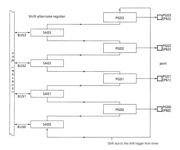
Figure 3.10 (7). Pattern Generation Mode Block Diagram (PG0)
