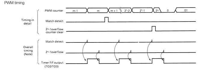
Figure 3.8 (8). Output Waves in PWM Timer Mode
