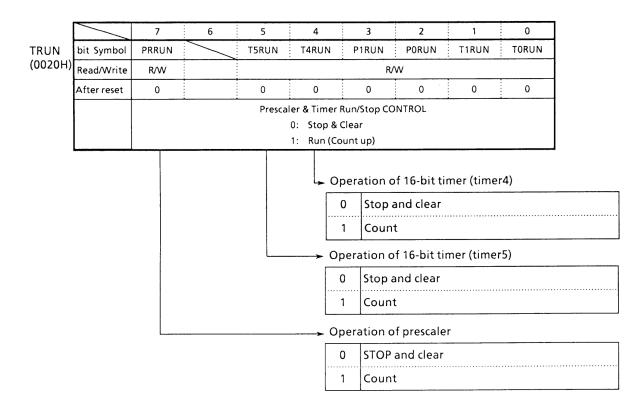
Figure 3.9 (10). Timer Operation Control Register (TRUN)
