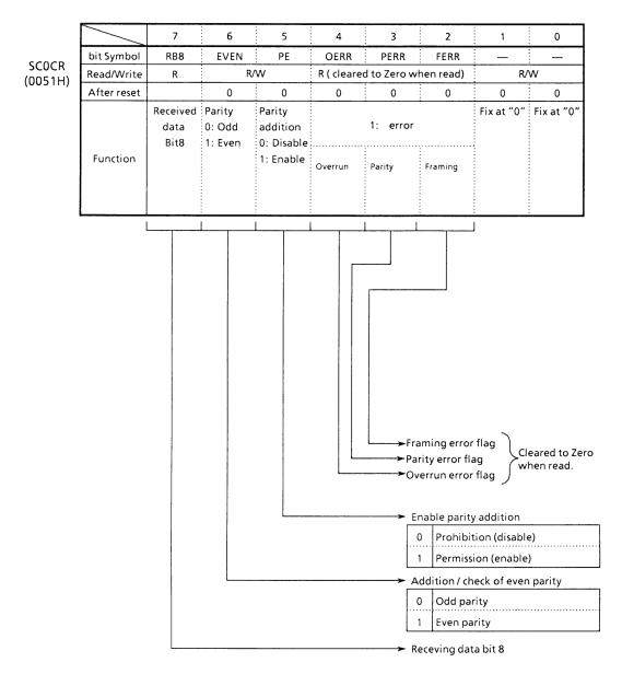
Note: Serial control register for channel 1 is SC1CR (55H). As all error flags are cleared after reading, do not test only a single bit with a bit-testing instruction.
