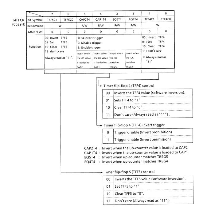
Figure 3.9 (5). 16-Bit Timer 4 F/F Control (T4FFCR)
