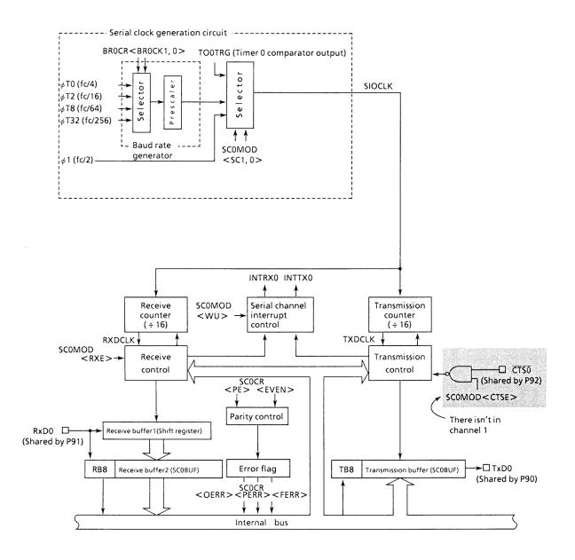
Figure 3.11 (12). Block Diagram of the Serial Channel 0
