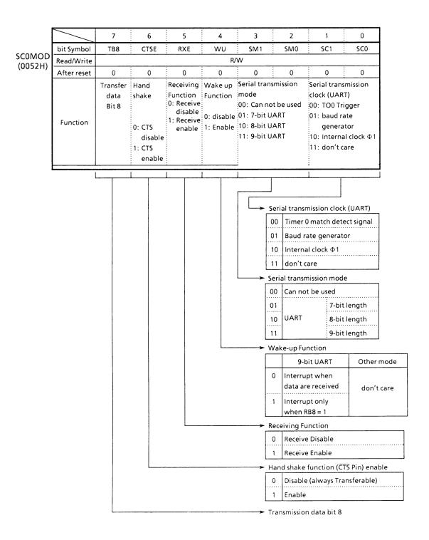
Note: There is SC1MOD (56H) in Channel 1 Figure 3.11 (2). Serial Mode Control Register (Channel 0, SC0MOD)
