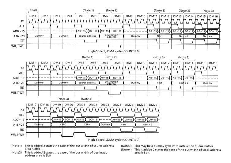
The following timing chart is a high-speed  $\mu\text{DMA}$  cycle of the Transfer Address Increment mode (the other mode exe-
