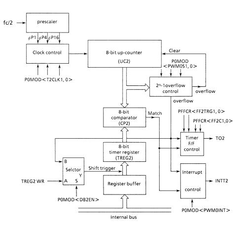
Figure 3.8 (9). Block Diagram of PWM Timer Mode (PWM0)
