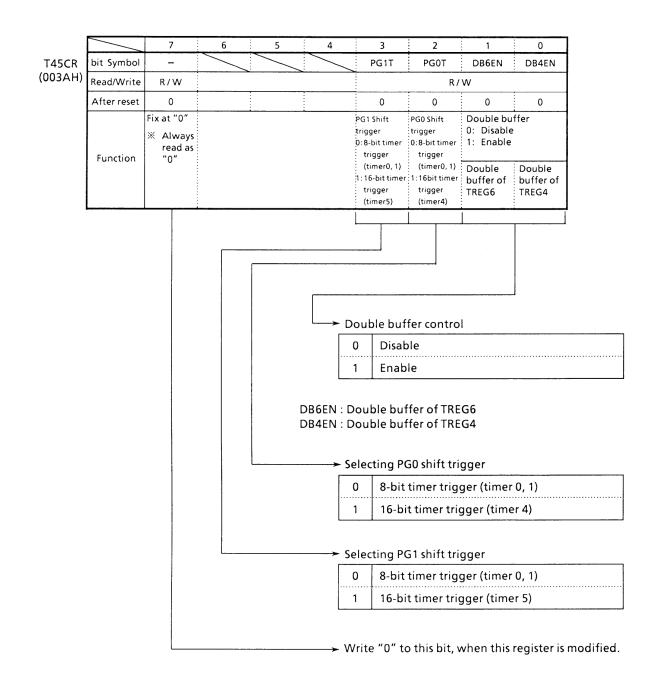
Figure 3.10 (5). 16-bit Timer Trigger Control Register (T45CR)
