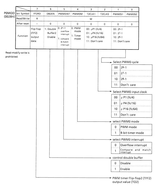
Figure 3.8 (4). 8-Bit PWM0 Mode Control Register
