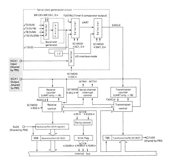
Figure 3.11 (13). Block Diagram of the Serial Channel 1
