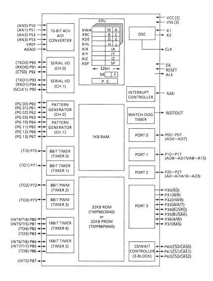
Figure 1. TMP96C141AF Block Diagram
