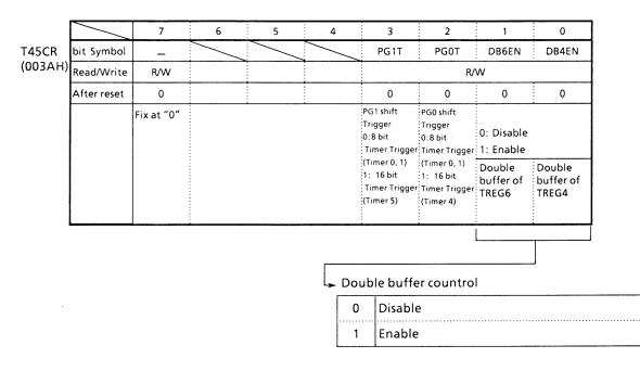
DB6EN : Double buffer of TREG6 DB4EN : Double buffer of TREG4
