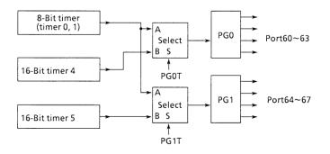
Figure 3.10 (6). Connection of Timer and Pattern Generator
