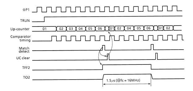
Figure 3.8 (11). Square Wave (50% Duty) Output Timing Chart
