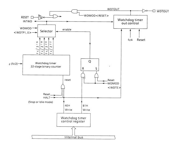
Figure 3.13 (1). Block Diagram of Watchdog Timer
