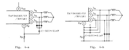
d) It is recommended to connect a path capacitor directly from V<sub>CC</sub> terminal (9 pin) without giving common impedance to GND. Further, it is also effective to insert C<sub>2</sub>  $(0.01 \sim 0.1 \mu F)$ .
