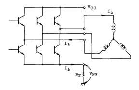
Further, if inputs (11 pin, 12 pin) are shorted or  $V_{11} \ge V_{12}$ , torque at the circuit becomes zero. However, this zero torque state also can be obtained by setting FRS input (10 pin) to specified voltage or by placing the circuit in open state and this is rather advantageous as current consumption is less.
