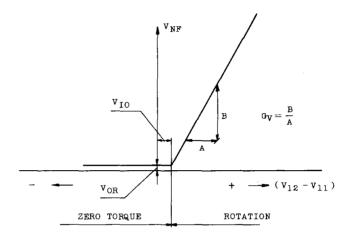
$\ensuremath{\text{V}_{\rm NF}}$  shows voltage drop at RF.
