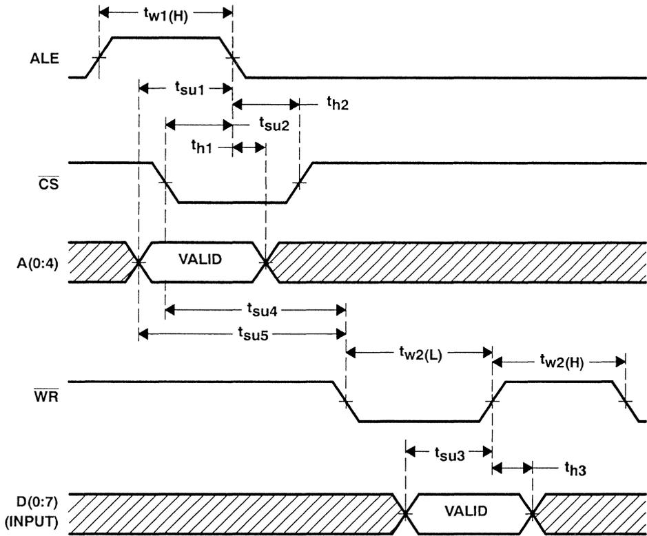
Figure 7-4. Processor Write Cycle (Multiplexed Address/Data Buses)
