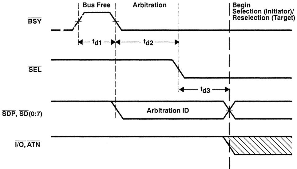
NOTE: " - - - - " waveform for  $\overline{BSY}$  (wired-OR signal) indicates that  $\overline{BSY}$  is being driven by another SCSI device.
