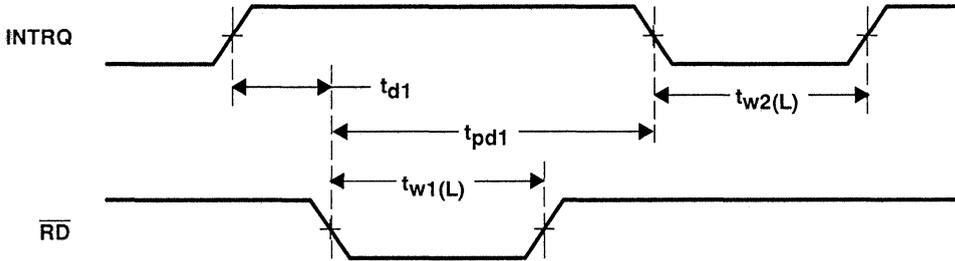
NOTE: Timing for chip select and address lines is shown in earlier timing diagrams.  $\overline{RD}$  is for functional or error interrupt status registers.
