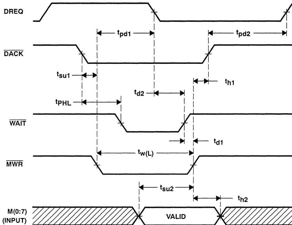
NOTE:  $\overline{\text{WAIT}}$  timing is shown only for demand-mode transfers that have automatically entered the nondemand mode due to inadequate FIFO status or approaching end of transfer. The  $\overline{\text{WAIT}}$  signal is inactive for nondemand transfers.
