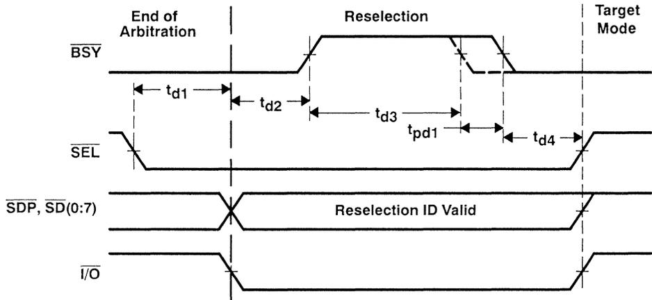
NOTE: "----" waveform for  $\overline{BSY}$  (wired-OR signal) indicates that  $\overline{BSY}$  is being driven by the initiator.
