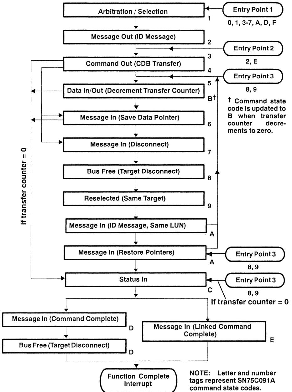
Figure 4-1. Select with  $\overline{ATN}$  and Transfer Command
