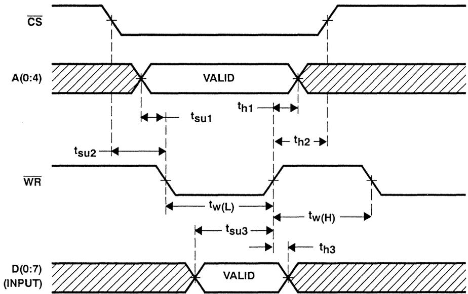
Figure 7-2. Processor Write Cycle (Nonmultiplexed Address/Data Buses)
