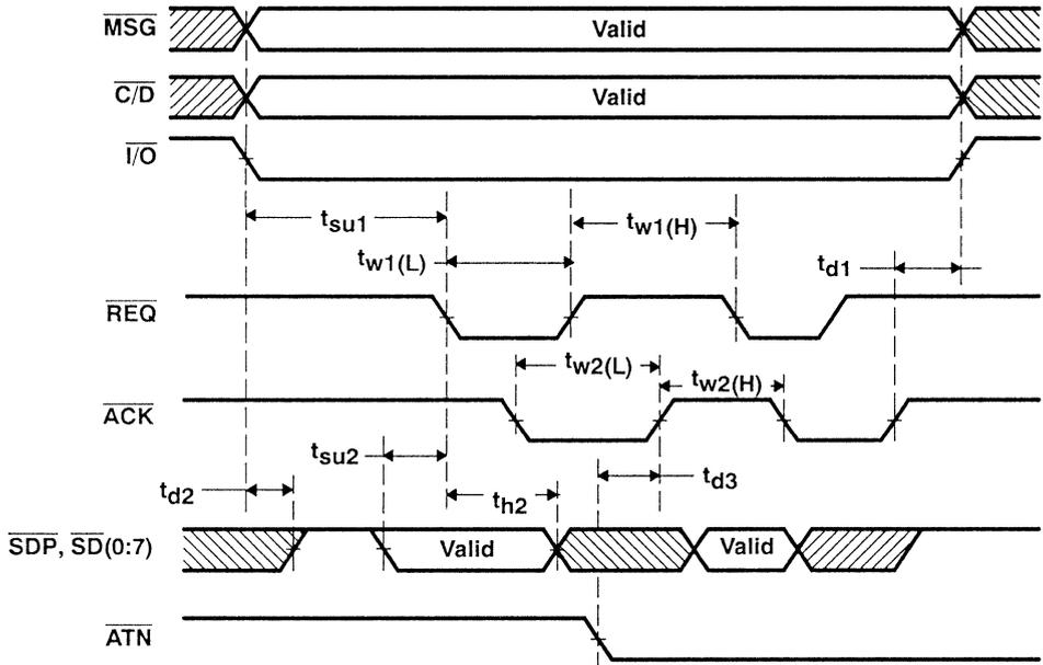
Figure 7-28. SCSI Bus Synchronous Data-In Transfer (Initiator)
