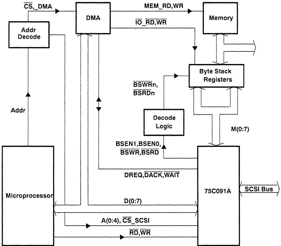
NOTE: For 16-bit byte stack operation, no decode logic is required to produce  $\overline{BSWRn}$  and  $\overline{BSRDn}$ . These signals are decoded internally to minimize the external logic required for this application.
