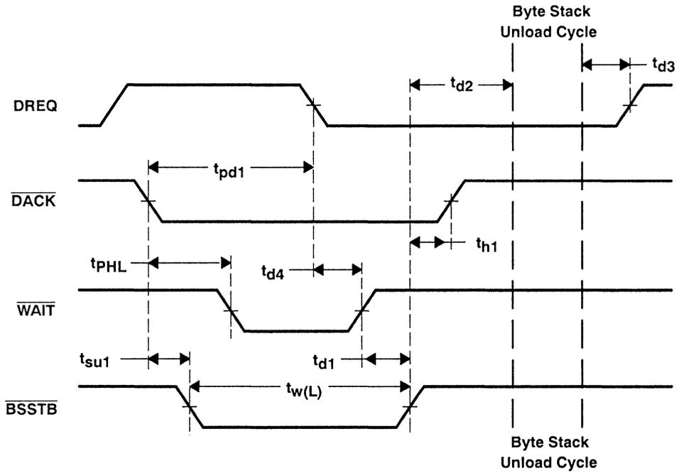
Figure 7-10. DMA Write – Byte Stack, Nondemand Mode
