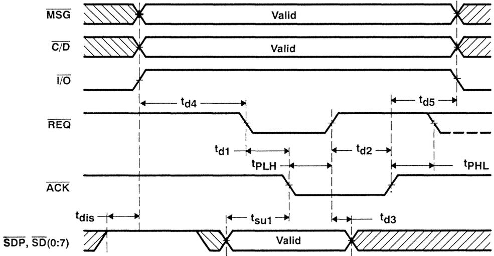
Figure 7-27. SCSI Bus Asynchronous Information Transfer Out (Target)
