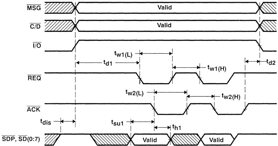
Figure 7-31. SCSI Bus Synchronous Data-Out Transfer (Target)
