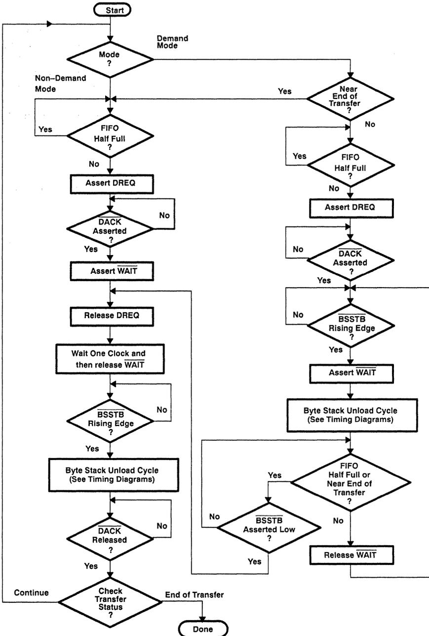
Figure 6-5. Flowchart for DMA Write (Byte Stack Mode)
