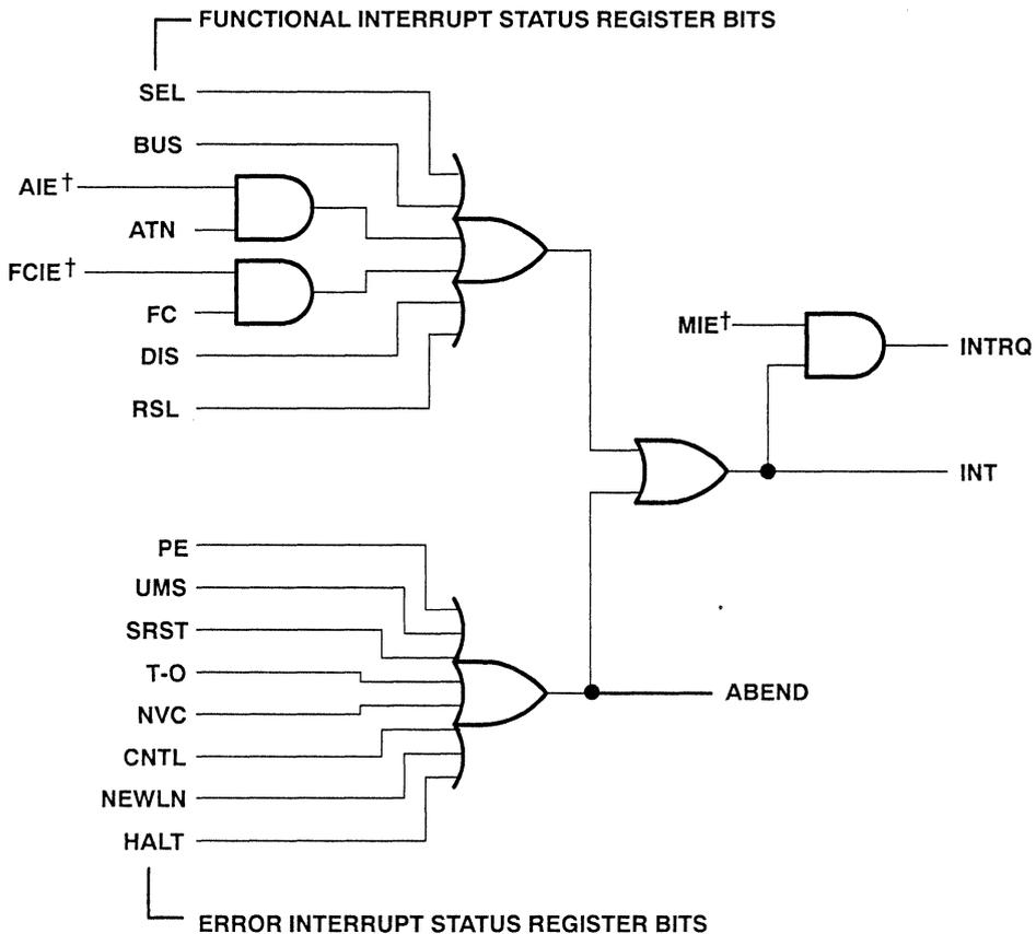
† These inputs are from the Interrupt Enable register.
