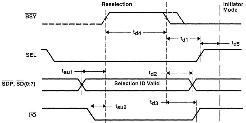
NOTE: "----" waveform for  $\overline{BSY}$  (wired-OR signal) indicates that  $\overline{BSY}$  is being driven by the target.
