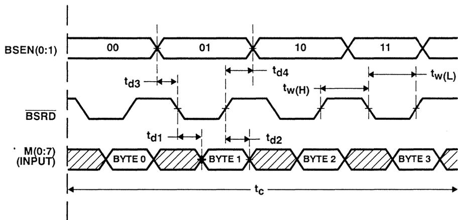
Figure 7-16. Byte Stack Unload Cycle (24- or 32-Bit)
