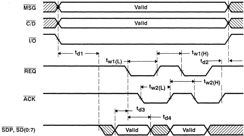
Figure 7-29. SCSI Bus Synchronous Data-In Transfer (Target)
