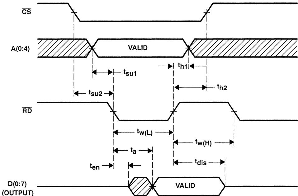
**Figure 7-1. Processor Read Cycle (Nonmultiplexed Address/Data Buses)**
