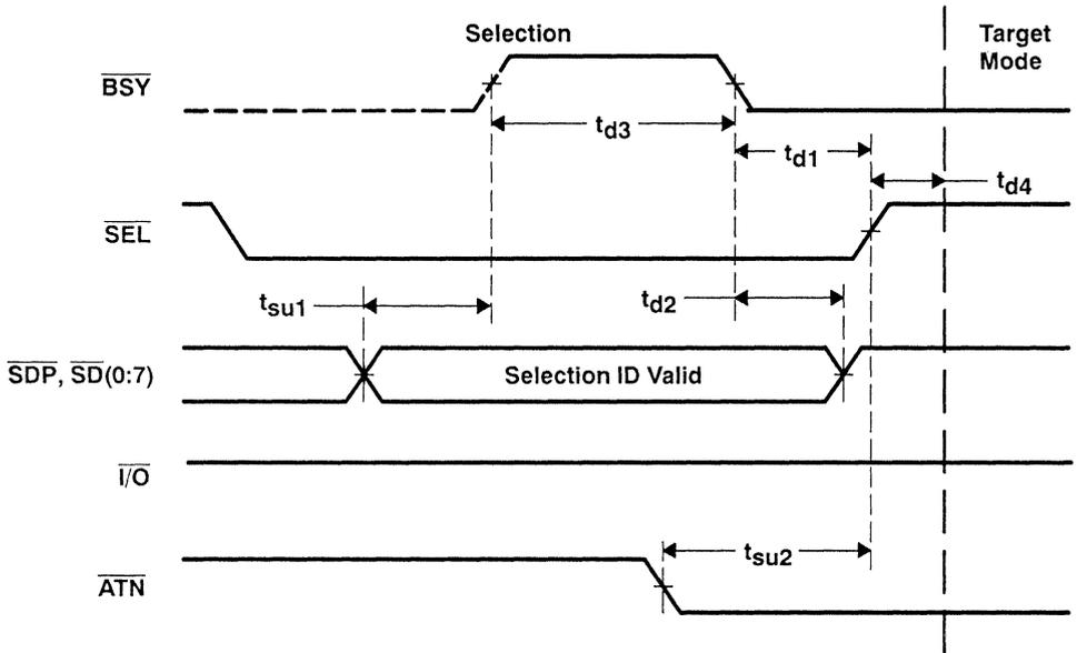
NOTE: "----" waveform for  $\overline{BSY}$  (wired-OR signal) indicates that  $\overline{BSY}$  is being driven by the initiator.
