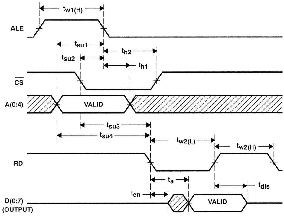
Figure 7-3. Processor Read Cycle (Multiplexed Address/Data Buses)
