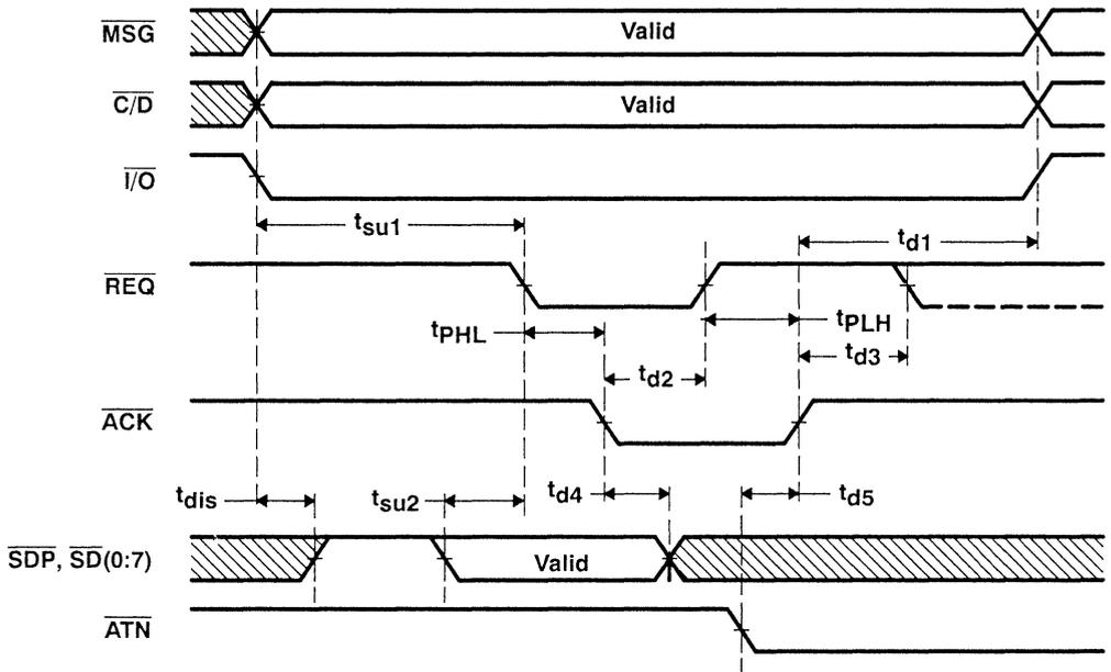
Figure 7-24. SCSI Bus Asynchronous Information Transfer In (Initiator)
