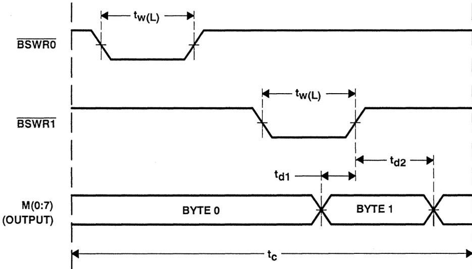
**Figure 7-13. Byte Stack Load Cycle (16-bit)**
