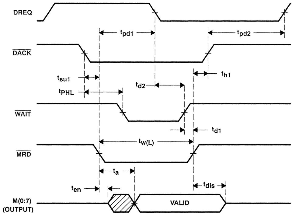
NOTE:  $\overline{\text{WAIT}}$  timing is shown only for demand-mode transfers that have automatically entered the nondemand mode due to inadequate FIFO status or approaching end of transfer. The  $\overline{\text{WAIT}}$  signal is inactive for nondemand transfers.
