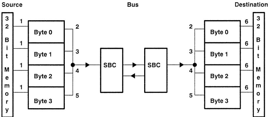
Figure 6-2. Byte Stack Mode Data Compression and Expansion
