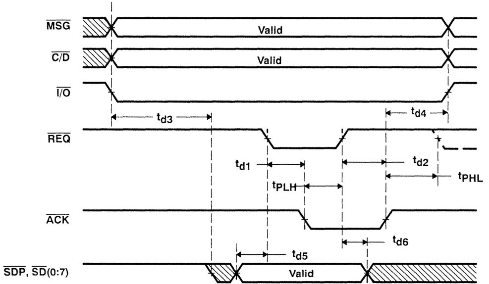
Figure 7-25. SCSI Bus Asynchronous Information Transfer In (Target) (TARGET TO INITIATOR)
