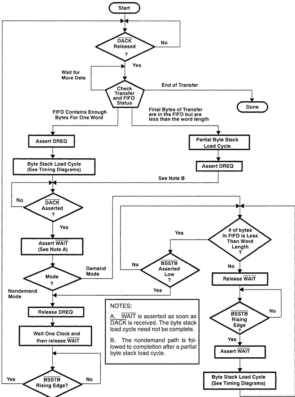
Figure 6-4. Flowchart for DMA Read (Byte Stack Mode)
