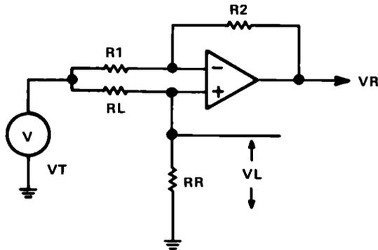
FIGURE 17 – EQUIVALENT CIRCUIT FOR TWO-TO-FOUR WIRE HYBRID
