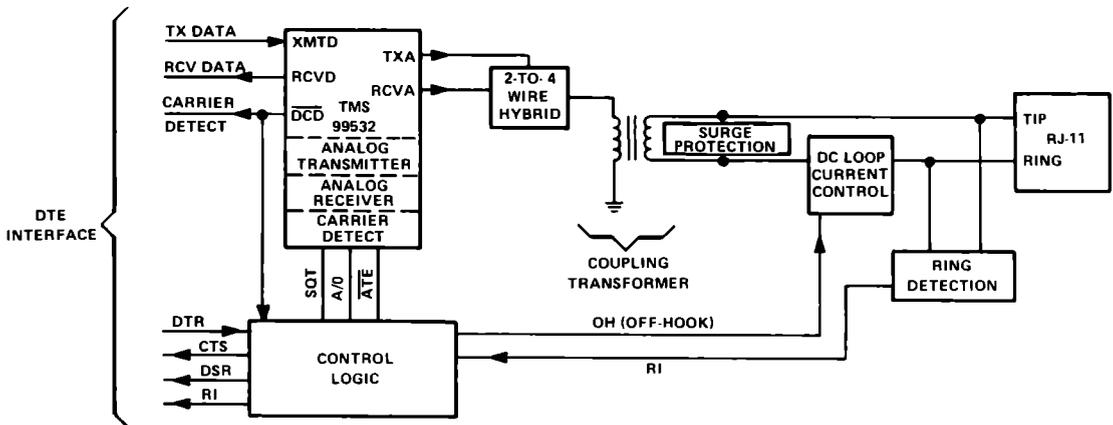
FIGURE 14 - BLOCK DIAGRAM OF DIRECT CONNECT MODEM
