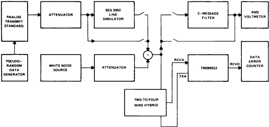
FIGURE 24 - MODEM TEST SET
