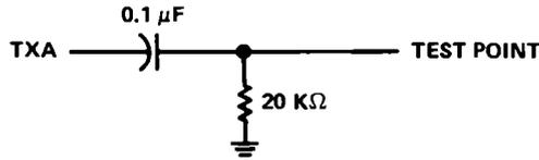
FIGURE 28 – LOADING FOR VOLTAGE LEVEL MEASUREMENT
