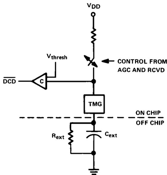
FIGURE 10 – EQUIVALENT CIRCUIT FOR CARRIER DETECT TIMING
