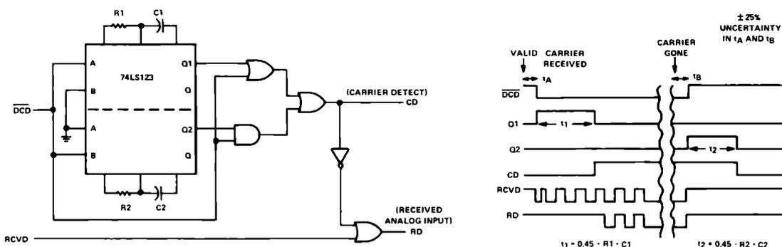
FIGURE 20 -  $\overline{\text{DCD}}$  PIN CONNECTION FOR EXTERNAL TIMER CIRCUIT
