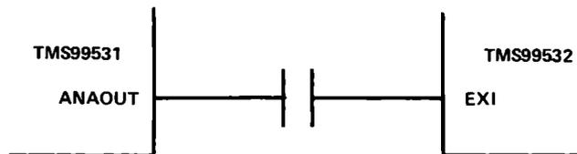
FIGURE 23 – CONNECTION OF TMS99532 MODEM TO TMS99531 DIALER
