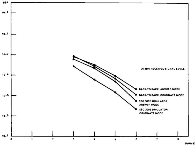
FIGURE 25 - TMS99532 BIT ERROR RATE CURVES (TYPICAL)
