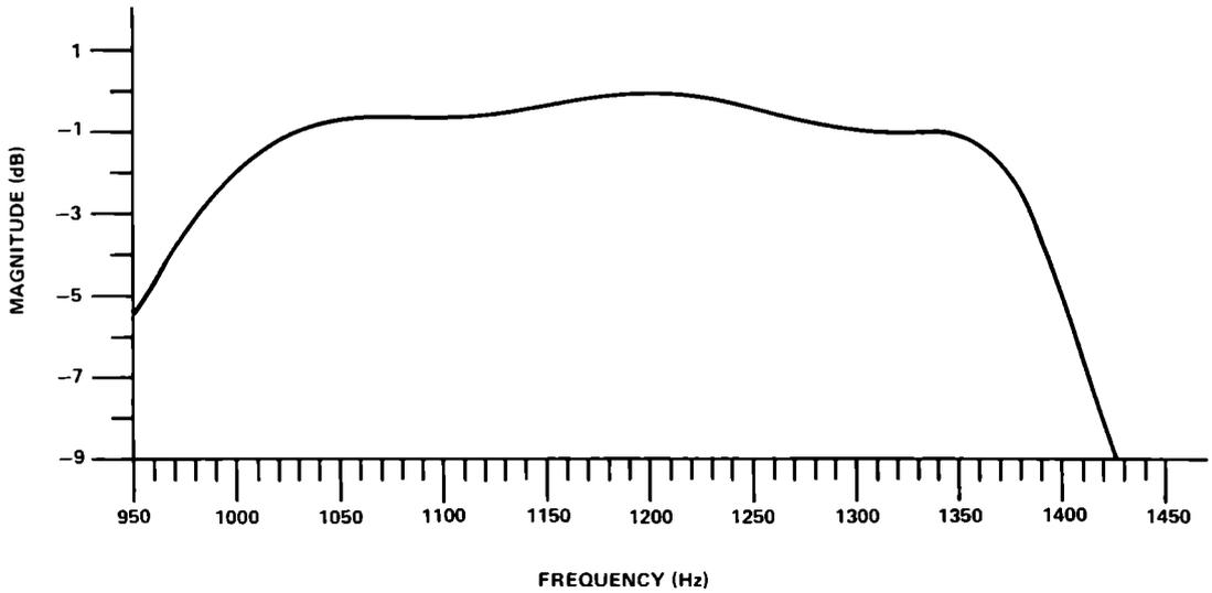
**FIGURE 7 - IDEAL LOW-FREQUENCY PASS BAND RESPONSE**
