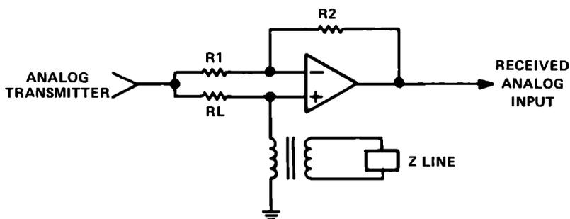
FIGURE 16 - TWO-TO-FOUR WIRE HYBRID
