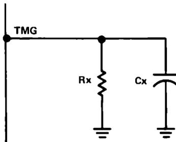
NOTE: In all applications, the TMG pin should have a parallel resistor/capacitor connection to ground. In addition, Rx should never be smaller than 4.7 MΩ. The TMS99532 modem will not operate properly if the TMG pin is tied off or left floating.
