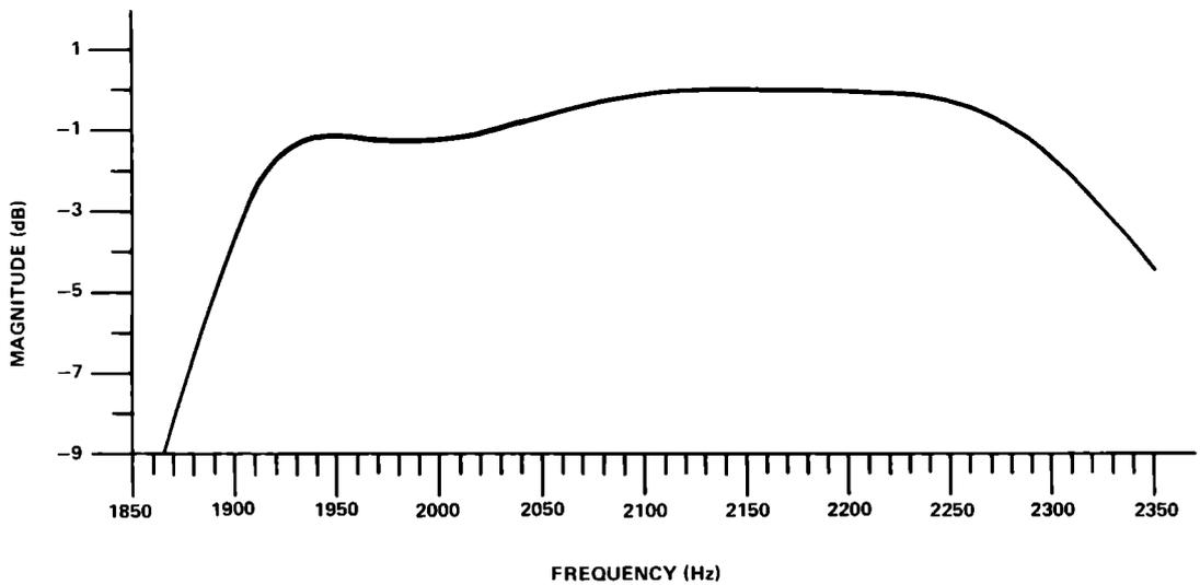
**FIGURE 8 - IDEAL HIGH-FREQUENCY PASS BAND RESPONSE**
