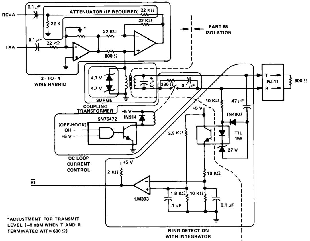
FIGURE 15 - EXAMPLE OF DIRECT CONNECTION (NOT FCC APPROVED)
