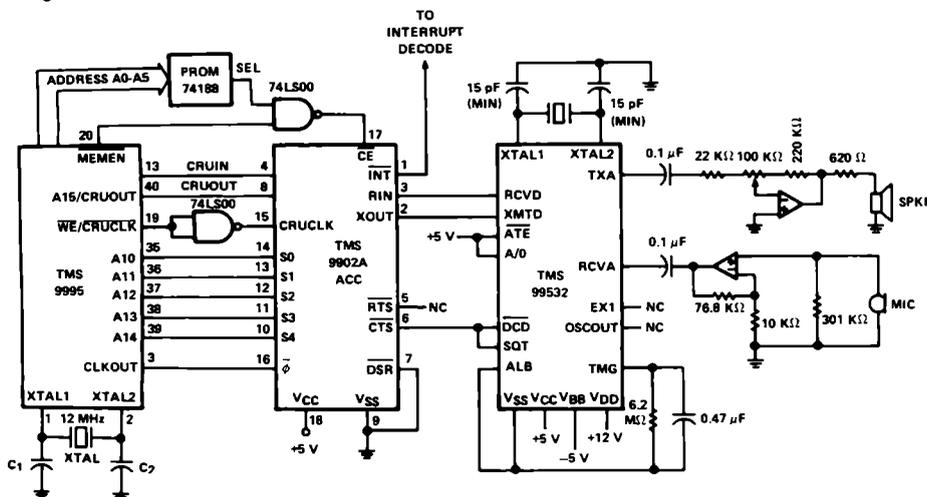
FIGURE 13 – TMS9995 SYSTEM UTILIZING ORIGINATE-MODEM
