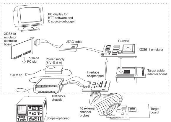
Figure 1–1. XDS522A Emulation System Components
