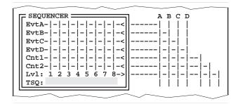
The sequencer operates as an 8-level state machine. Up to six inputs are ORed to determine whether the sequencer should advance to the next level:
