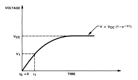
Figure 16. Voltage on the TMS320C25 Reset Pin
