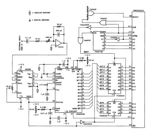
Figure 21. Interface of the ADADC84 to the TMS320C25
