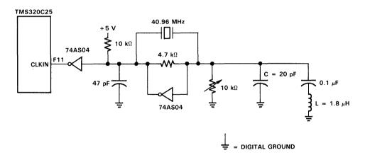
Figure 17. Crystal Oscillator Circuit
