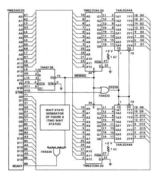
Figure 11. Interface of the TMS27C64-20 to the TMS320C25
