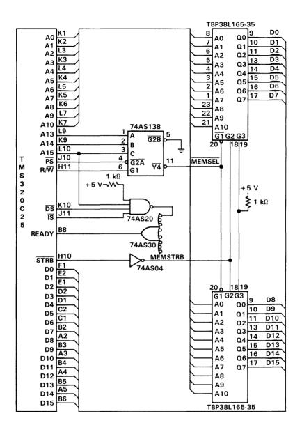
Figure 4. Interface of the TBP38L165-35 to the TMS320C25
