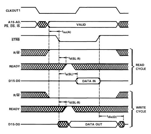
Figure 1. Read and Write Timings
