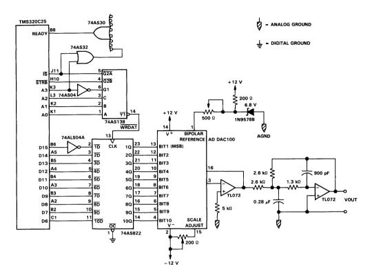
Figure 23. Interface of the ADDAC100 to the TMS320C25
