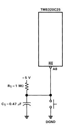
Figure 15. Reset Circuit
