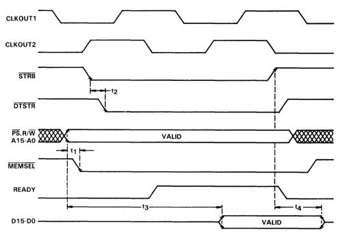
Figure 10. Interface Timing of the WS57C64F-12 to the TMS320C25
