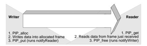
Internally, pipes are implemented as a circular list; frames are reused at the writer end of the pipe after PIP\_free releases them.
