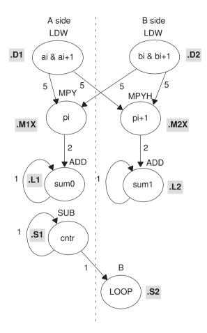
Example 5–17. Linear Assembly for Fixed-Point Dot Product Inner Loop With LDW (With Allocated Resources)
