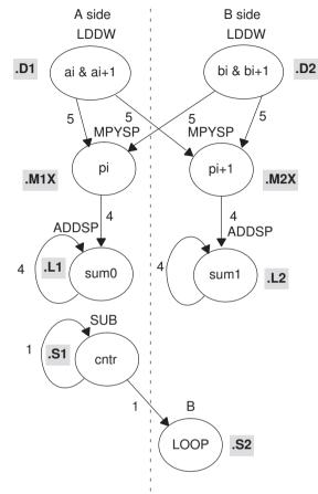
Example 5–18. Linear Assembly for Floating-Point Dot Product Inner Loop With LDDW (With Allocated Resources)
