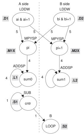
Example 5–22. Linear Assembly for Floating-Point Dot Product Inner Loop (With Conditional SUB Instruction)
