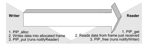
Internally, pipes are implemented as a circular list; frames are reused at the writer end of the pipe after PIP\_free releases them.
