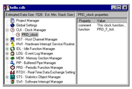
Unlike systems that create objects at run time with API calls that require extra target overhead (especially code space), all DSP/BIOS objects are statically configured and bound into an executable program image. In addition to minimizing the target memory footprint by eliminating run-time code and optimizing internal data structures, this static configuration strategy detects errors earlier by validating object properties before program execution.
