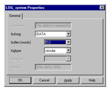
You see the properties dialog for this object. At run time, this log stores events traced by the system for various DSP/BIOS modules.
