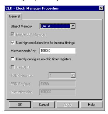
Notice that there is a check mark in the Enable CLK Manager box. When this box is checked, the timer interrupt drives the CLK manager.
