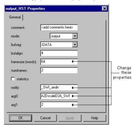
When this output channel contains an empty frame (because the target read and released a frame), it uses SWI\_andn to clear bit 1 of the mailbox.
