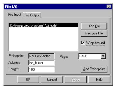
■ The Address field specifies where the data from the file is to be placed. The inp\_buffer is declared in volume.c as an integer array of BUFSIZE.
