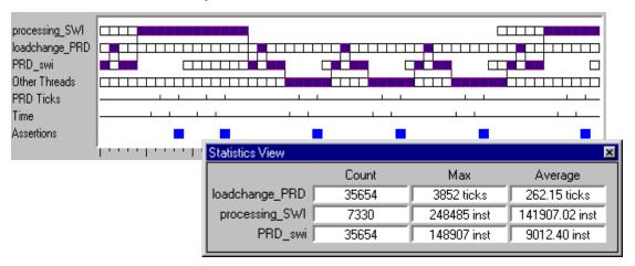
What is happening? The Max value for loadchange\_PRD increases when you increase the load beyond a certain point. With the increased load, the processing\_SWI takes so long to run that the loadchange\_PRD cannot begin running until long past its real-time deadline.
