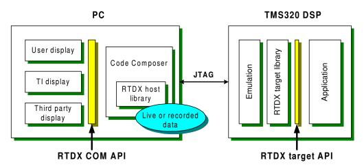
On the host platform, an RTDX library operates in conjunction with Code Composer Studio. Display and analysis tools can communicate with RTDX via an easy-to-use COM API to obtain the target data or send data to the DSP application. Designers may use standard software display packages, such as National Instruments' LabVIEW, Quinn-Curtis' Real-Time Graphics Tools, or Microsoft Excel. Alternatively, designers can develop their own Visual Basic or Visual C++ applications.
