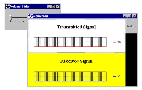
The slider.exe program must be started after RTDX is enabled and the program is running because it creates and opens the RTDX control channel when you run the program. If RTDX is not enabled at this point, slider.exe cannot open the channel.
