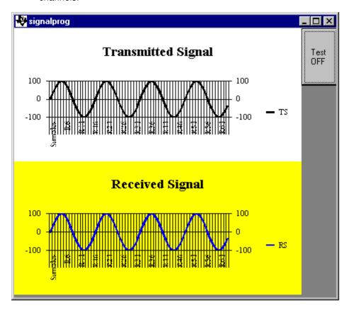
11) Slide the control in the Volume Slider window. This changes the volume of the output signal. Watch the amplitude of the Received Signal graph change.
