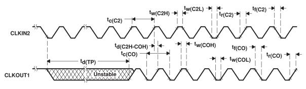
Figure 14. PLL Clock Generator Timing
