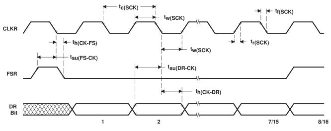
Figure 22. Serial-Port Receive Timing
