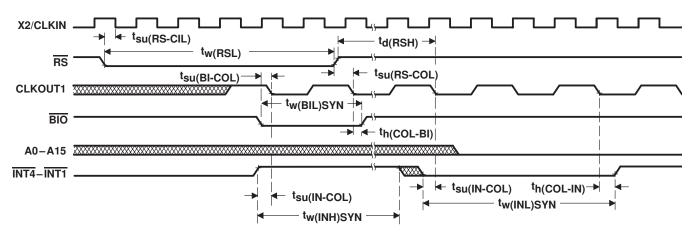
Figure 19. Reset, Interrupt, and BIO Timings
