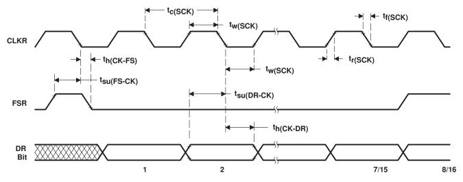
Figure 27. Buffered Serial-Port Receive Timing
