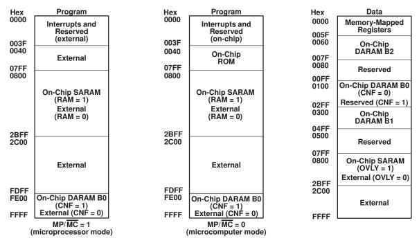
Figure 1. TMS320C50 and TMS320LC50 Memory Map
