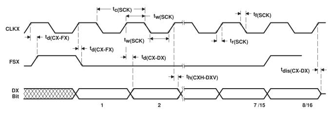
Figure 24. Serial-Port Transmit Timing of Internal Clocks and Internal Frames
