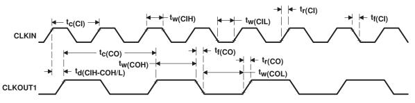
Figure 13. External Divide-by-Two Clock Timing
