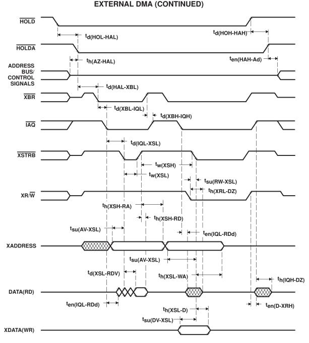
Figure 21. External DMA Timing
