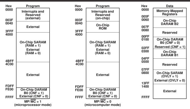
Figure 4. TMS320C53, TMS320C53S, TMS320LC53, and TMS320LC53S Memory Map
