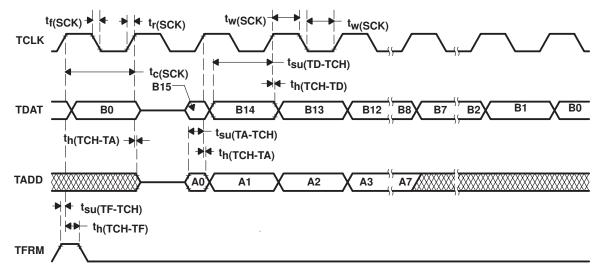
Figure 25. Serial-Port Receive Timing in TDM Mode
