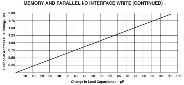
Figure 16. Address Bus Timing Variation With Load Capacitance
