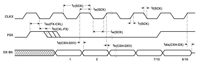
Figure 28. Buffered Serial-Port Transmit Timing of External Clocks and External Frames
