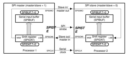
Figure 5–2. SPI Master/Slave Connection (4-Pin Option)
