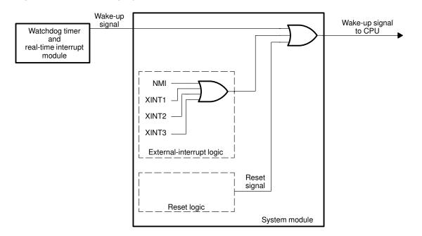
Figure 11–16. Waking Up the Device from Power Down
