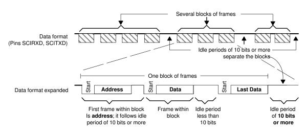
Figure 4–3. Idle-Line Multiprocessor Communication Format
