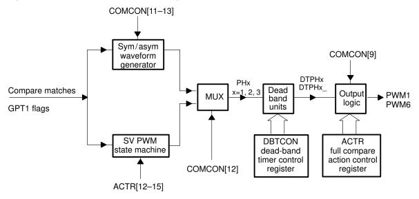
The PWM circuits are designed to minimize the CPU overhead and user intervention in generating pulse width modulated wave forms used in motor control and motion control applications. PWM generation with full compare units and the associated PWM circuits are controlled by the following control registers:
