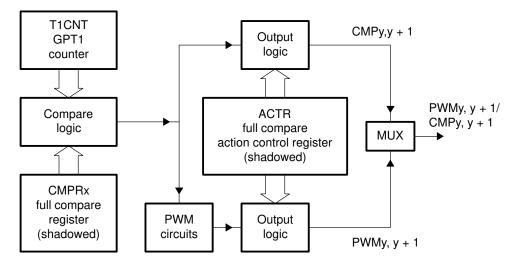
Figure 2–13. Full Compare Unit Block Diagram (x = 1, 2, 3; y = 1, 3, 5)
