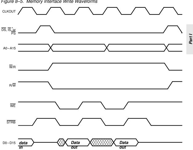
Figure 8–5. Memory Interface Write Waveforms
