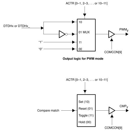
Figure 2–20. Output Logic Block Diagram (x = 1, 2, or 3; y = 1, 2, 3, 4, 5, or 6)
