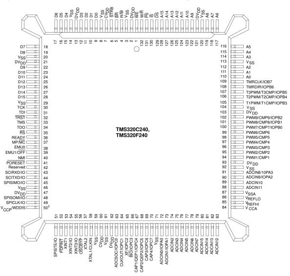
Figure 11-2. TMS320C240 and TMS320F240 Pin Out Assignment
