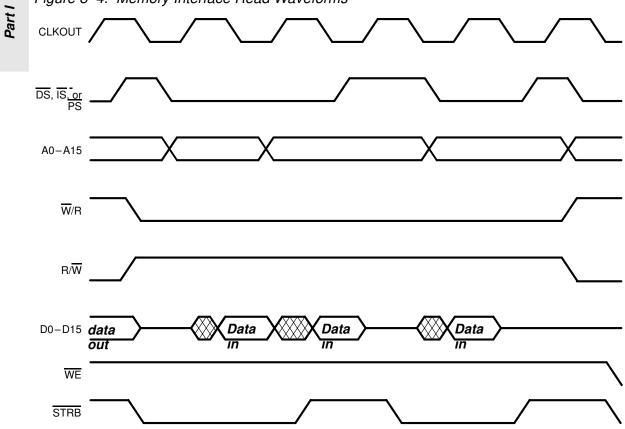
Figure 8-4. Memory Interface Read Waveforms
