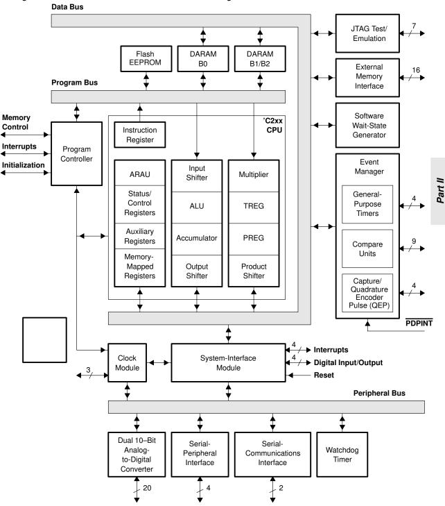
Figure 11–3. TMS320x240 Functional Block Diagram
