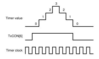
Figure 2–6. GP Timer Single Up/down Counting Mode (TxPR = 3)
