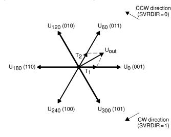
Figure 2–24. Basic Space Vectors and Switching Patterns
