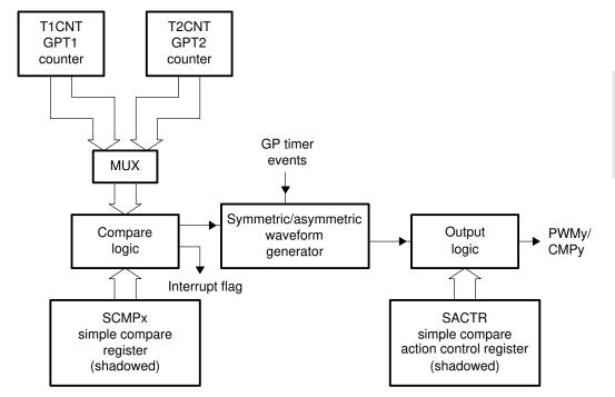
Figure 2–12. Simple Compare Unit Block Diagram (x = 1, 2, or 3; y = 7, 8, or 9)
