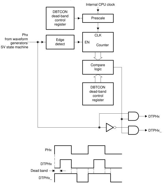
Figure 2–19. Dead-Band Unit Block Diagram (x = 1, 2, or 3)
