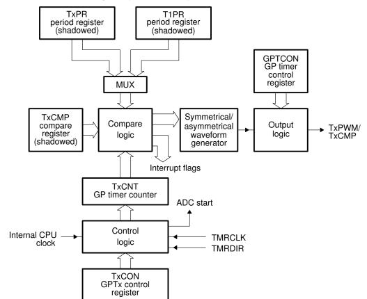
Figure 2–2. GP Timer Block Diagram (x = 1, 2, or 3)
