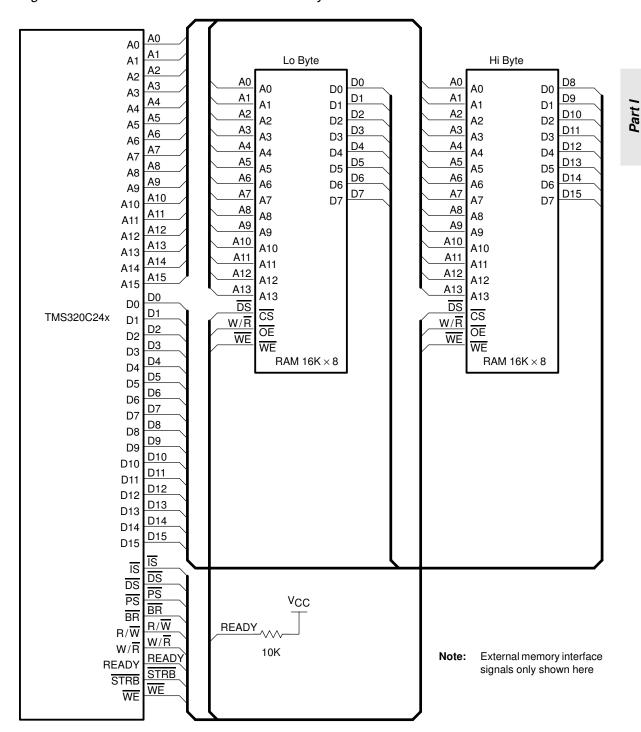
Figure 8-2. Interface to External Data Memory
